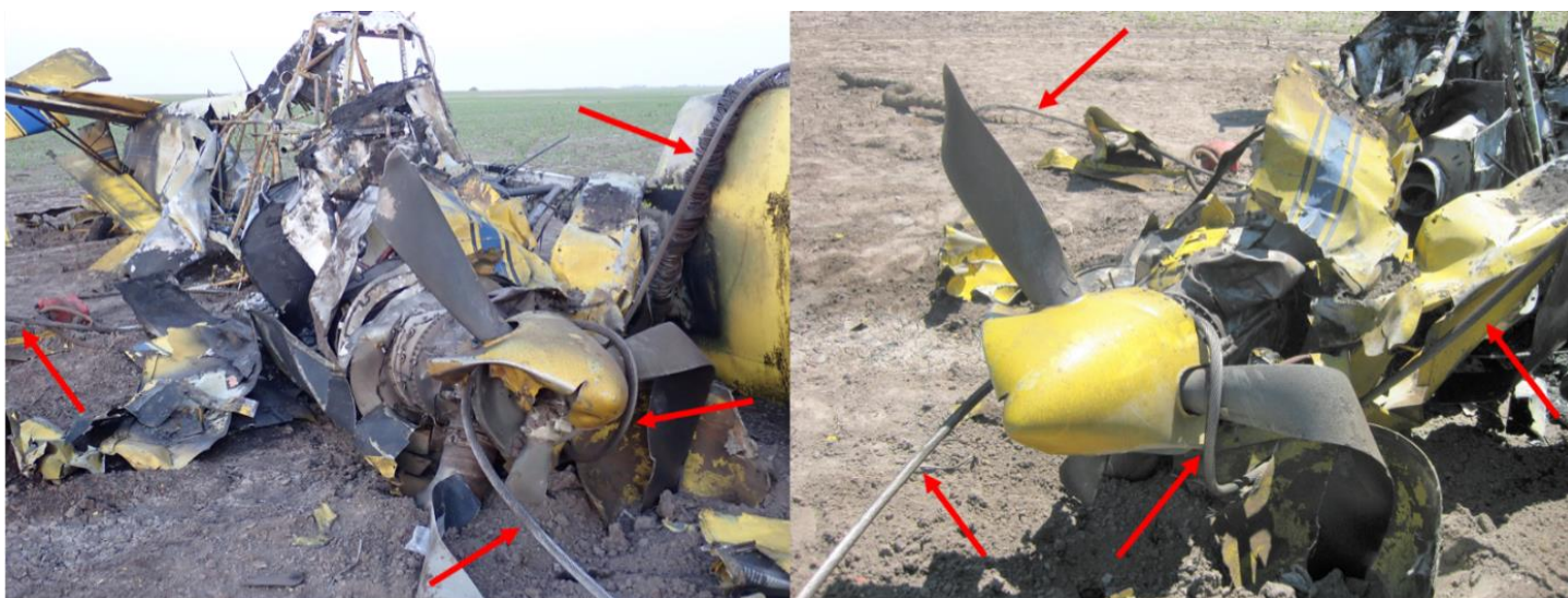
Figure 2 - Power Transmission Cables Conjoined with Main Wreckage (red arrows point to cables)
