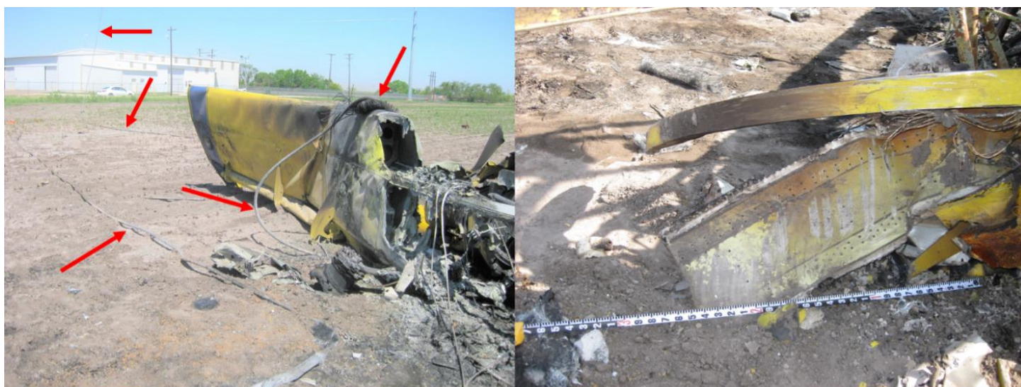
Figure 3 - Power Transmission Cables Conjoined with Right Wing (Left Image) and Cable Impact Marks to the Forward Face of the Left Main Wing Spar (Right Image)
