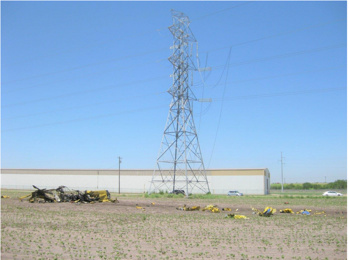
Figure 1. Main Wreckage and Impact Debris Path
