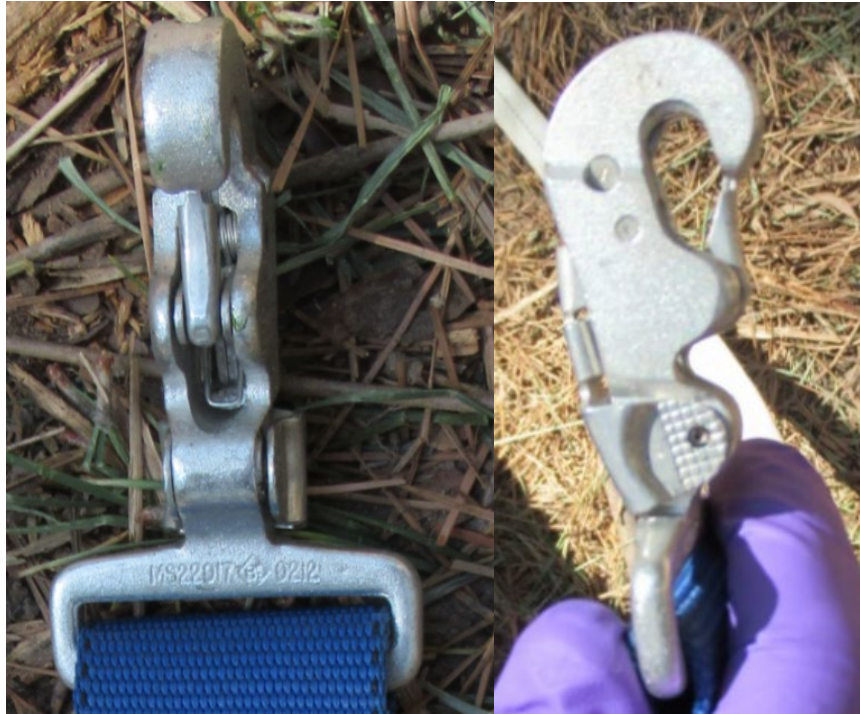
Photograph 9 – Hook of Rear Supplemental Passenger Restraint System
