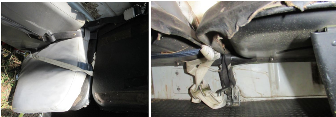
Photograph 12 - Tether Routed Between Double Bench Seats and Secured to the Cabin Floor
