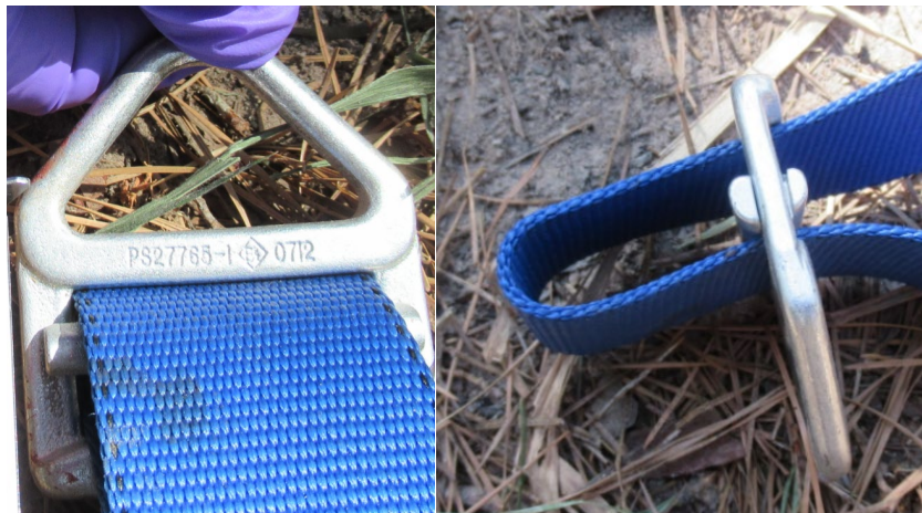
Photograph 10 – Adjuster of Rear Supplemental Passenger Restraint System
