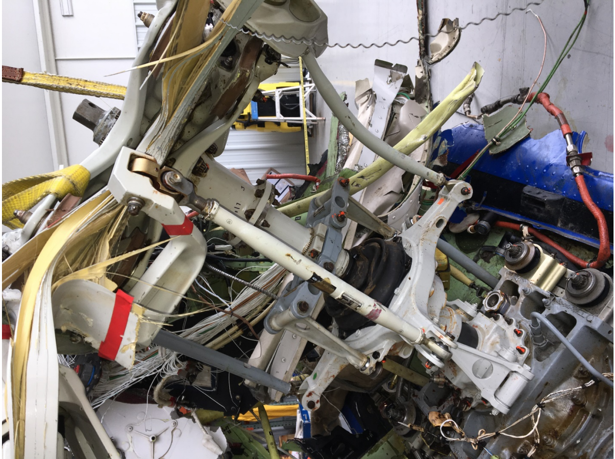
Photo 2: Main Rotor Mast
