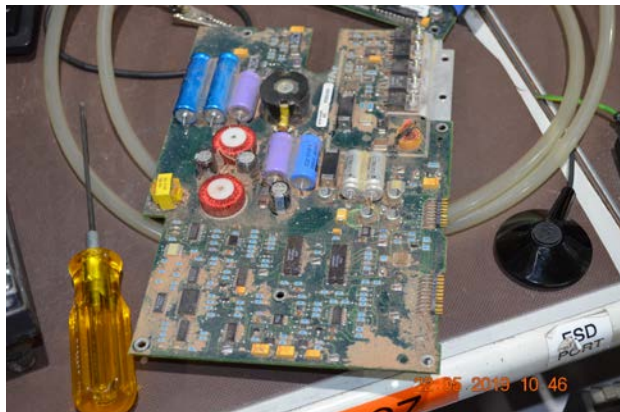
KC 225 Flight Computer – dried dirt/mud/sand present
