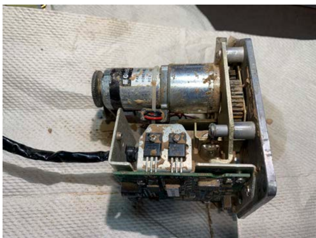
Dried dirt/mud present on servo electrical and mechanical assemblies
