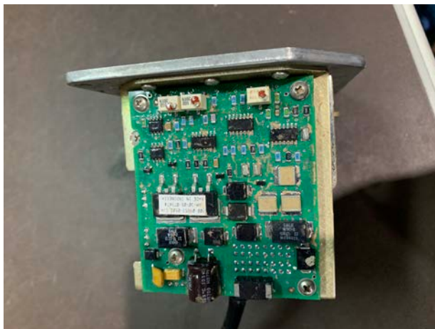
Dried dirt/mud present on electrical and mechanical assemblies
