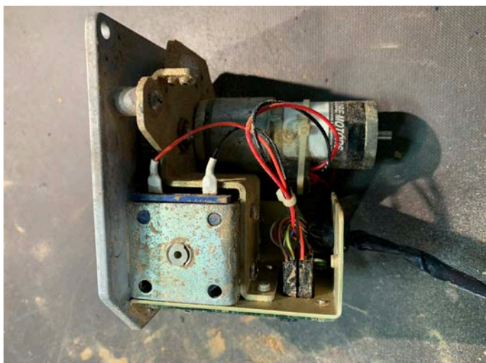
KS 271C Yaw Servo – dried dirt/mud/sand present
