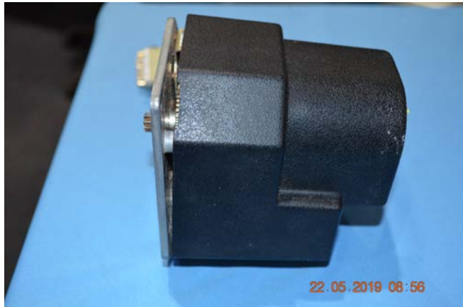
Cover attach bracket bent causing poor cover fitment
