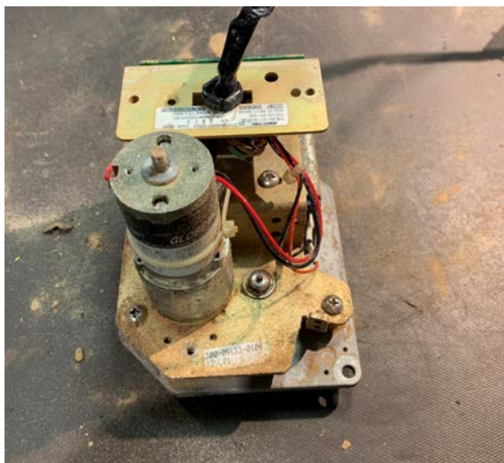
KS 271C Yaw Servo – dried dirt/mud/sand present
