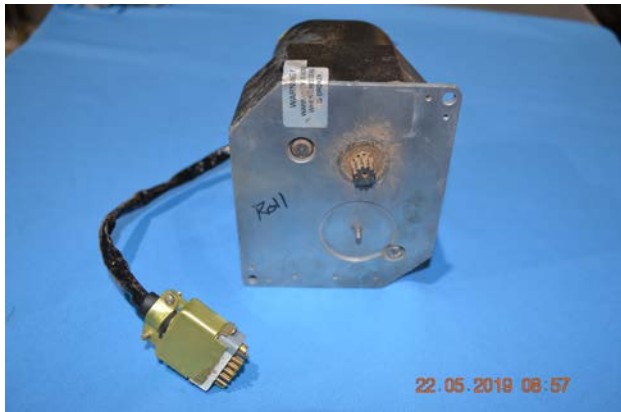
Dried dirt/mud on pinion gear and bearing
