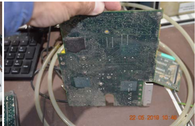
KC 225 Flight Computer – dried dirt/mud/sand present
