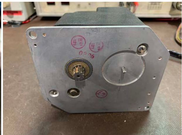
Dried dirt/mud present on electrical and mechanical assemblies
