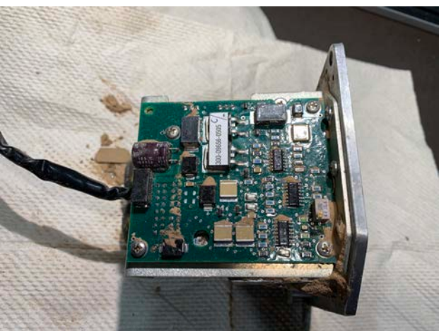
Dried dirt/mud present on servo electrical and mechanical assemblies
