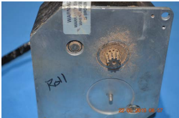
Dried dirt/mud on pinion gear and bearing
