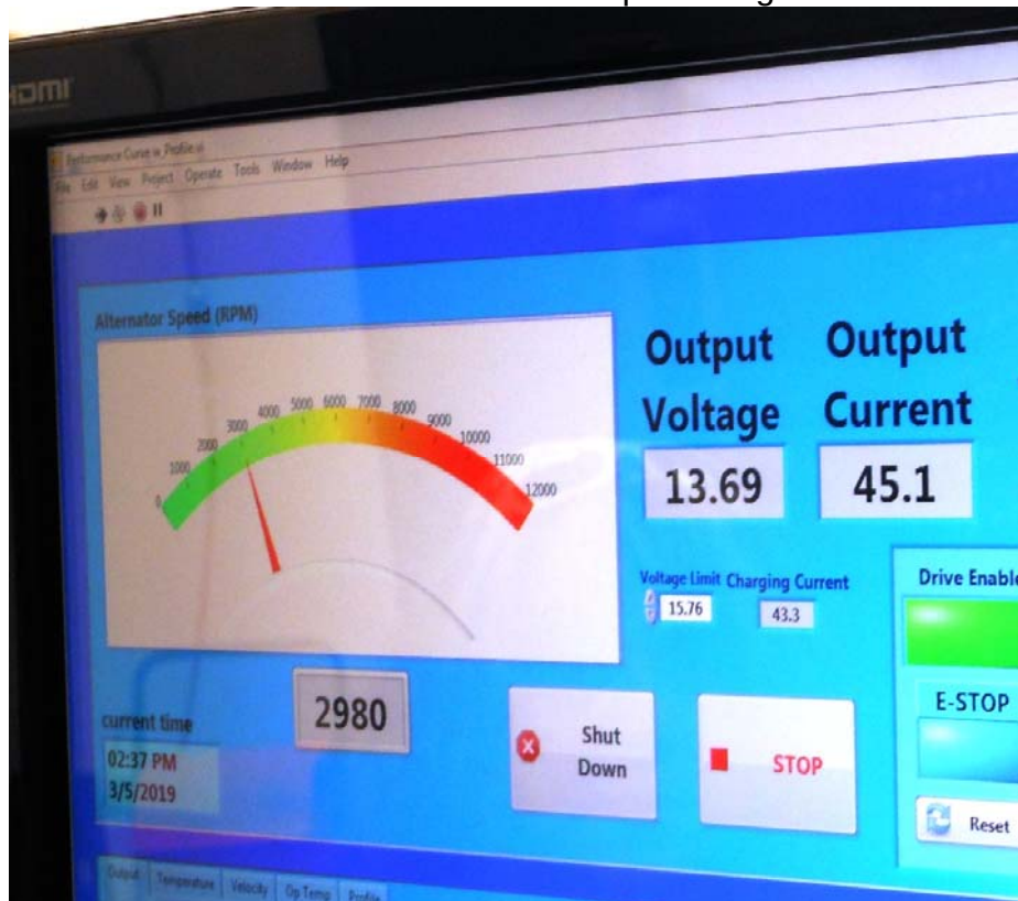
Photo #16 – Alternator Controller output voltage and current
