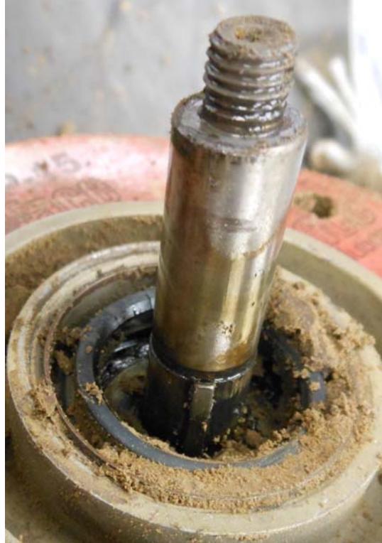
Photo #5 – Alternator drive shaft and Woodruff key
