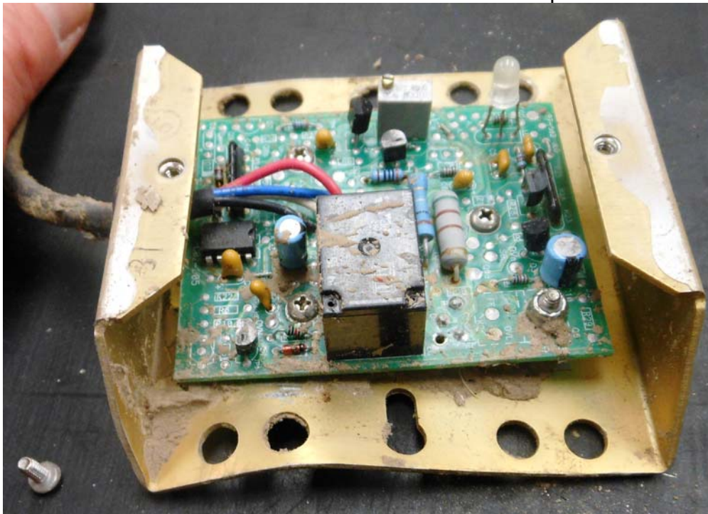
Photo #15 – Alternator Controller internal components
