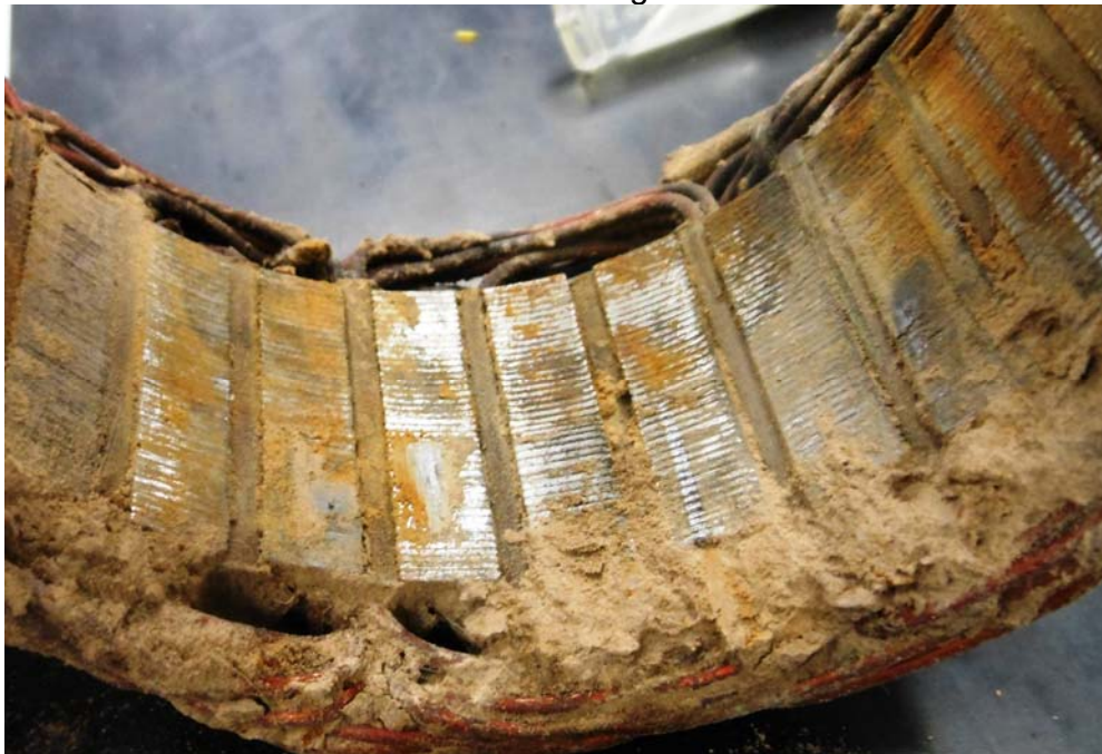
Photo #11 – Stator/armature damage from contact with rotor
