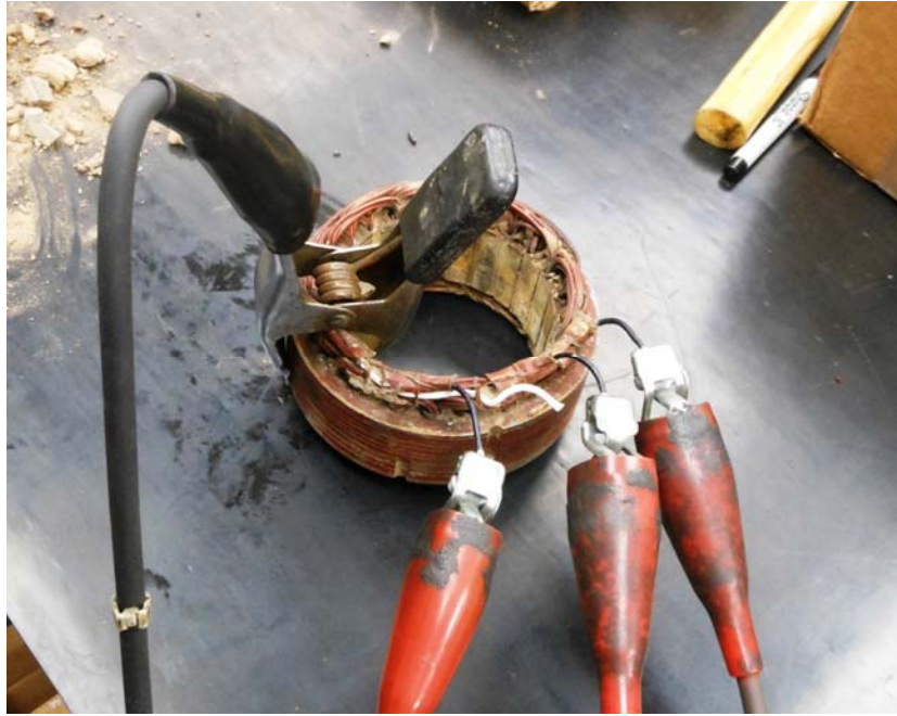
Photo #13 – Stator/armature coil test
