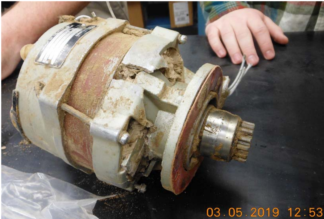
Photo #1 – Alternator as-received
