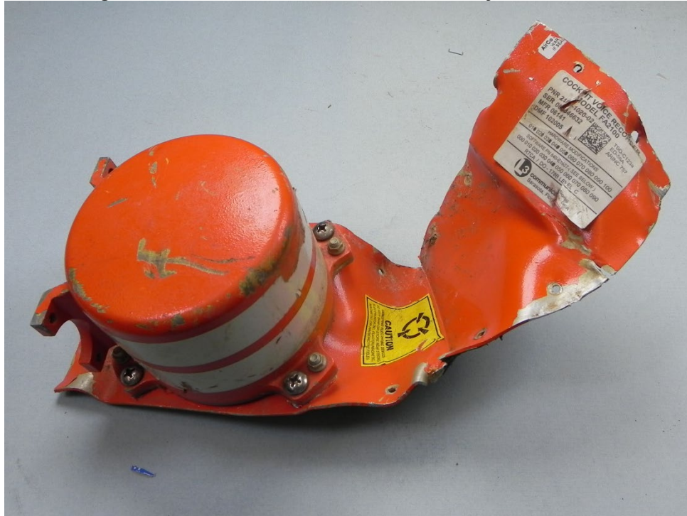
Figure 1. Exterior of crash-survivable memory, as received.
