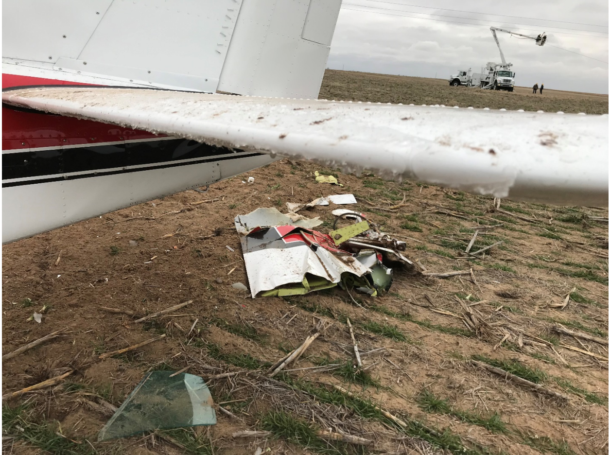
Photo 2: Ice on the Horizontal Stabilizer
