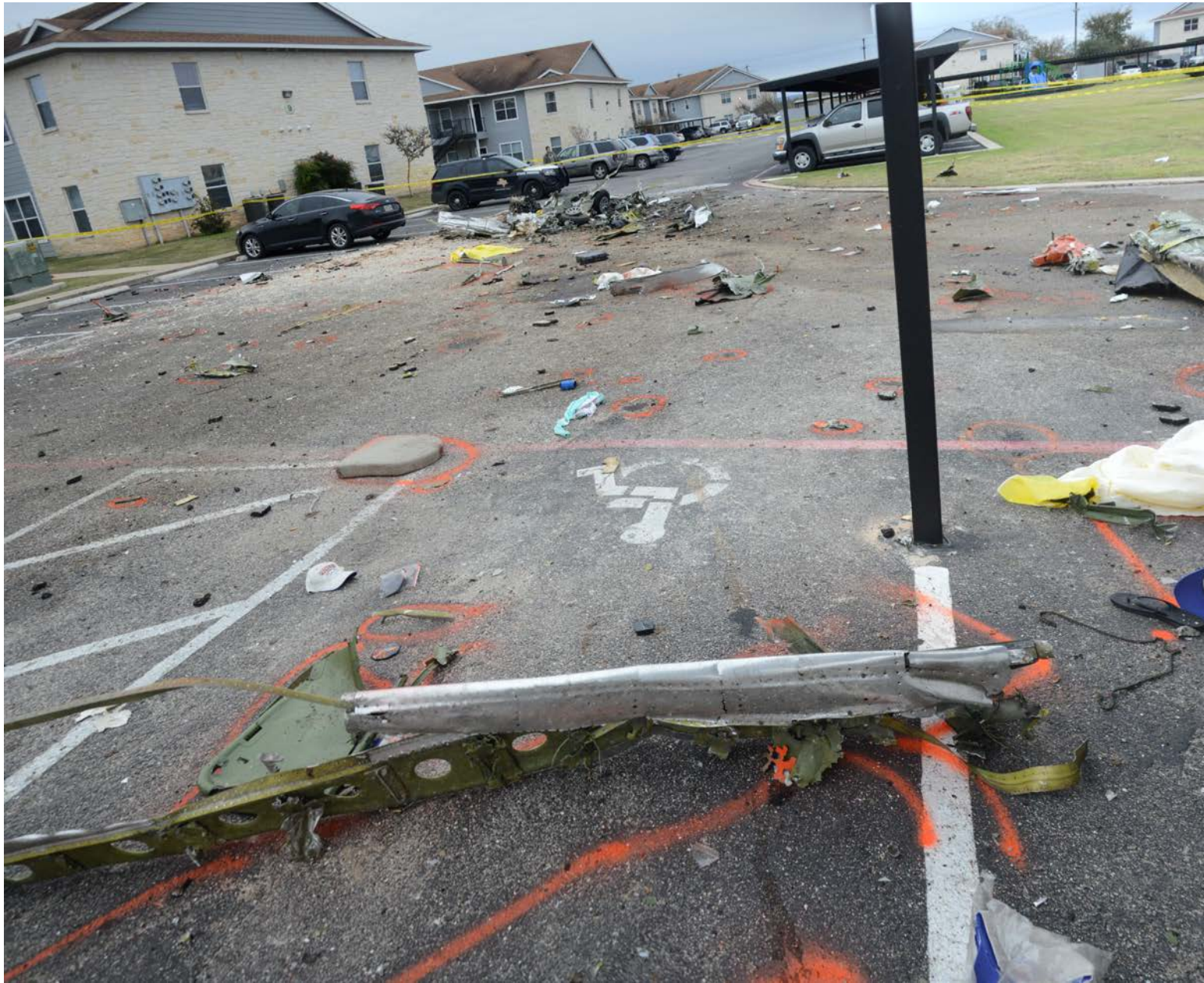
Photo 11 - View of a separated section of a wing spar with the embedded engine in the background.
