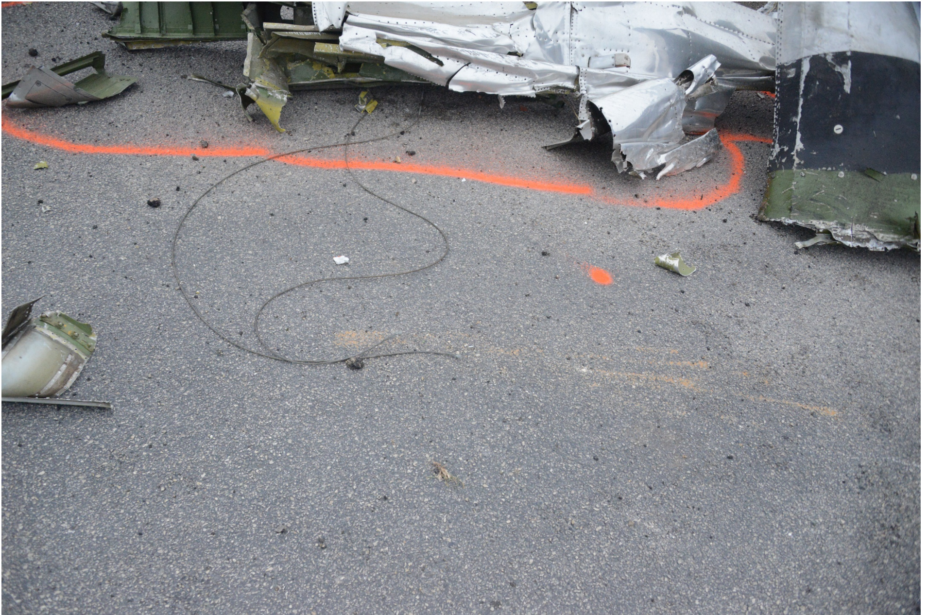
Photo 14 - View of the separated flight control cables.
