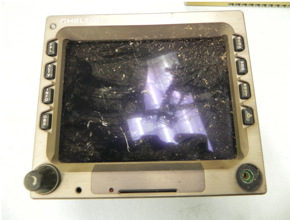
Figure 1. Photo of damaged device #1 (S/N 40557)
