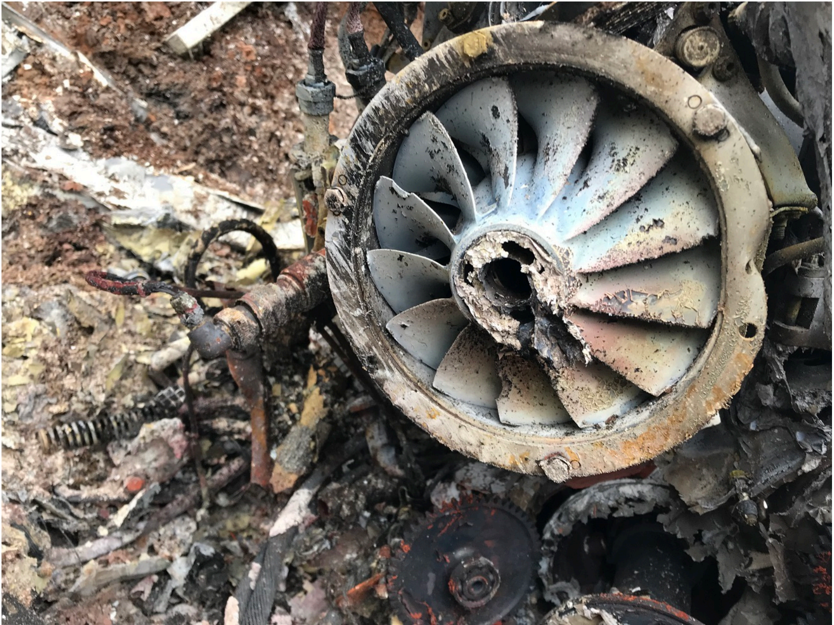
Photo 5 - Engine inlet compressor
