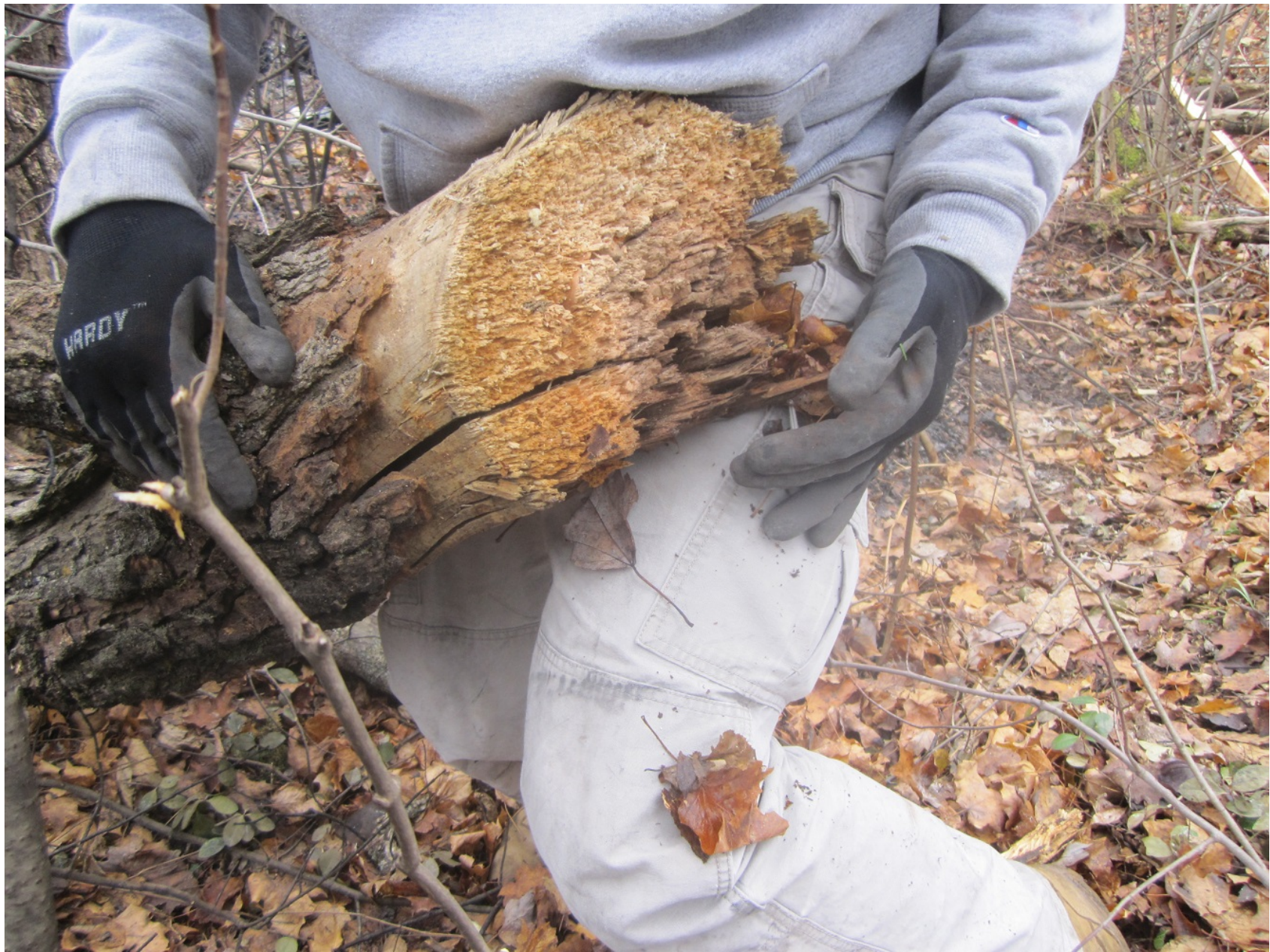
Photo 9 – Cut tree – likely from the main rotor blade
