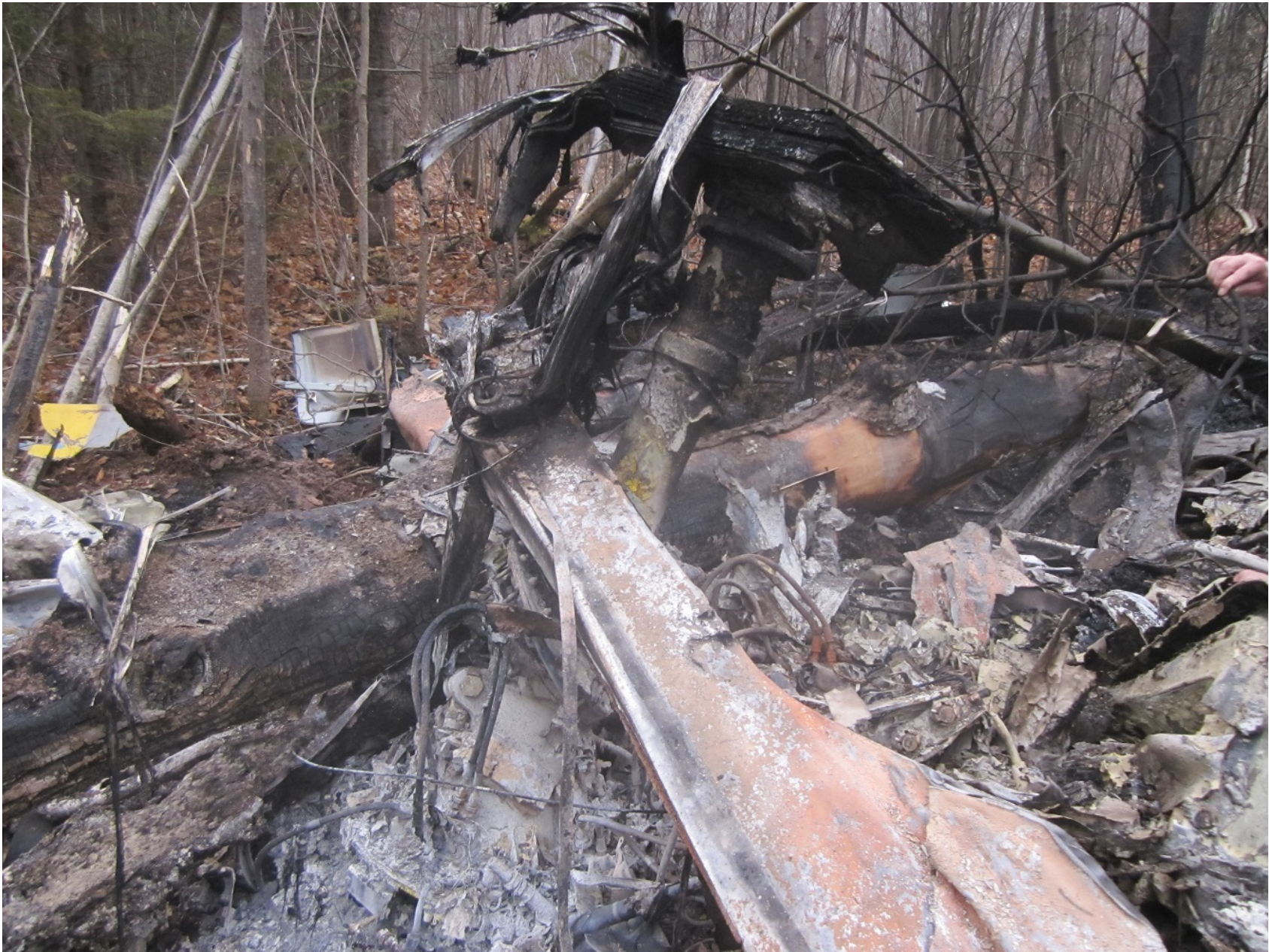
Photo 7 – Main Wreckage – Rotor mast
