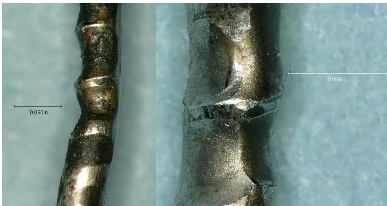
Figure 5: Close-up of scalloped wear pattern on control cable end (right image taken after cleaning).
