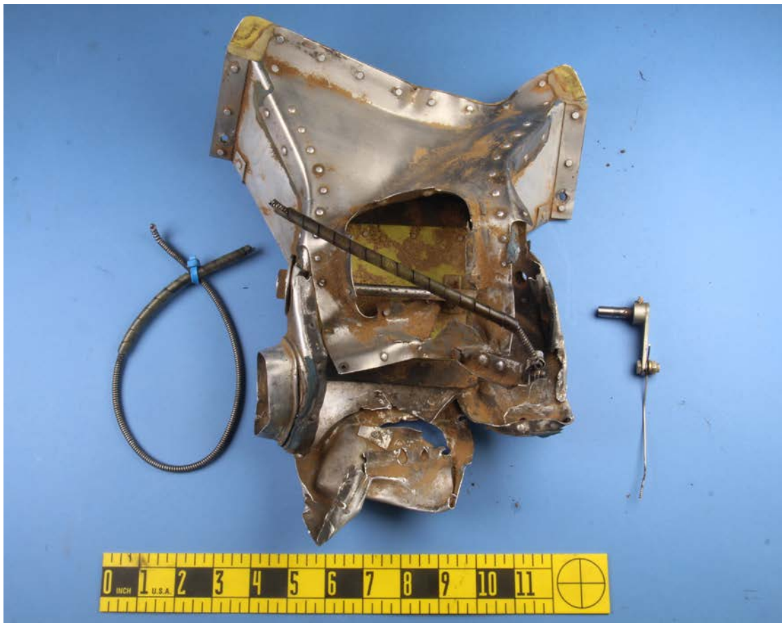
Figure 1: Carburetor heat box, portion of heat valve shaft and cable sheathing as received.
