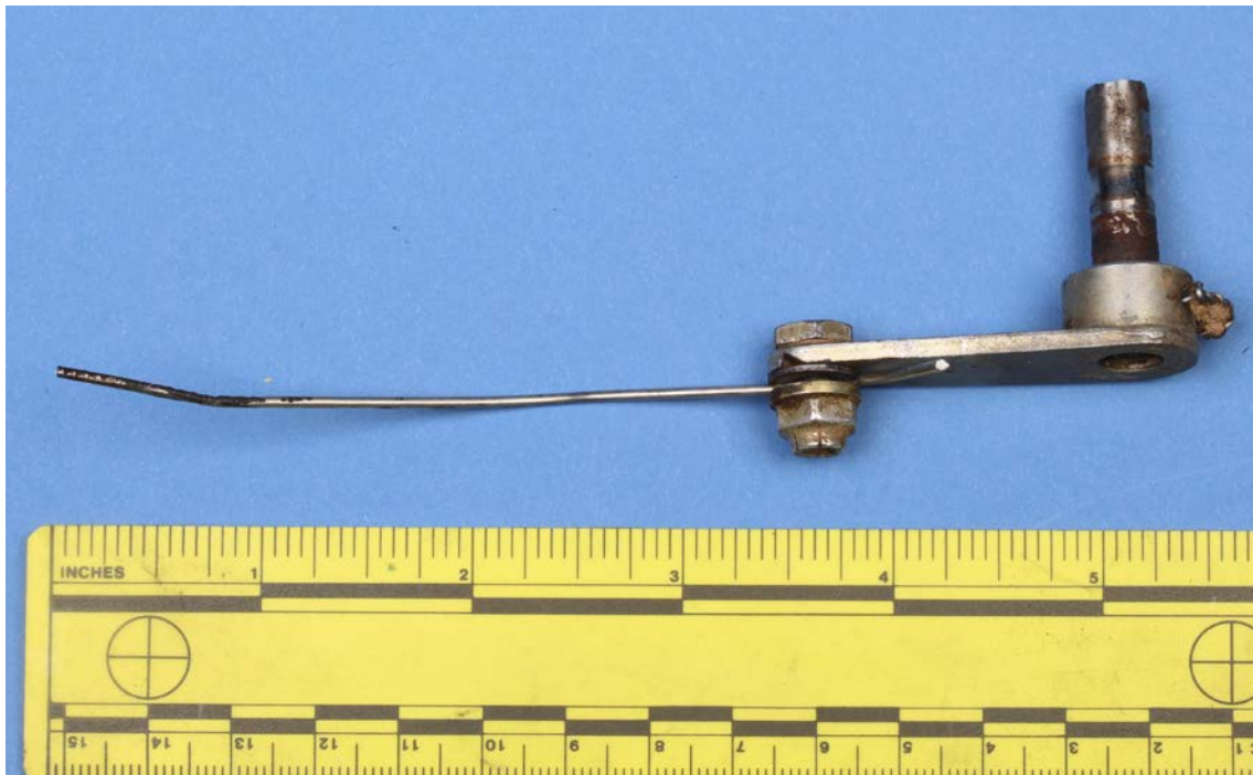
Figure 2: Portion of heat valve shaft, control arm and portion of control cable.
