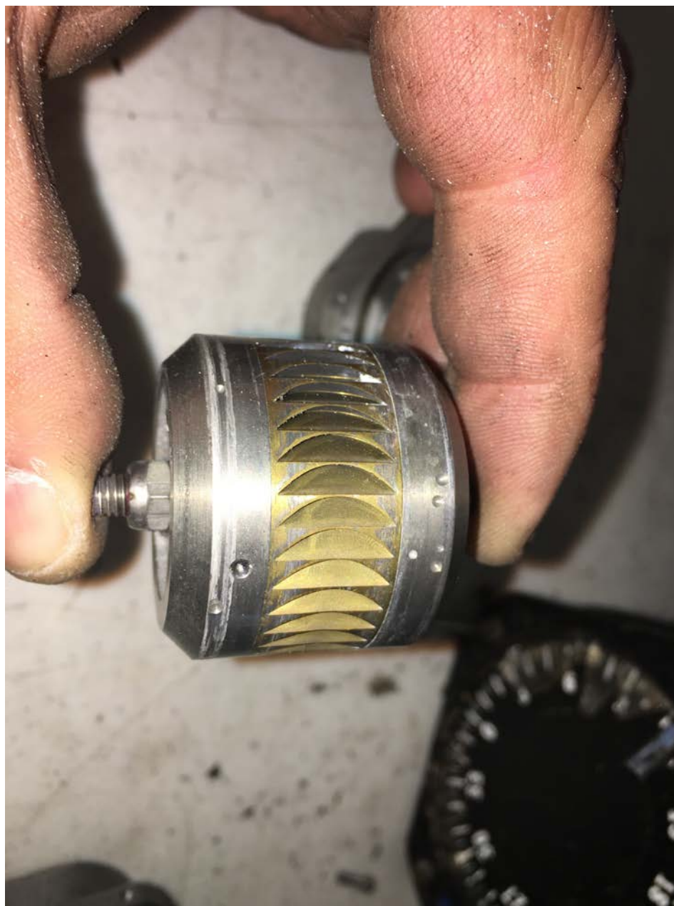
Photo 7 – Gyroscope core showing rotational scoring
