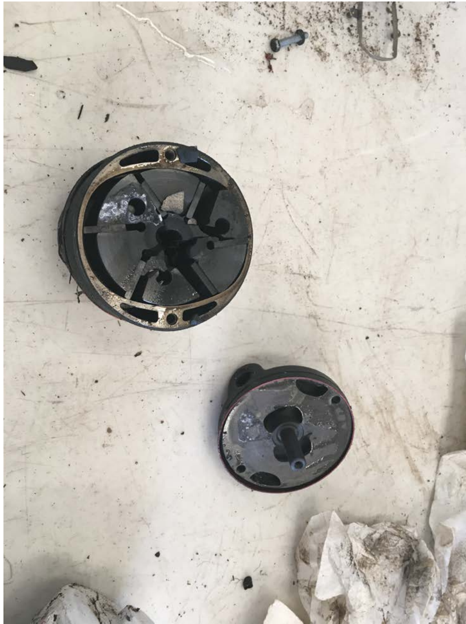
Photo 5 – Vacuum pump during layout examination
