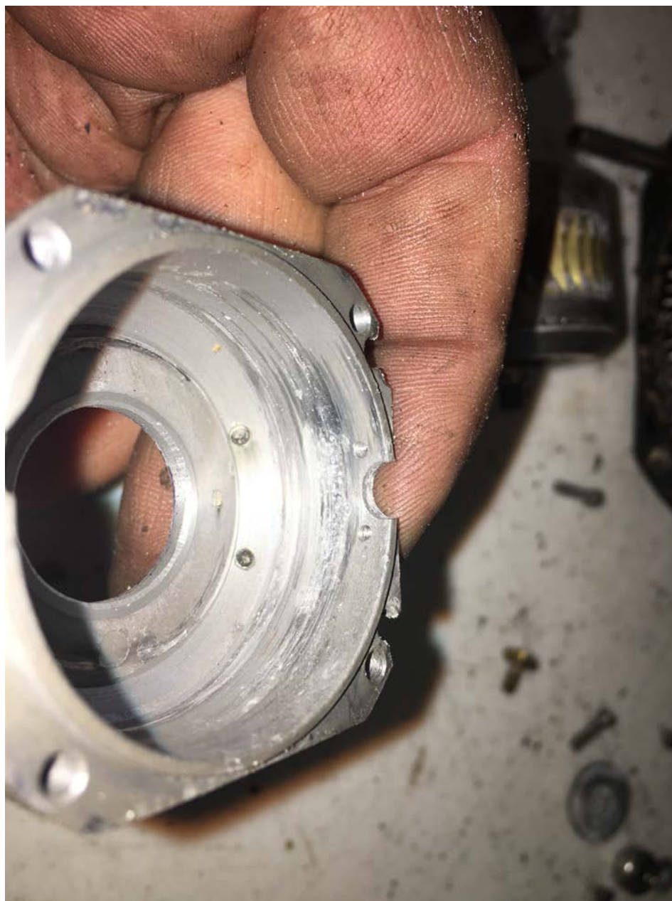
Photo 6 – Gyroscope housing showing rotational scoring
