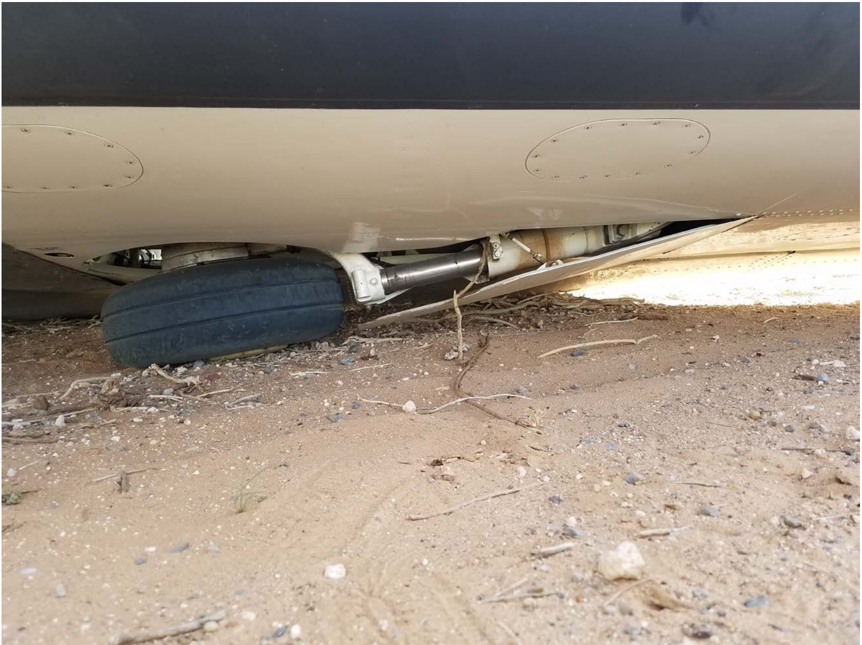
Photo 2 – Collapsed Landing Gear
