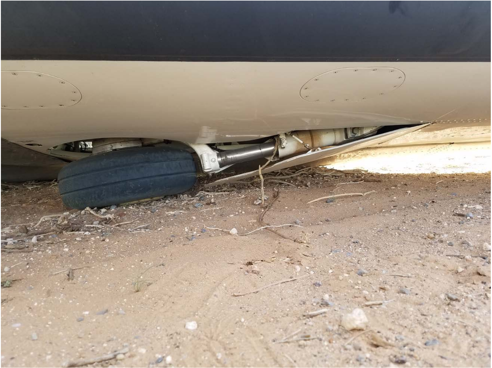
Photo 2 – Collapsed Landing Gear
