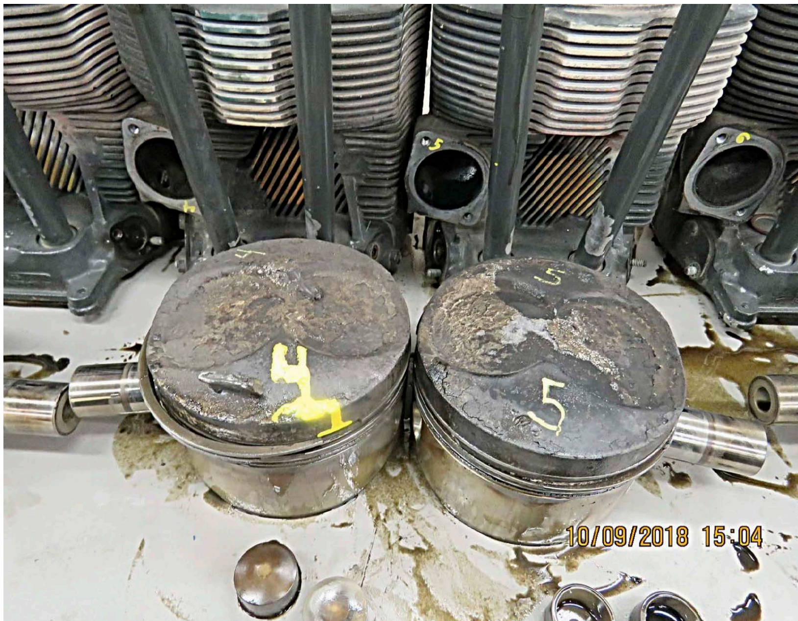
Photo 9 – Damage to pistons 4 and 5. Note embedded valve fragments.
