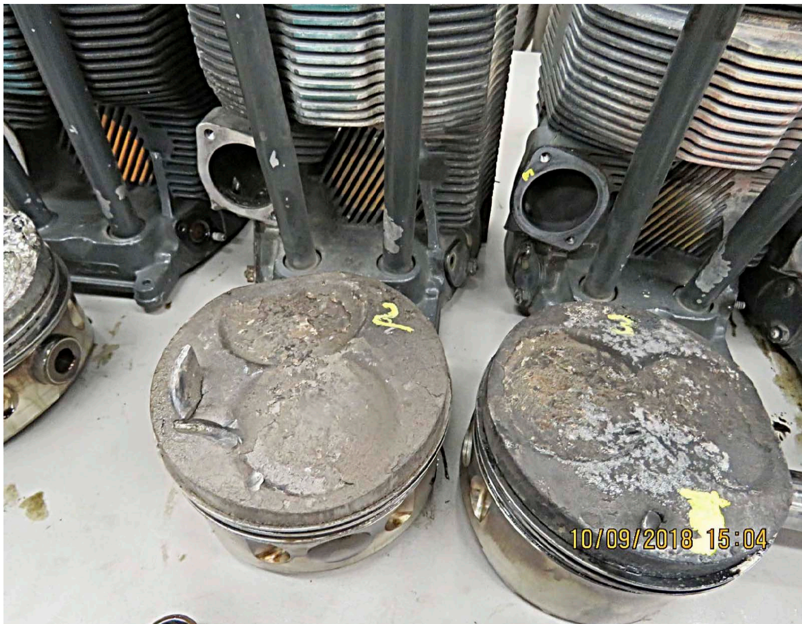
Photo 8 – Damage to pistons 2 and 3. Note embedded valve fragments.
