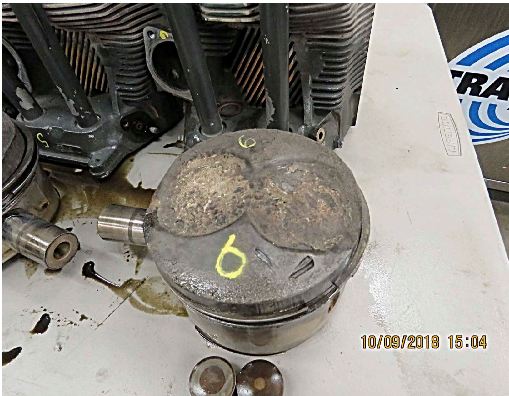
Photo 10 – Damage to piston 6. Note embedded valve fragment.
