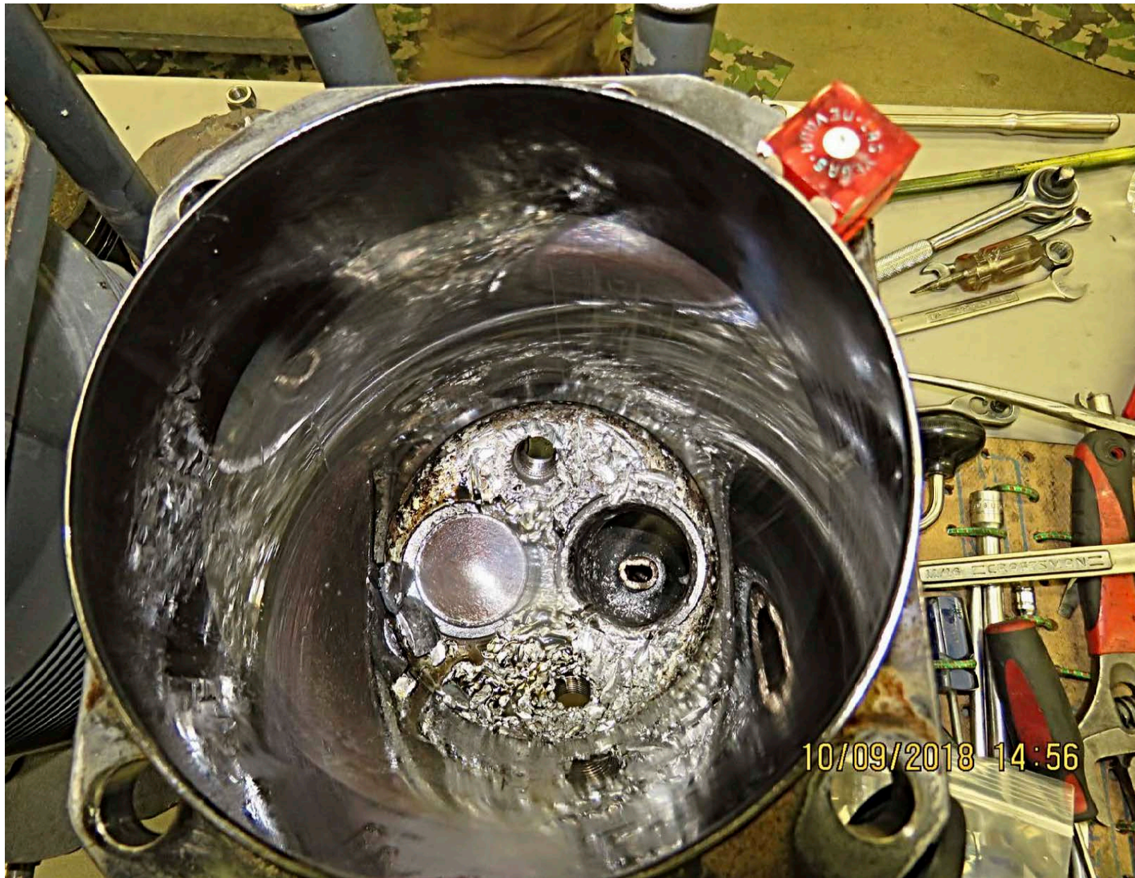
Photo 6 – Damage to cylinder 1.
