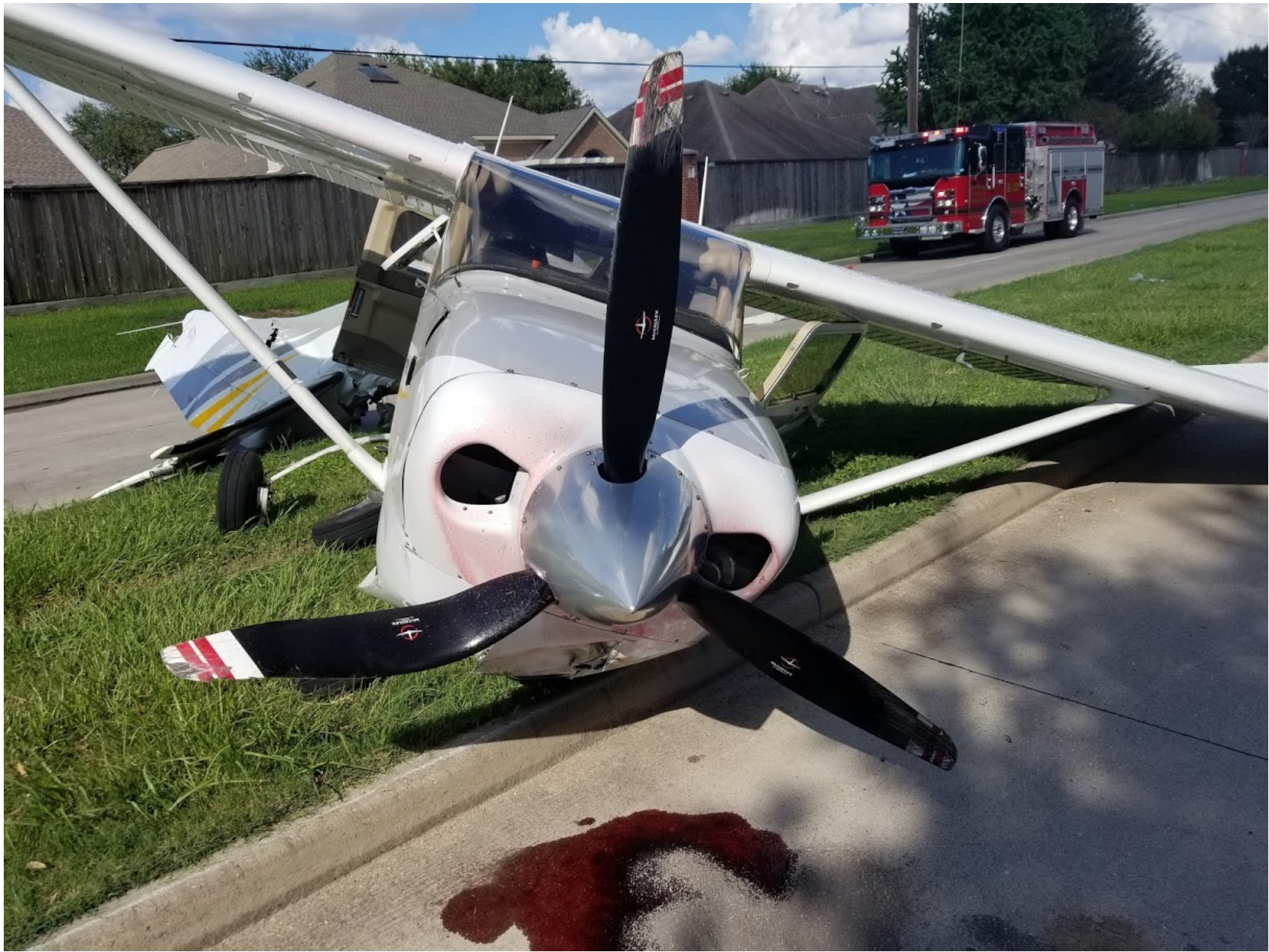
Photo 4 – The nose of the airplane and spilled hydraulic fluid.
