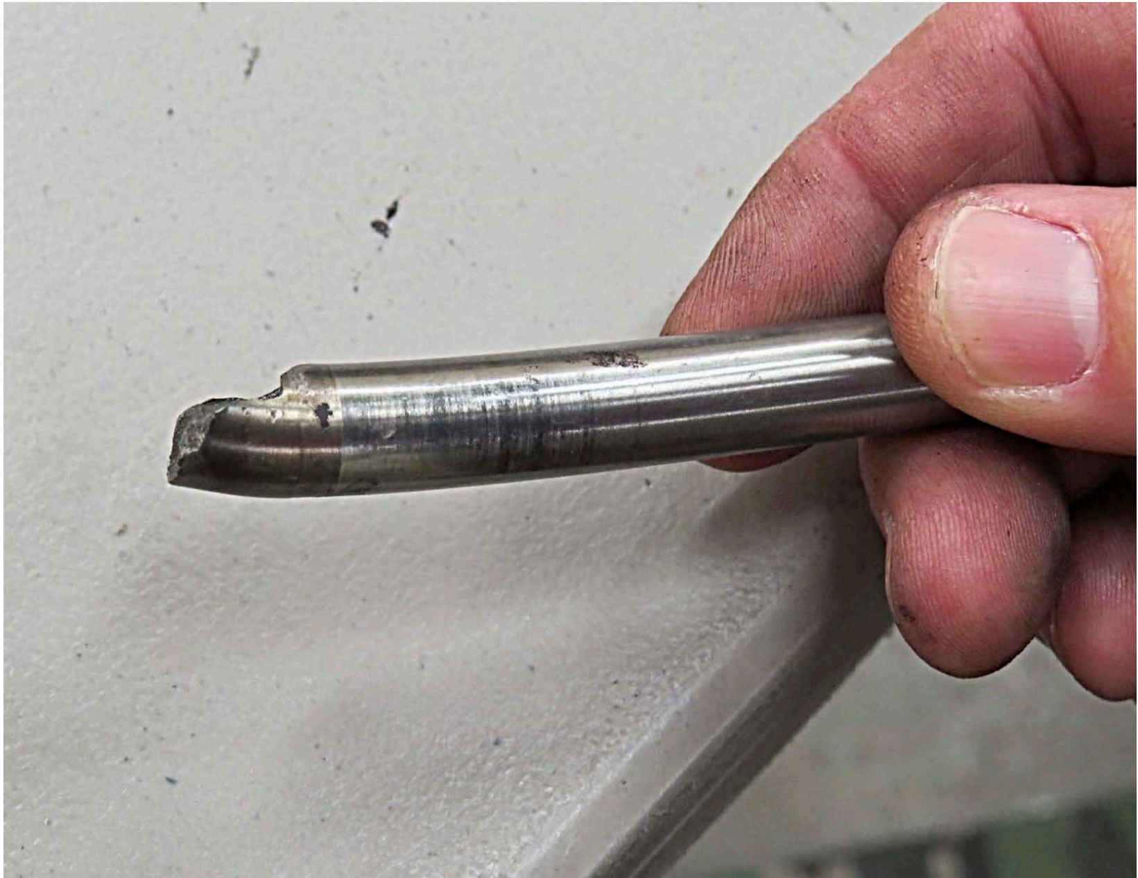
Photo 11 – Bent no. 1 valve stem tip caused by piston and combustion chamber contact, and most probably contributed to no. 1 intake valve failure.
