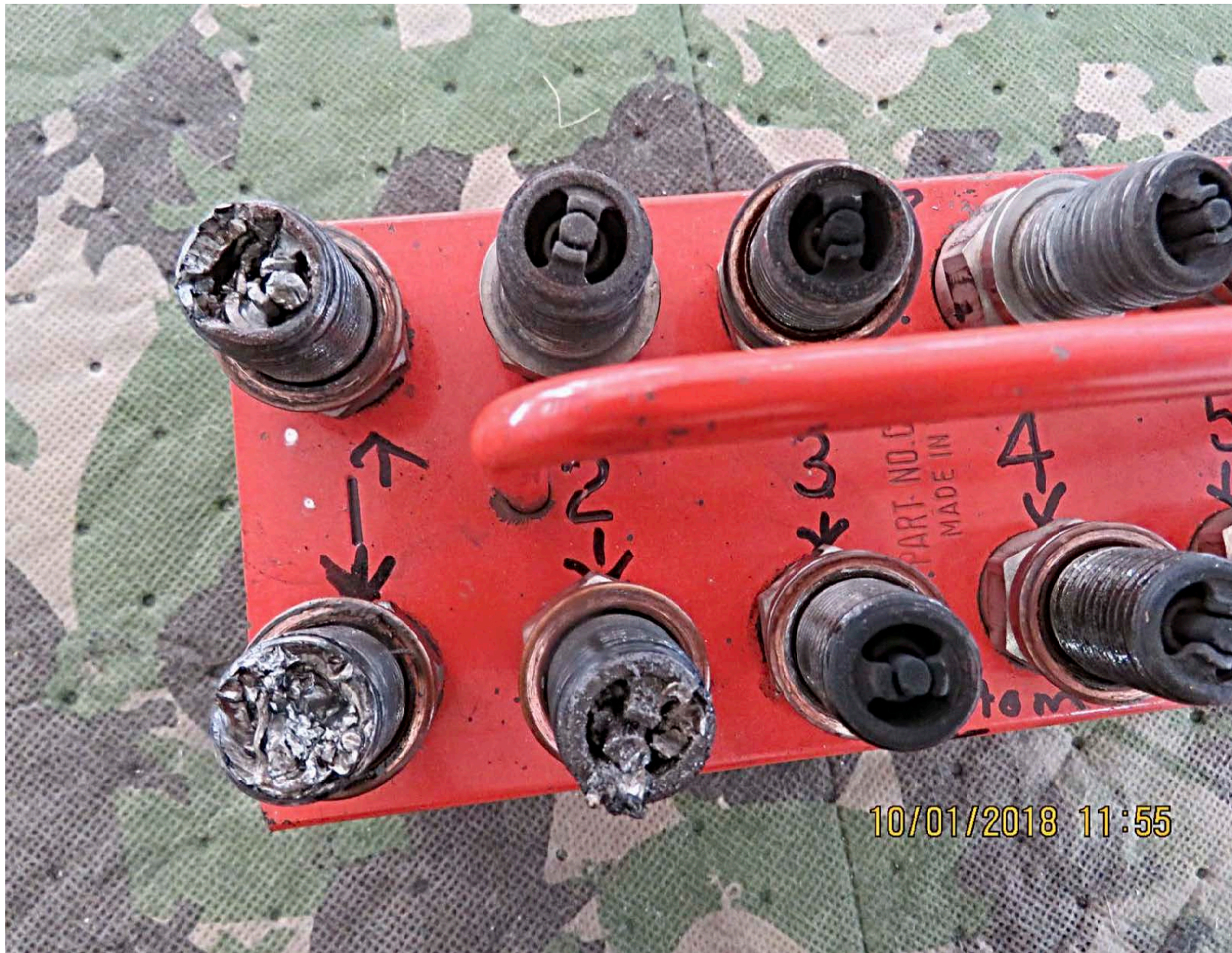
Photo 5 – The spark plugs after removal from the engine. Note the damage to plugs 1 and 2.
