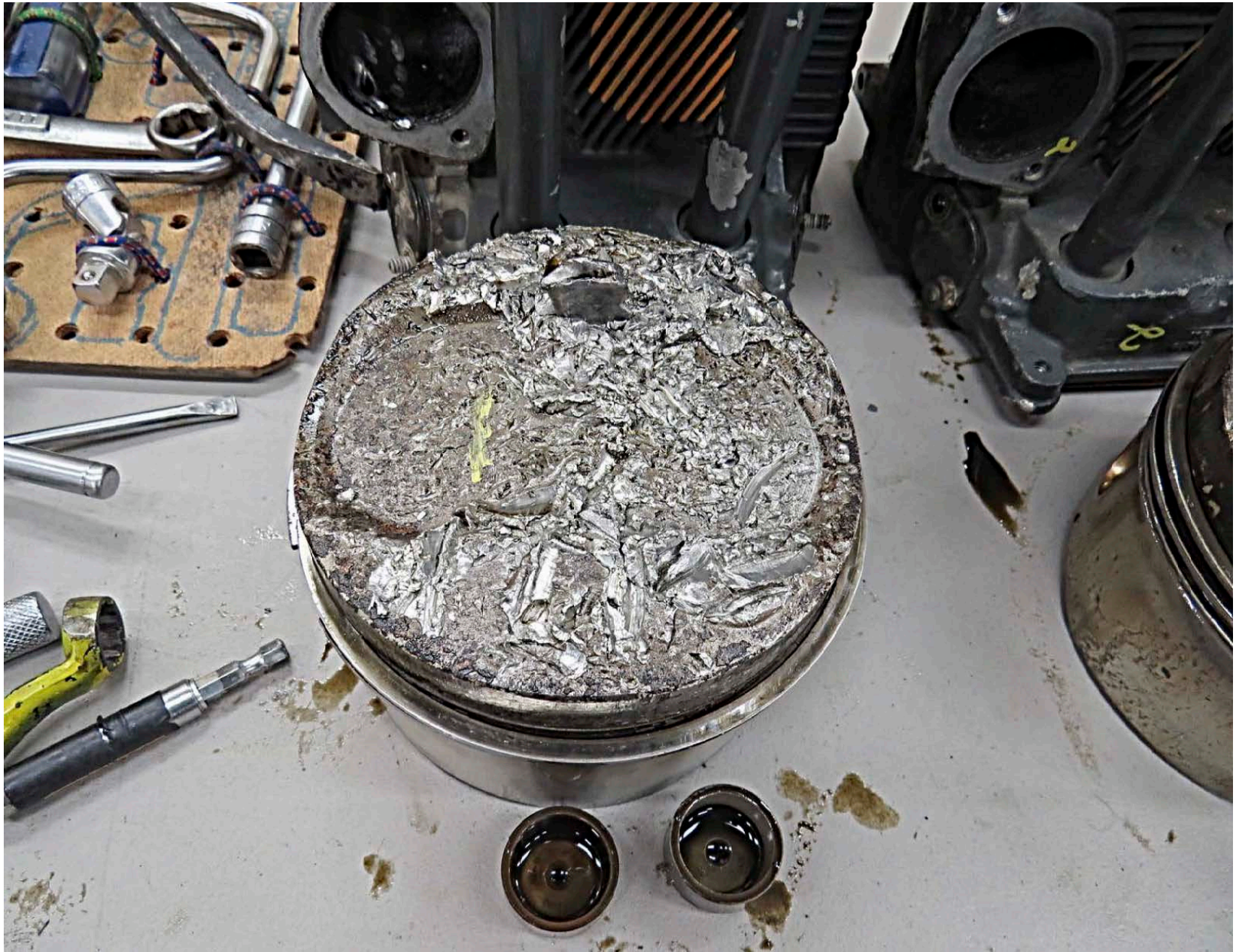
Photo 7 – Damage to piston 1. Note embedded valve fragment.
