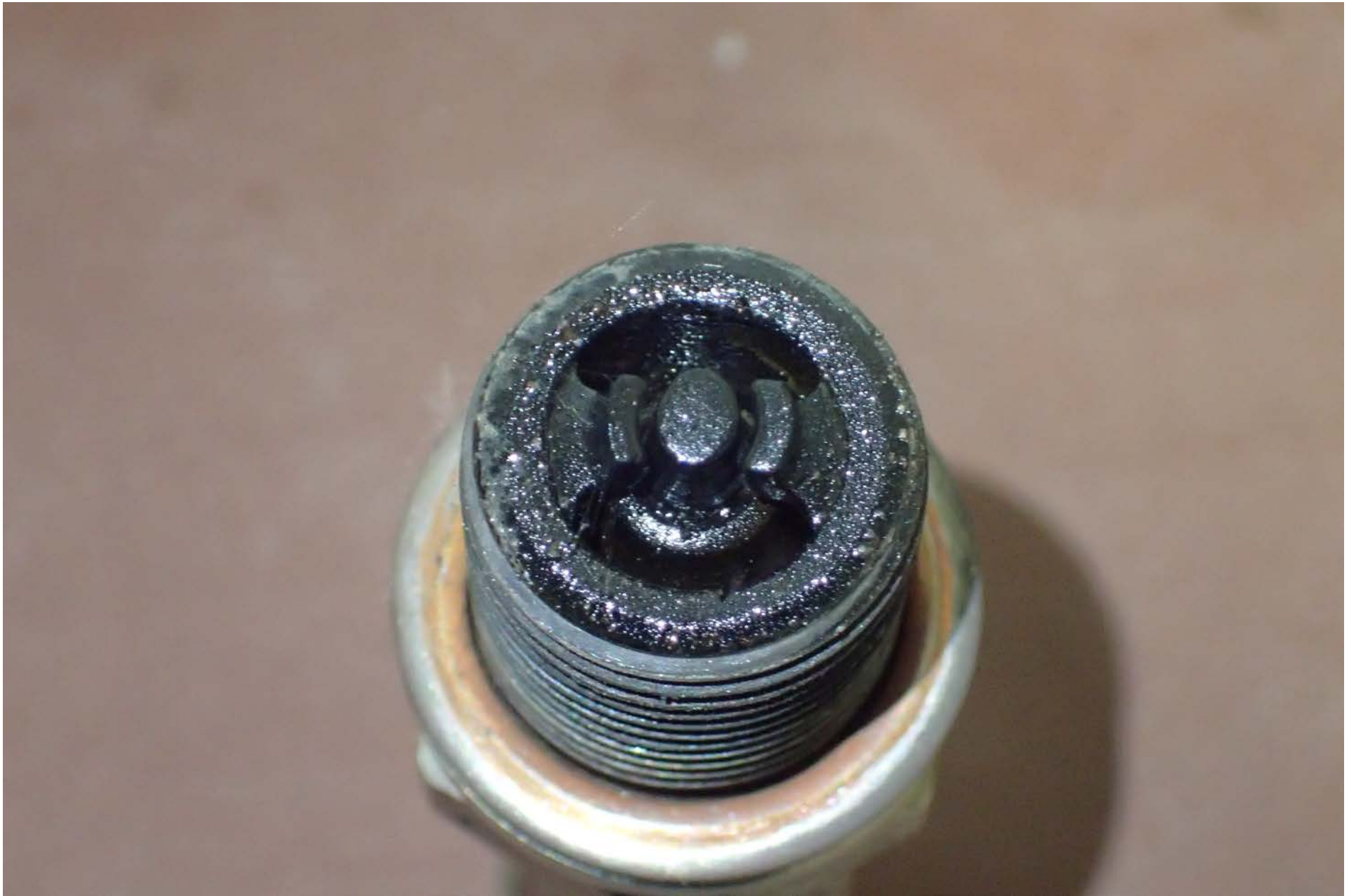
Photo 8 - View of carbon build-up on 2B sparkplug (CM Photo)
