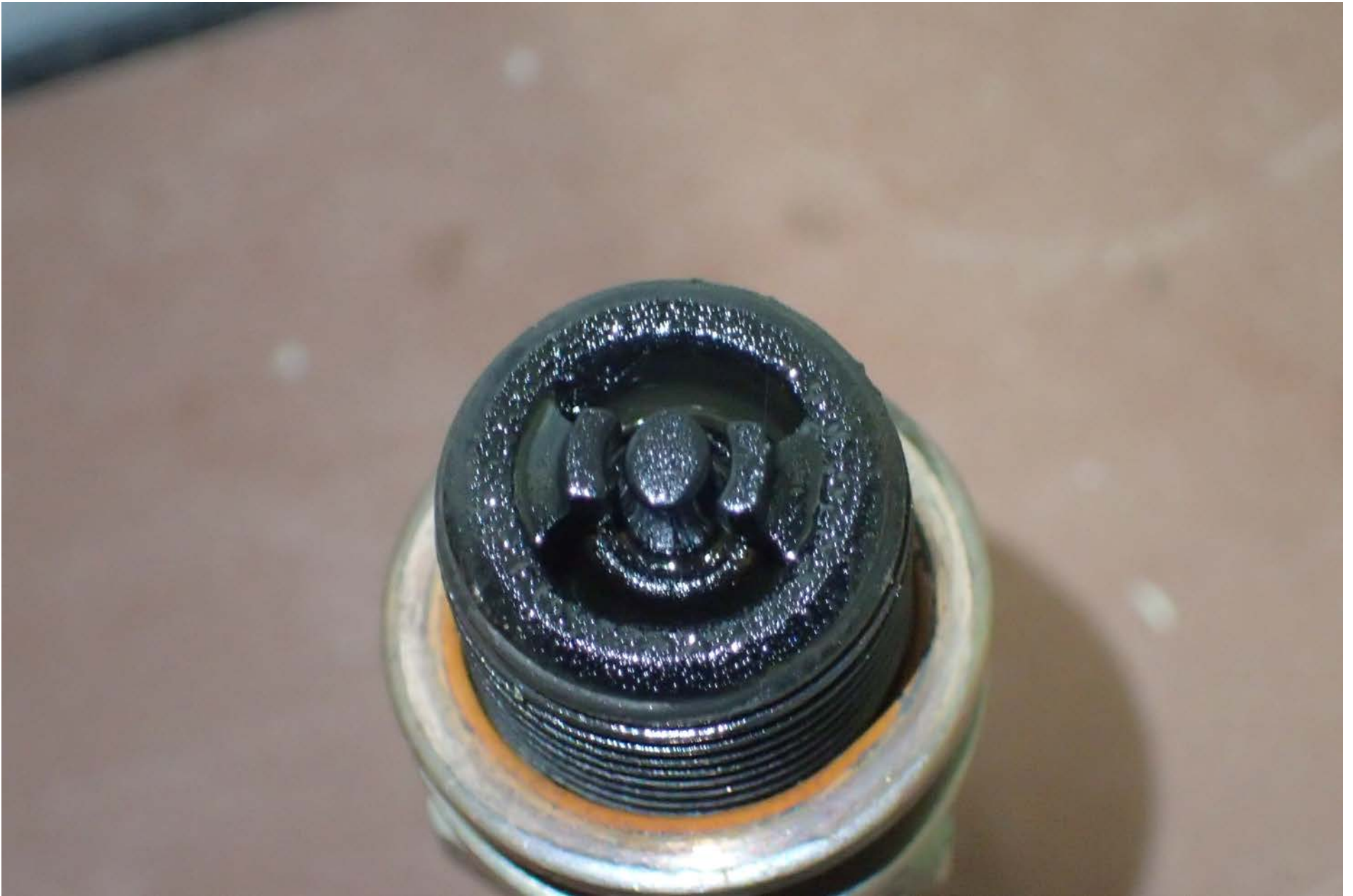
Photo 9 - View of carbon build-up on 4B sparkplug (CM Photo)
