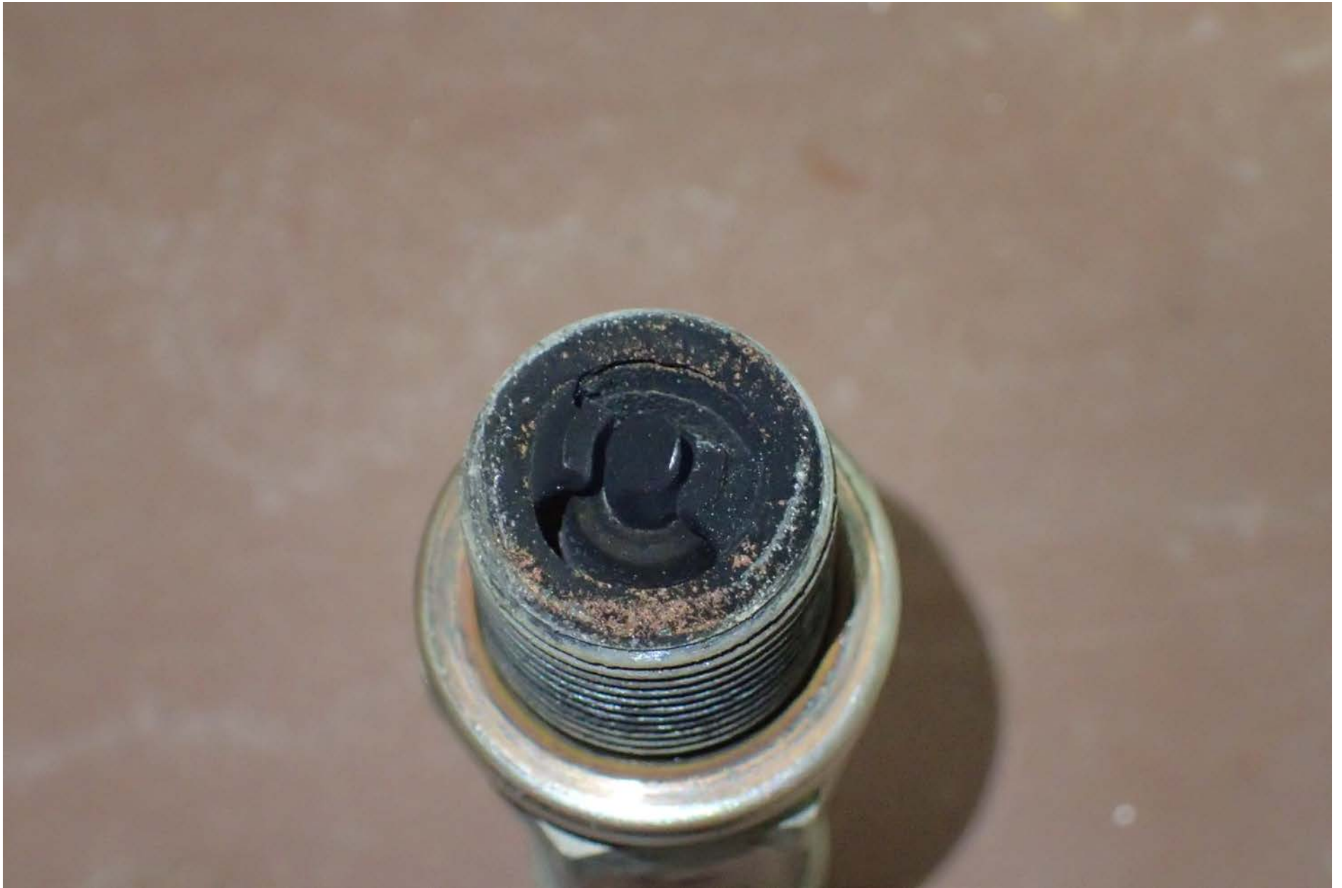
Photo 7 - View of carbon build-up on 5B sparkplug (CM Photo)
