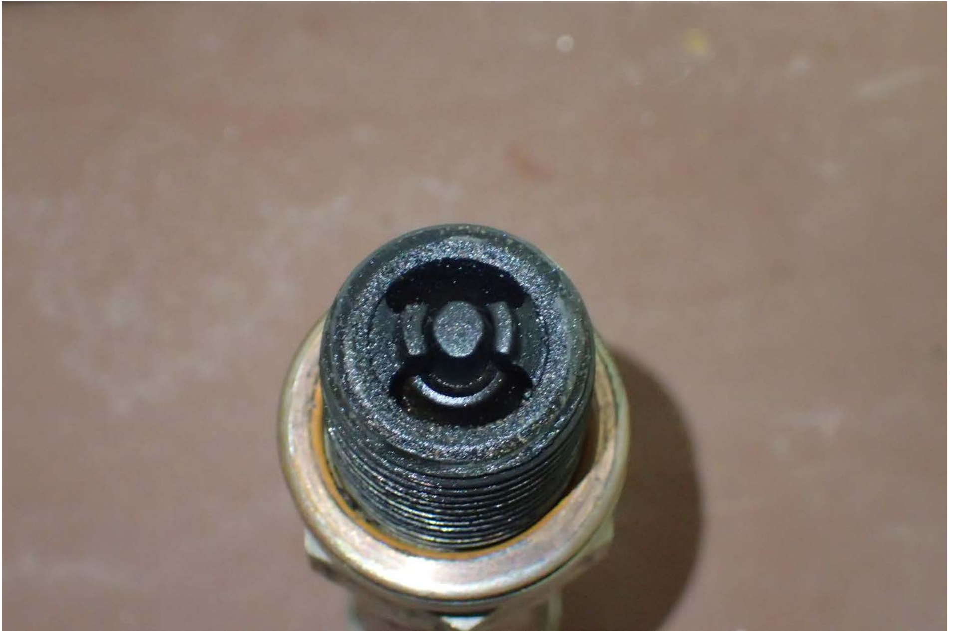
Photo 6 – View of carbon build-up on 3B sparkplug (CM Photo)
