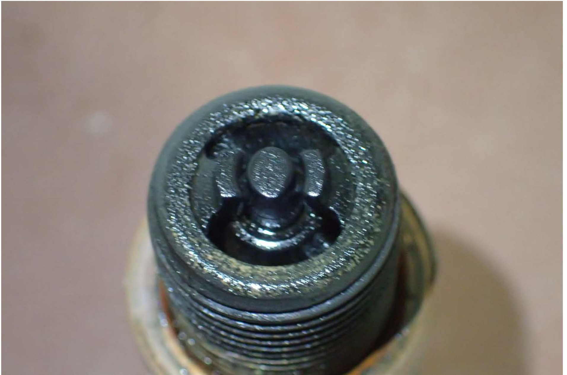
Photo 10 - View of carbon build-up on 6B sparkplug (CM Photo)
