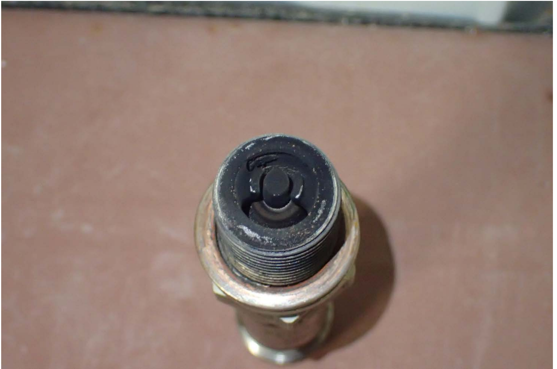
Photo 5 – View of carbon build-up on 1B sparkplug (CM Photo)
