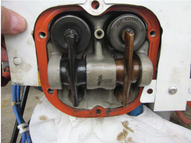
#1 cylinder valve cover removed
