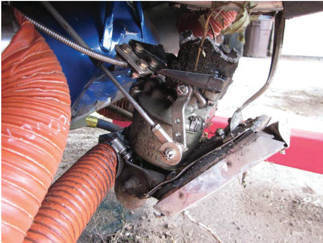
Fuel manifold broke from apparent ground impact.
