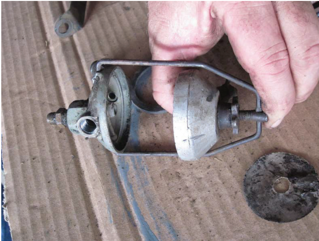
Reassembled gascolator, the wire clip, tightening nut, gasket, broken glass bowl and filter screen was found in the lower cowling on removal. The filter screen seen in the lower right is packed with dirt from the ground impact.
