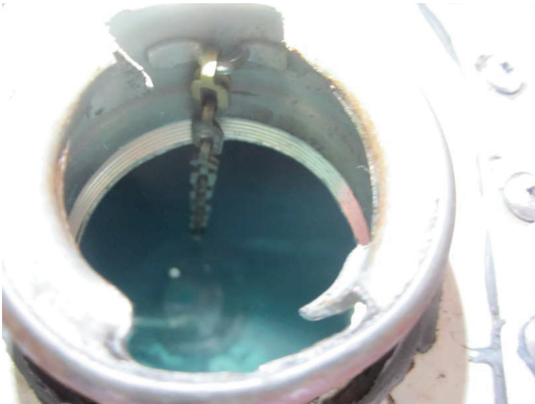
Fuel in right tank prior to draining, light blue tint indicates 100LL in the tank, removed approximately 5 gallons of fuel.
