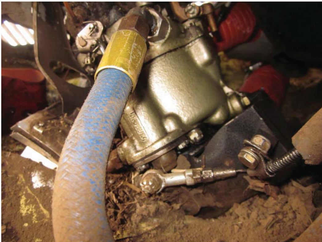
Carburetor heat linkage bent 90 degrees, unable to actuate due to damage.
