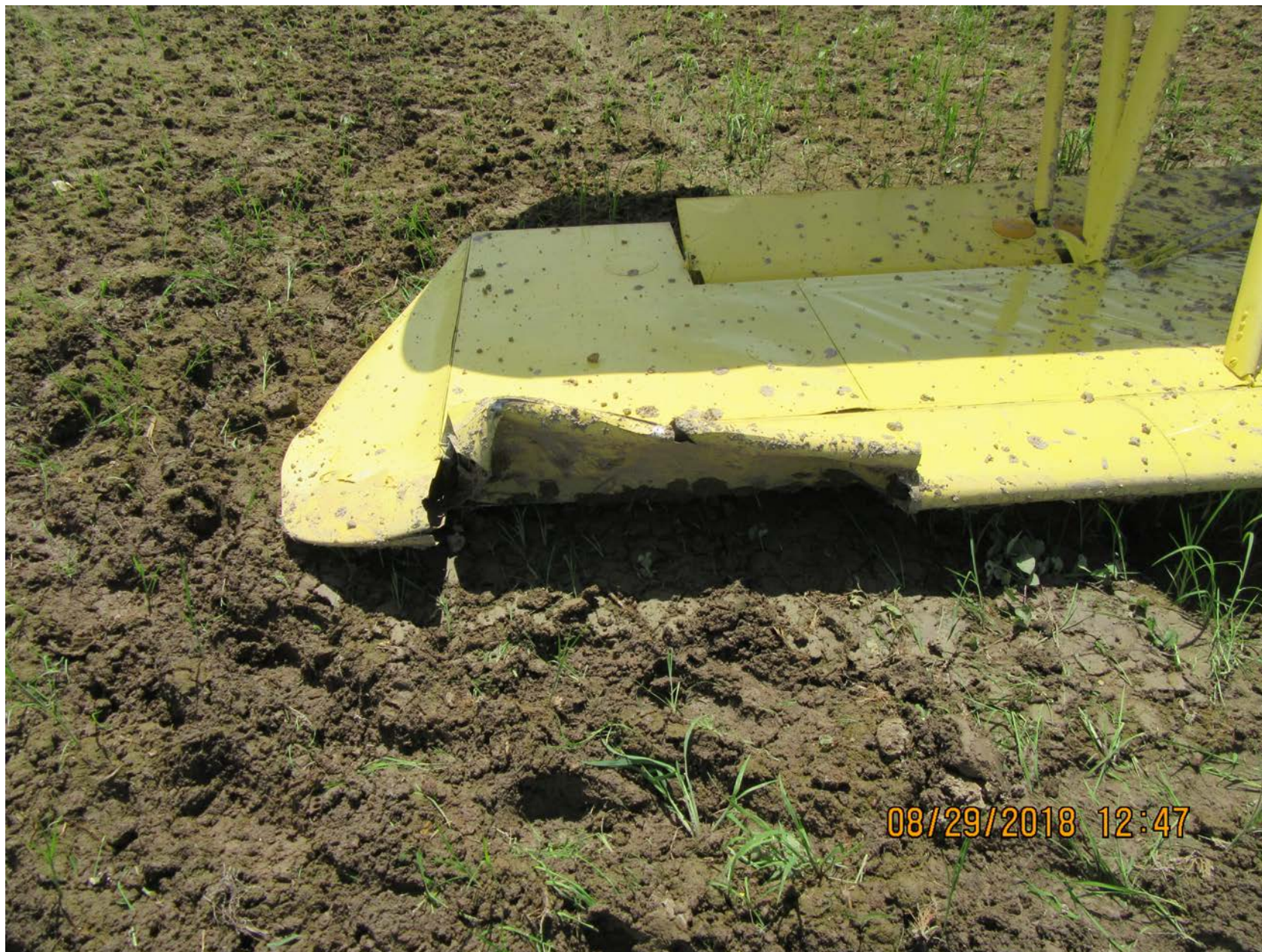
Photo 3 – Both upper wings sustained damage in the accident. This is the left upper wing leading edge.
