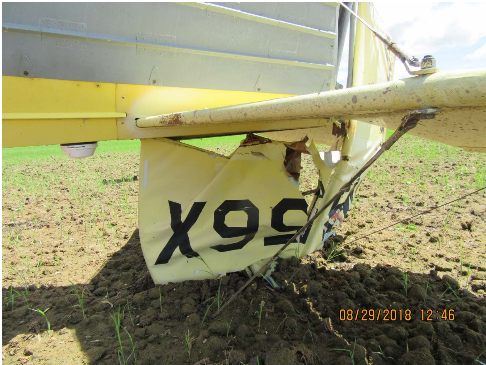
Photo 2 – Rudder and vertical stabilizer were crushed when the airplane overturned.
