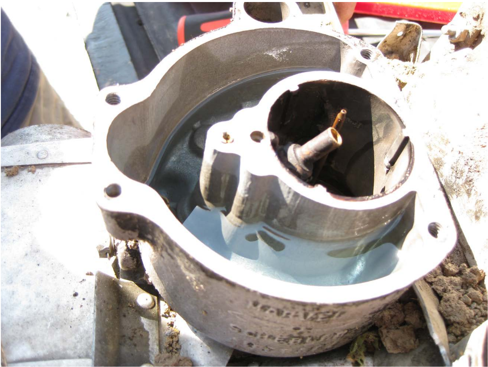
Photo 8 – View of the carburetor disassembled with fuel inside (courtesy of the Federal Aviation Administration).
