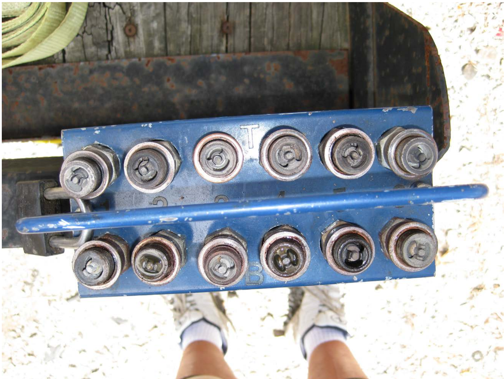
Photo 6 – View of the spark plugs (courtesy of the Federal Aviation Administration).
