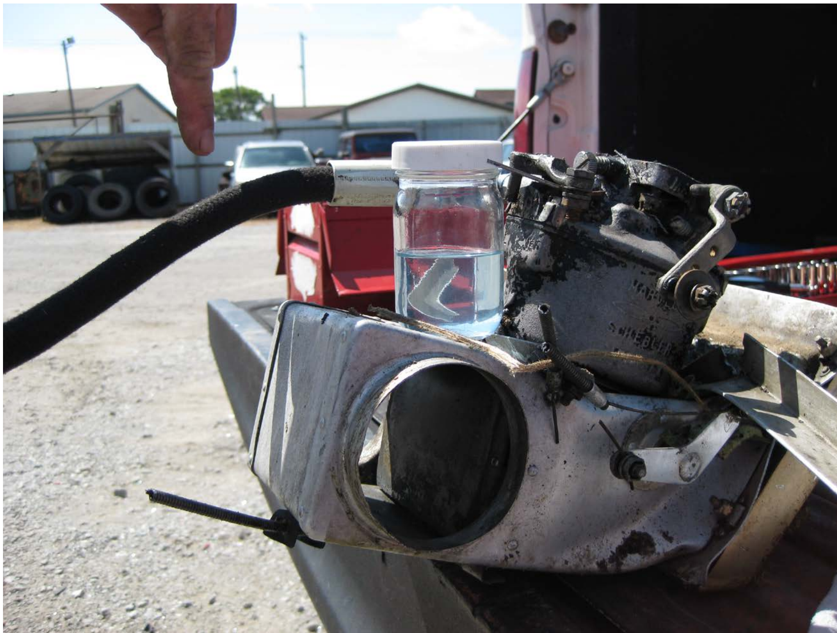
Photo 7 – View of the carburetor and fuel sample (courtesy of the Federal Aviation Administration).
