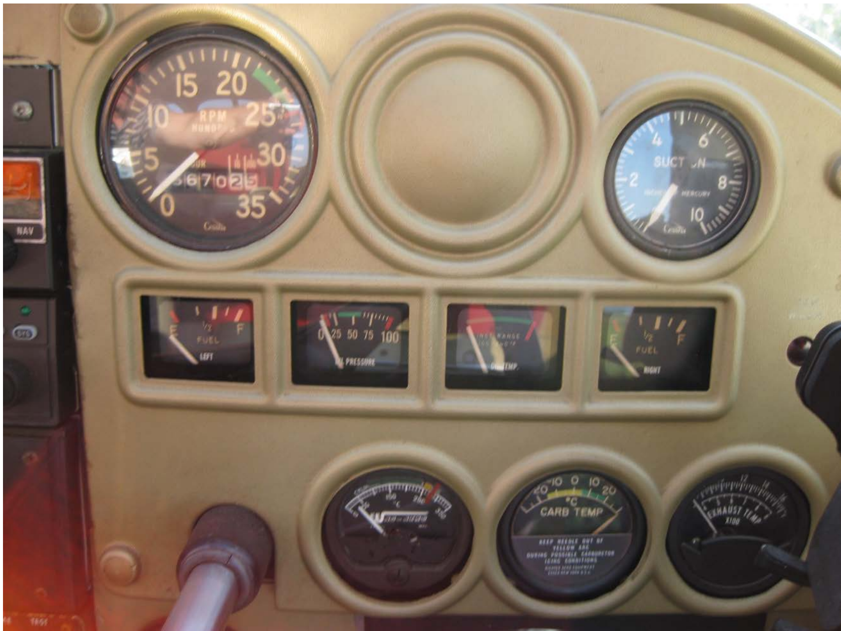
Photo 4 – View of the carburetor temperate gauge in the cockpit (courtesy of the Federal Aviation Administration).
