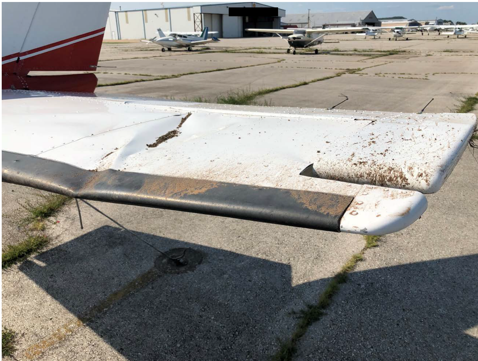
Photo 2 – Substantial Damage to Left Horizontal Stabilizer
