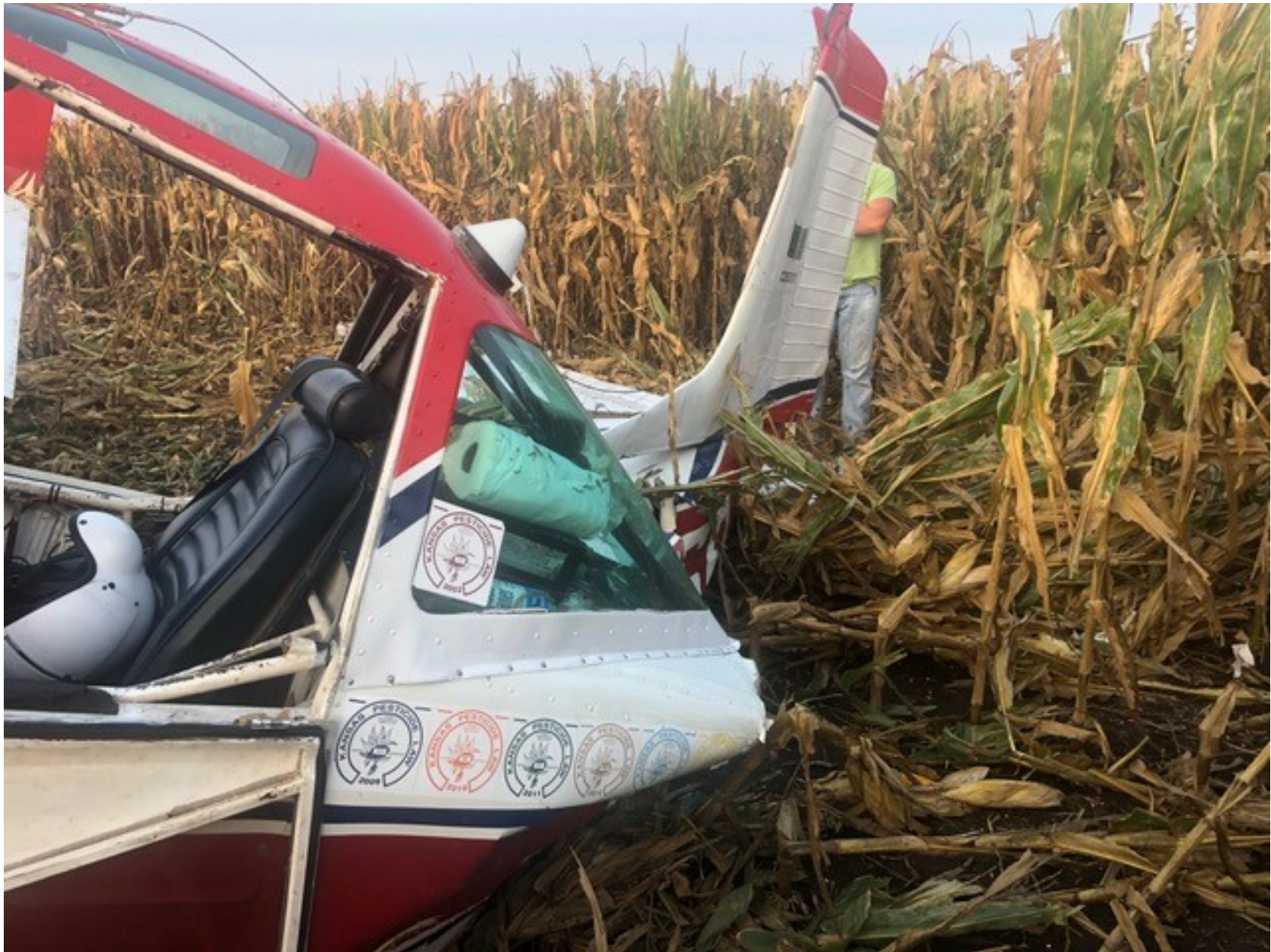
Photo 3 – Empennage Damage (Photo from Pilot)
