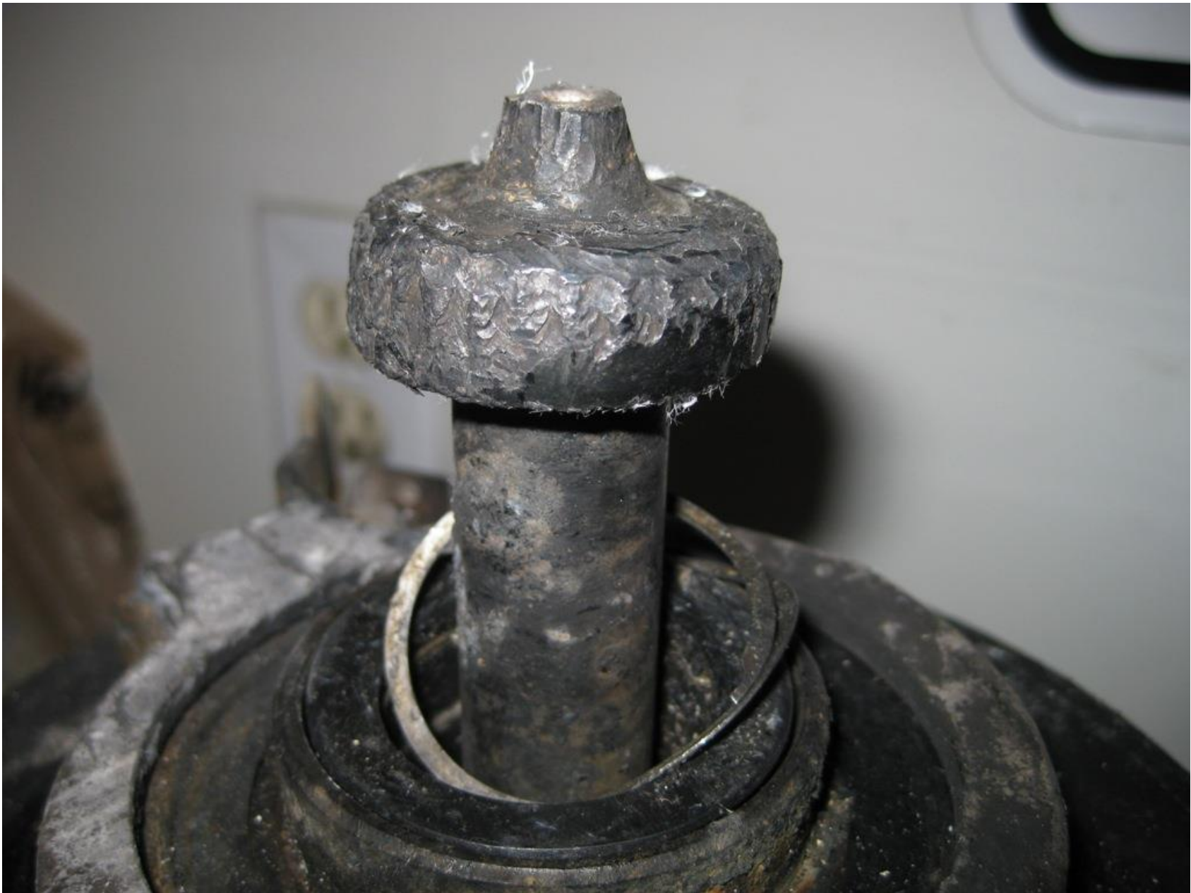
Photo 2 – Lower Coupling Drive Shaft, Forward End
