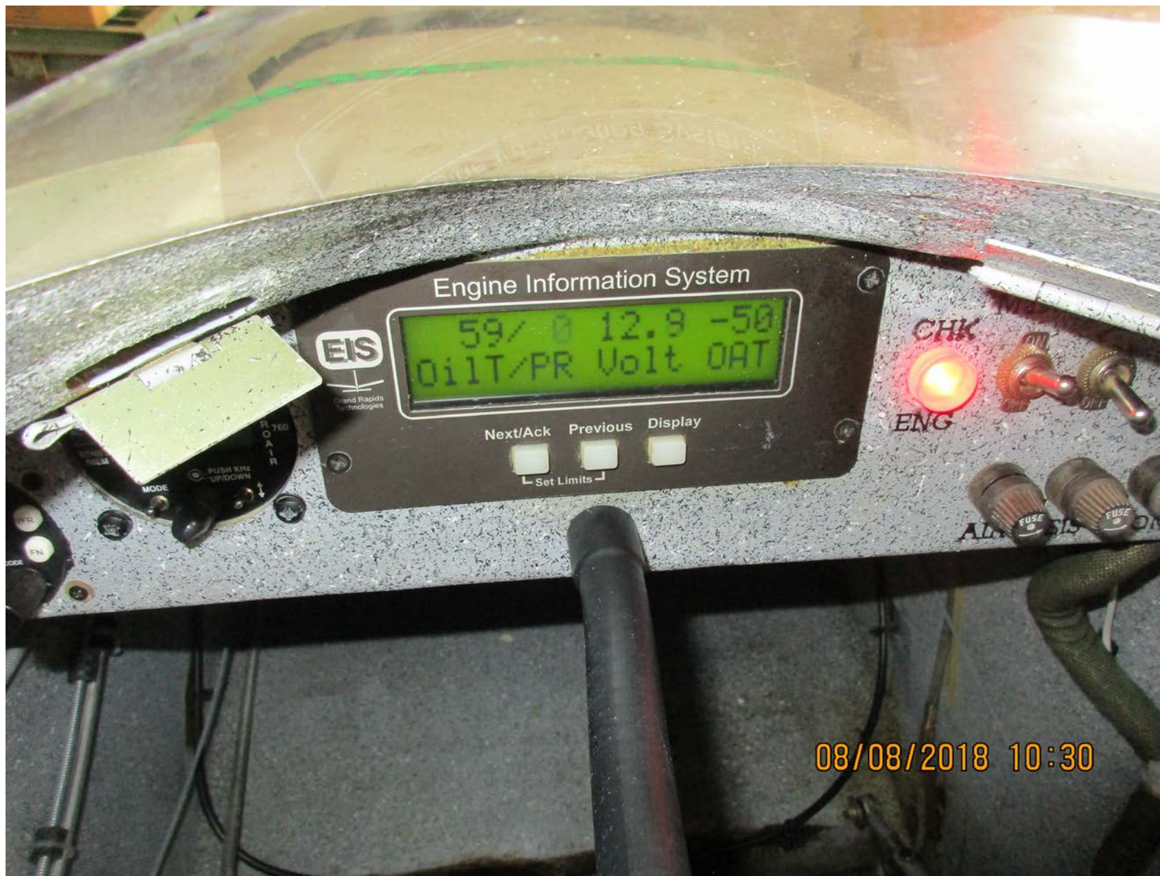
Photo 10 - FAA supplied close up photo of the engine monitor indicating a voltage of 12.9 volts.
