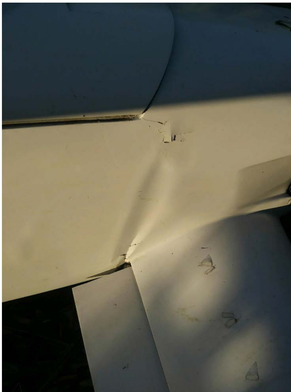
Photo 2 - FAA supplied close up photo of a deformation in the fuselage skin.
