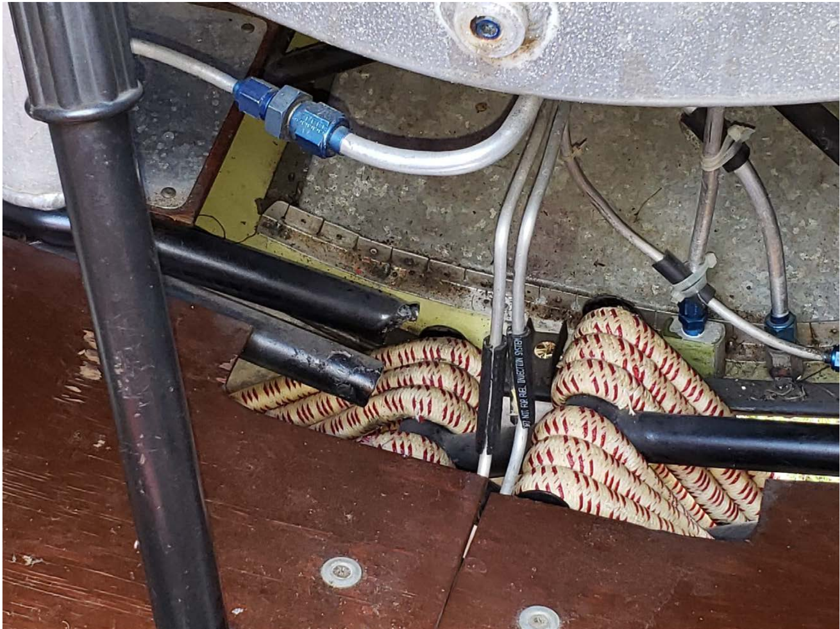
Photo 2 - View at flooring inside cockpit. Note fractured landing gear shock cord truss.
