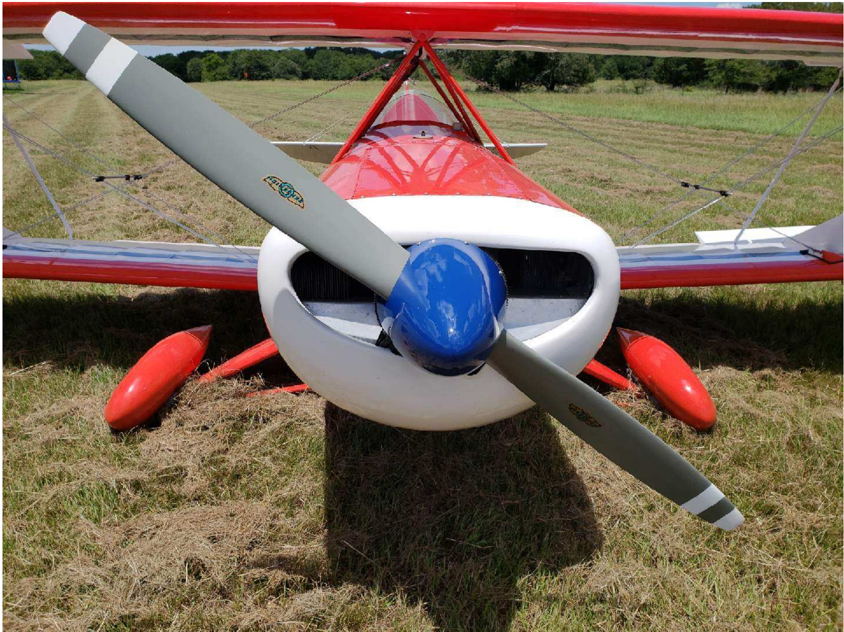
Photo 1 – The Steen Skybolt, N22GL, at the end of the runway. Note how the main landing gear has spread apart and the airplane has settled.
