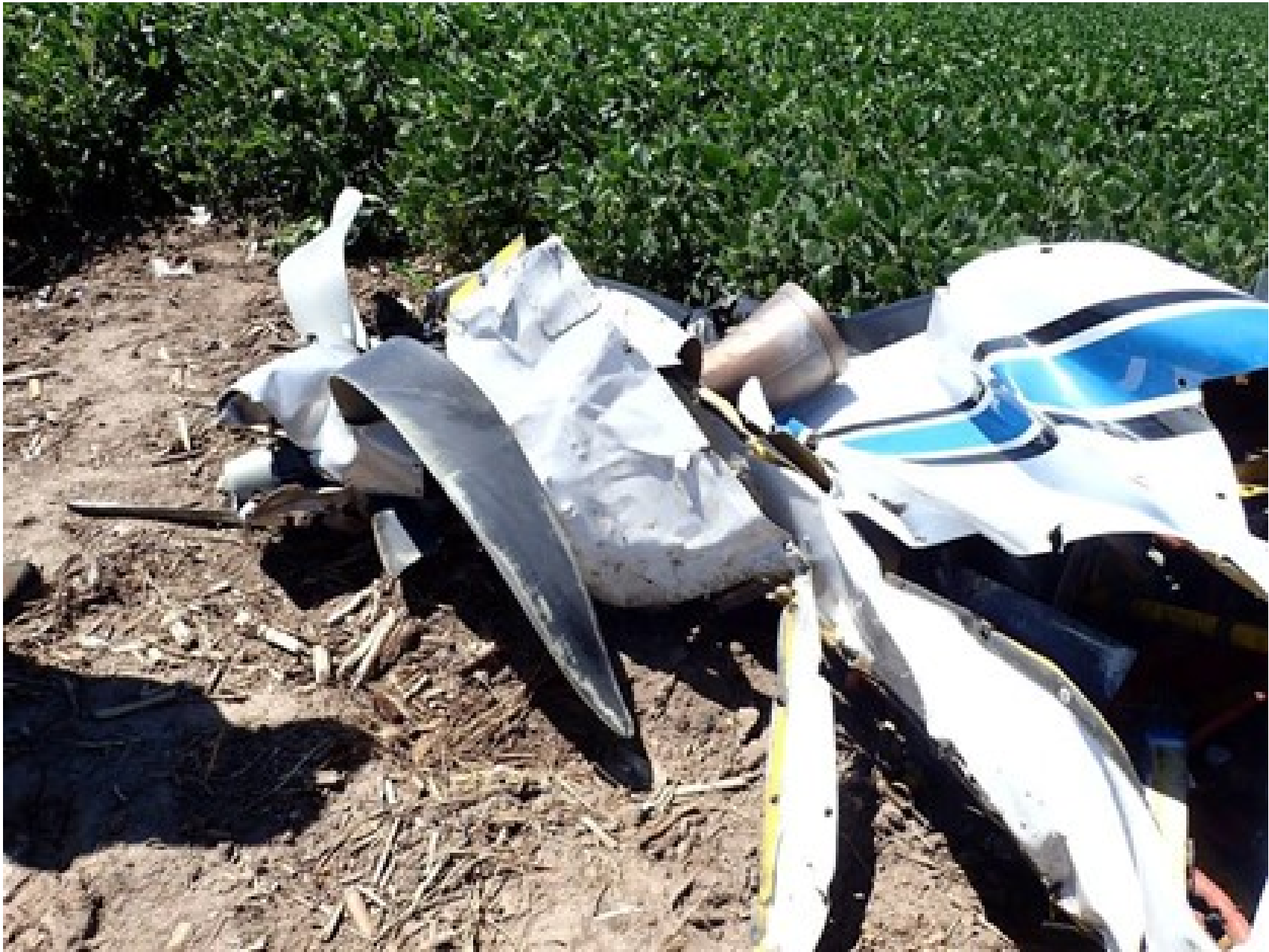
Photo 4 – View of Engine and Propeller with Chordwise Damage
