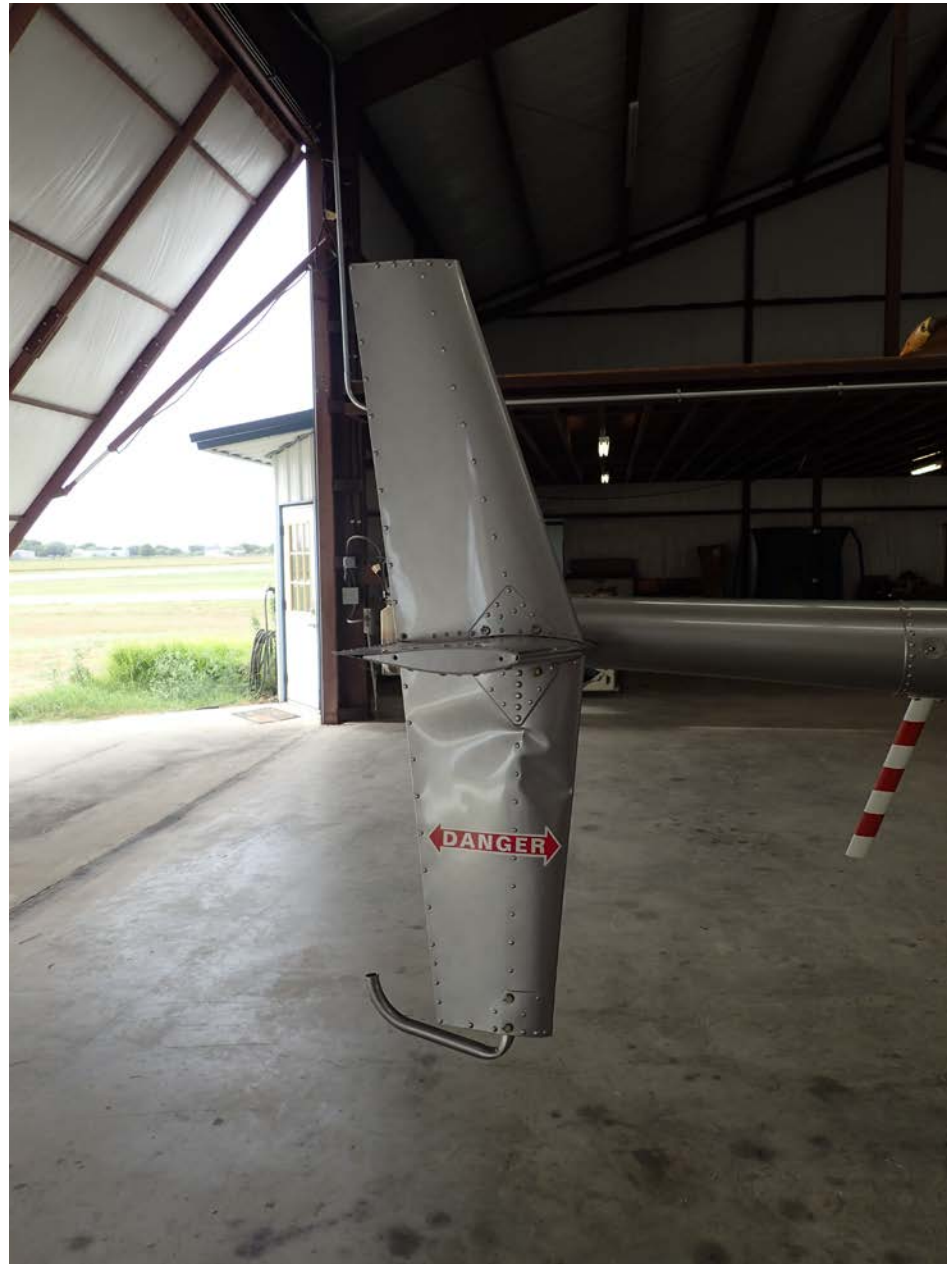
Photo 5 – View of the substantial damage to the vertical stabilizer.
