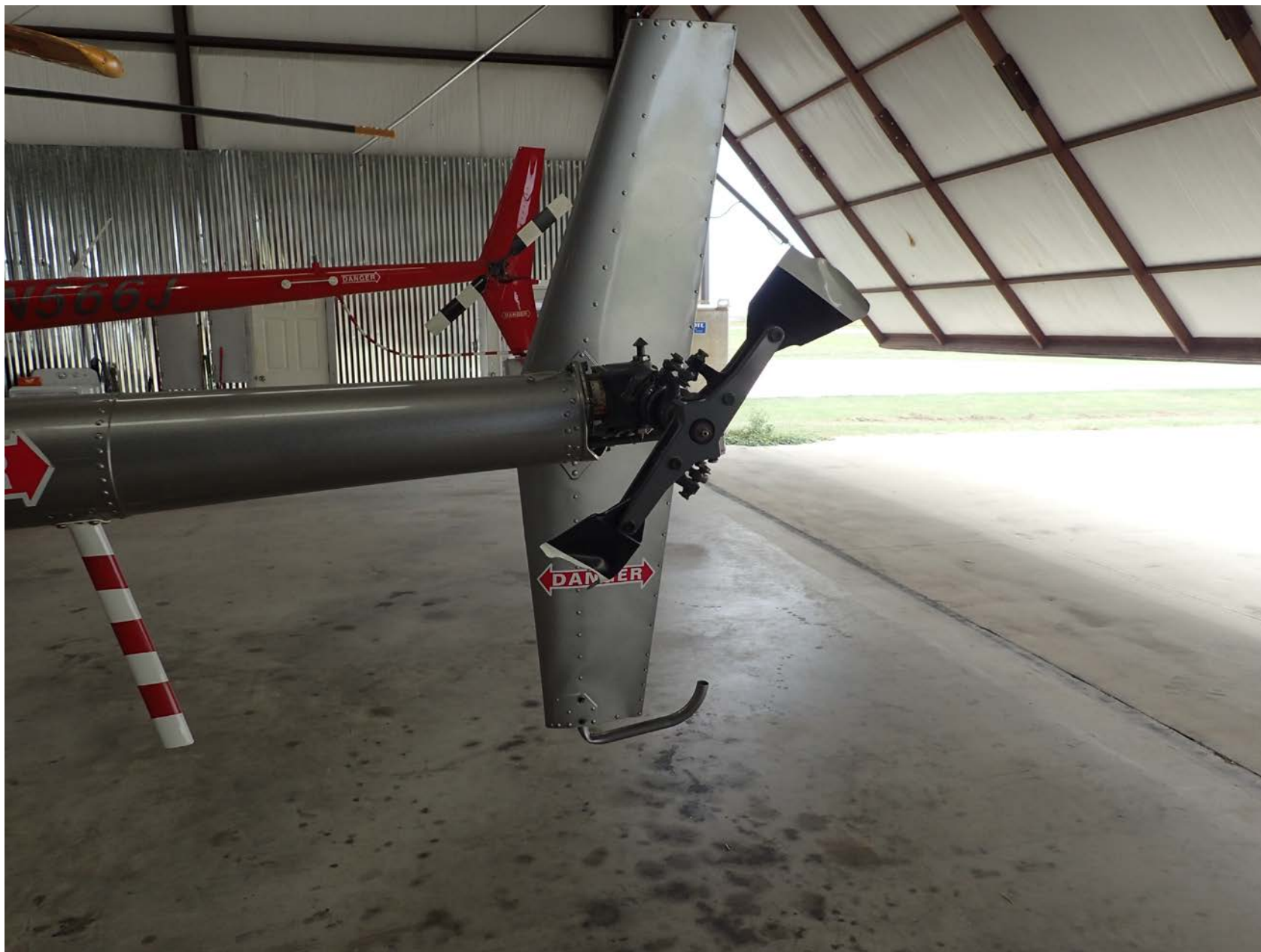
Photo 6 – View of the impact damage to the tail rotor blades.
