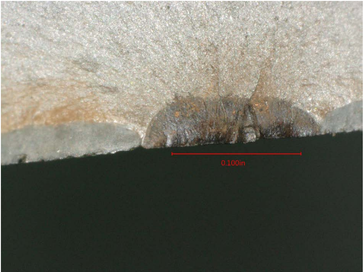
Figure 4:Thumbnail shaped fatigue crack at fracture origin.
