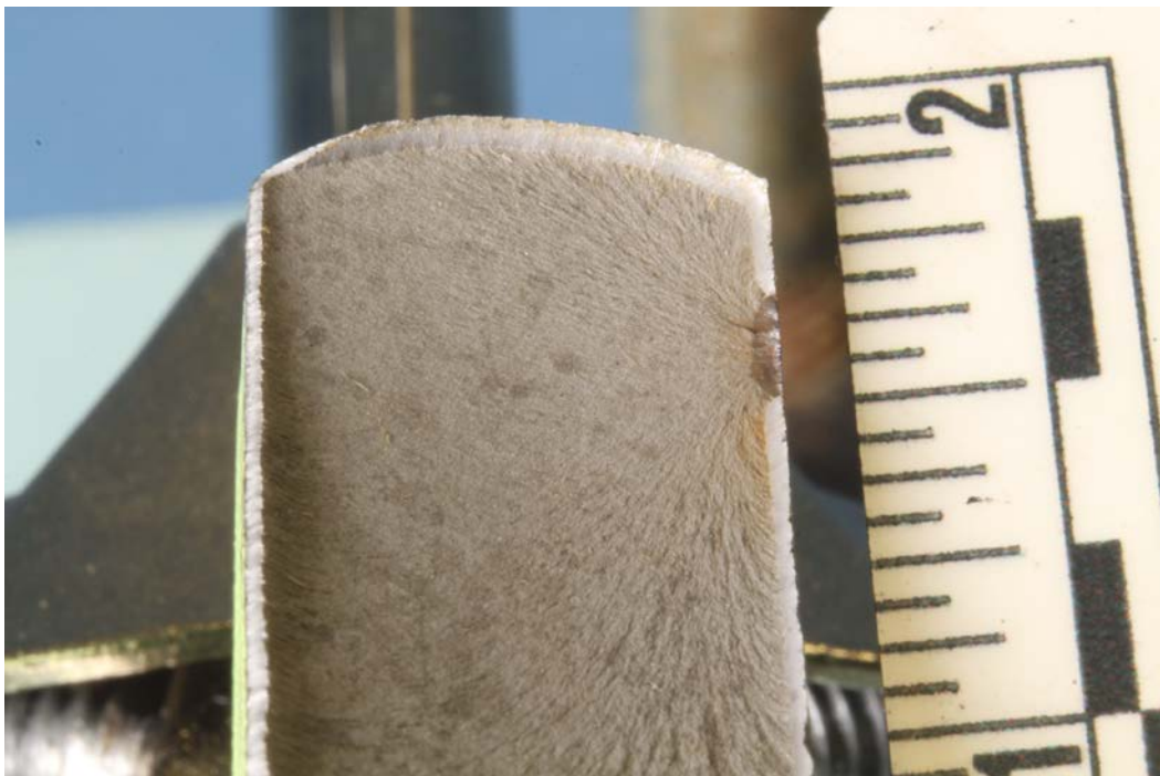
Figure 3: Thumbnail shaped area at the fracture origin.
