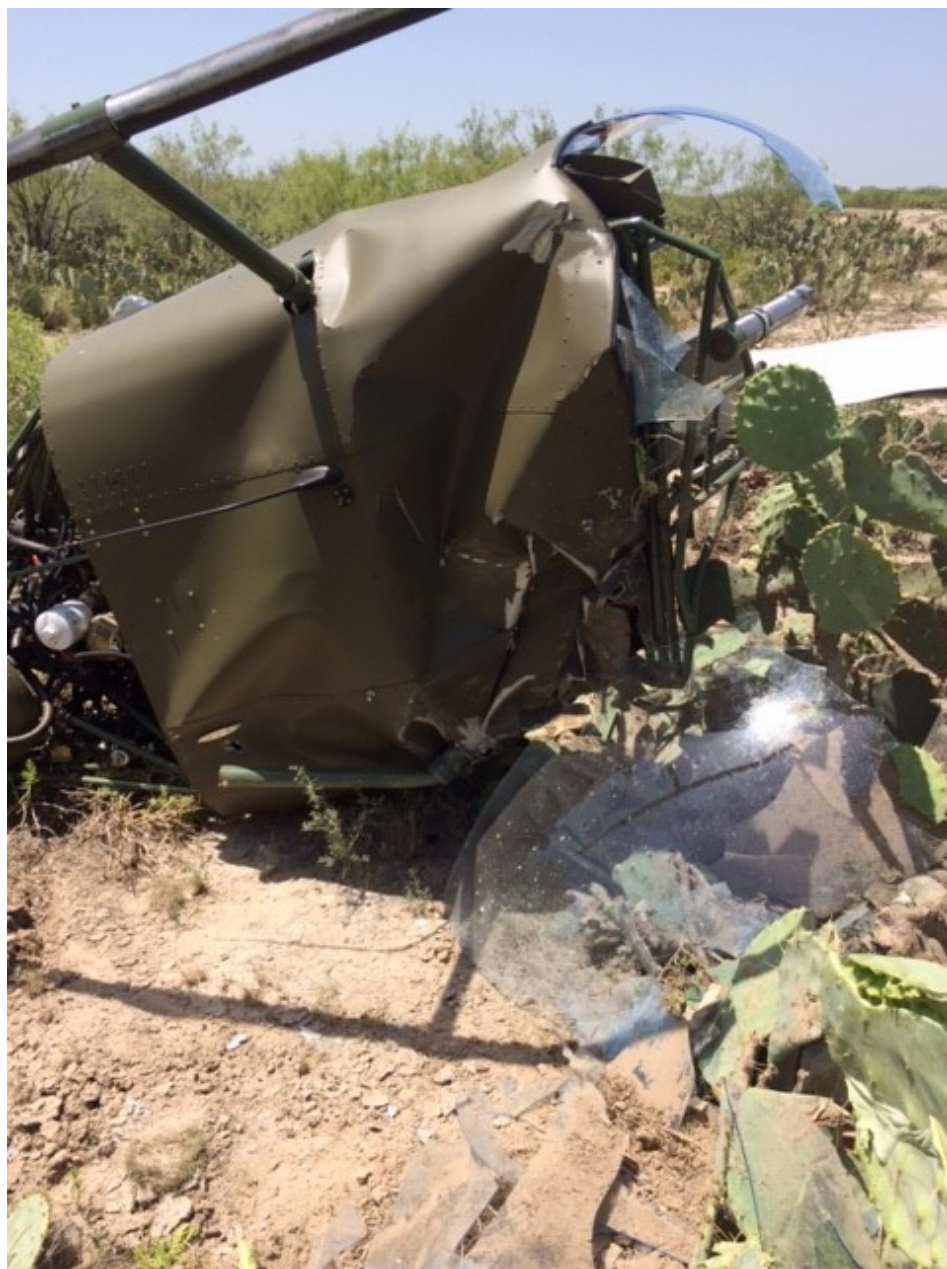
Photograph 4 – Lower Fuselage and Skids (provided by FAA)
