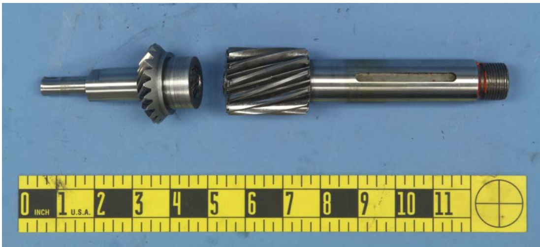
Figure 1: Two portions of a tail rotor pinion shaft as received.
