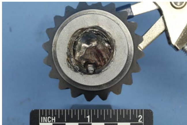
Figure 2: Fracture surface on both the beveled gear side and helical gear side.
