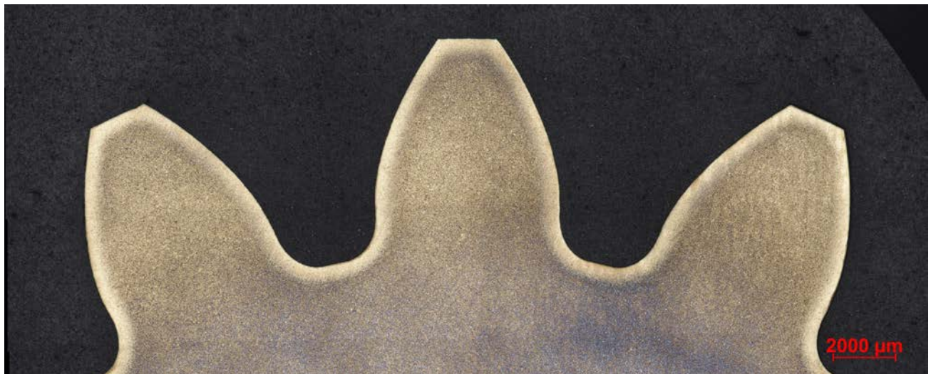
Figure 7: Micrograph of polished and etched portion of the pinion shaft and helical gear.
