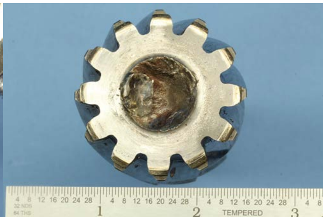
Figure 2: Fracture surface on both the beveled gear side and helical gear side.
