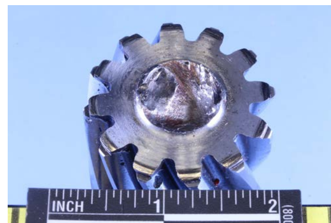
Figure 3: Fracture surface on both the beveled gear side and helical gear side.
