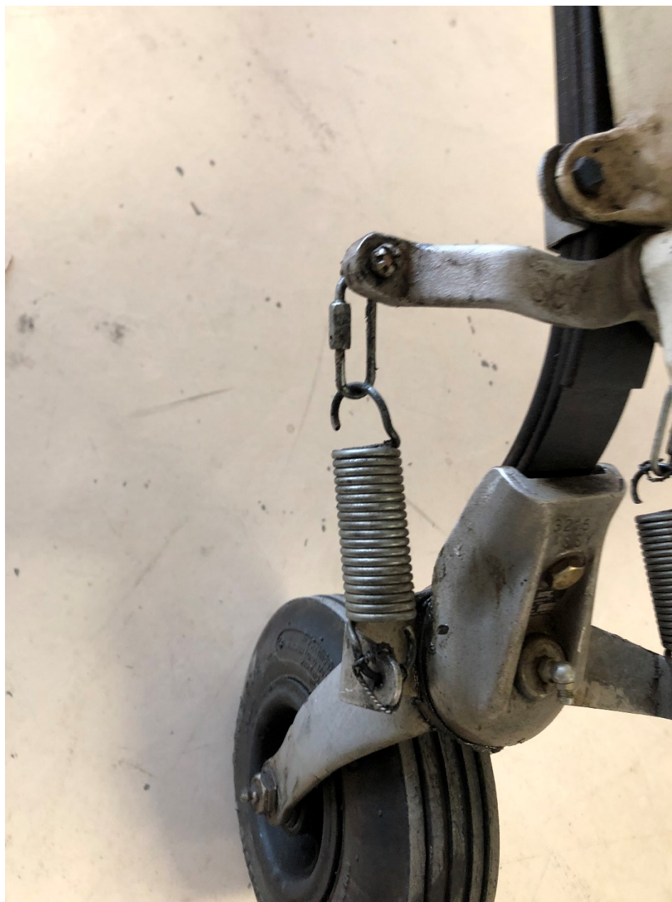
Photo 3 – Reattached Left Rudder Spring
