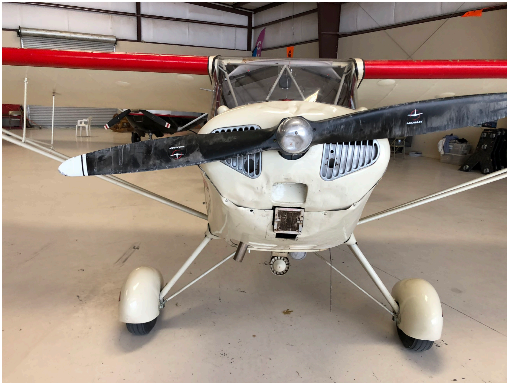
Photo 1 – Damage to Nose Section of the Airplane
