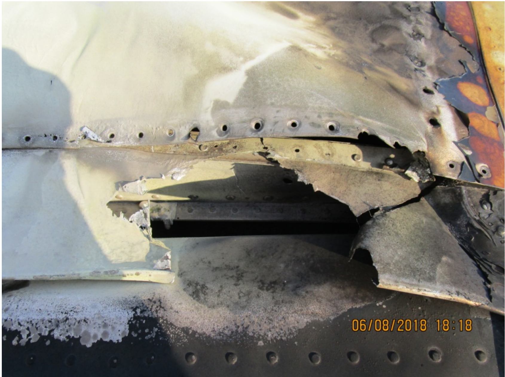
Photo 3 - Closeup view of fire damage to the right wing (FAA Photo)
