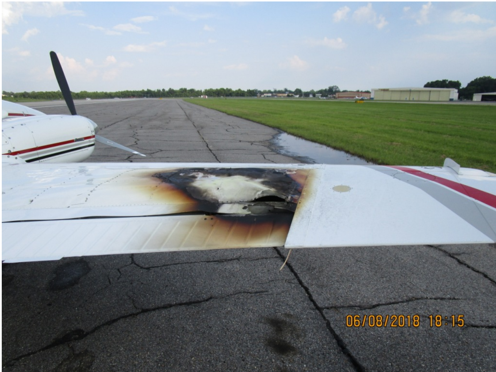
Photo 1 – View of fire damage to the right wing (FAA Photo)
