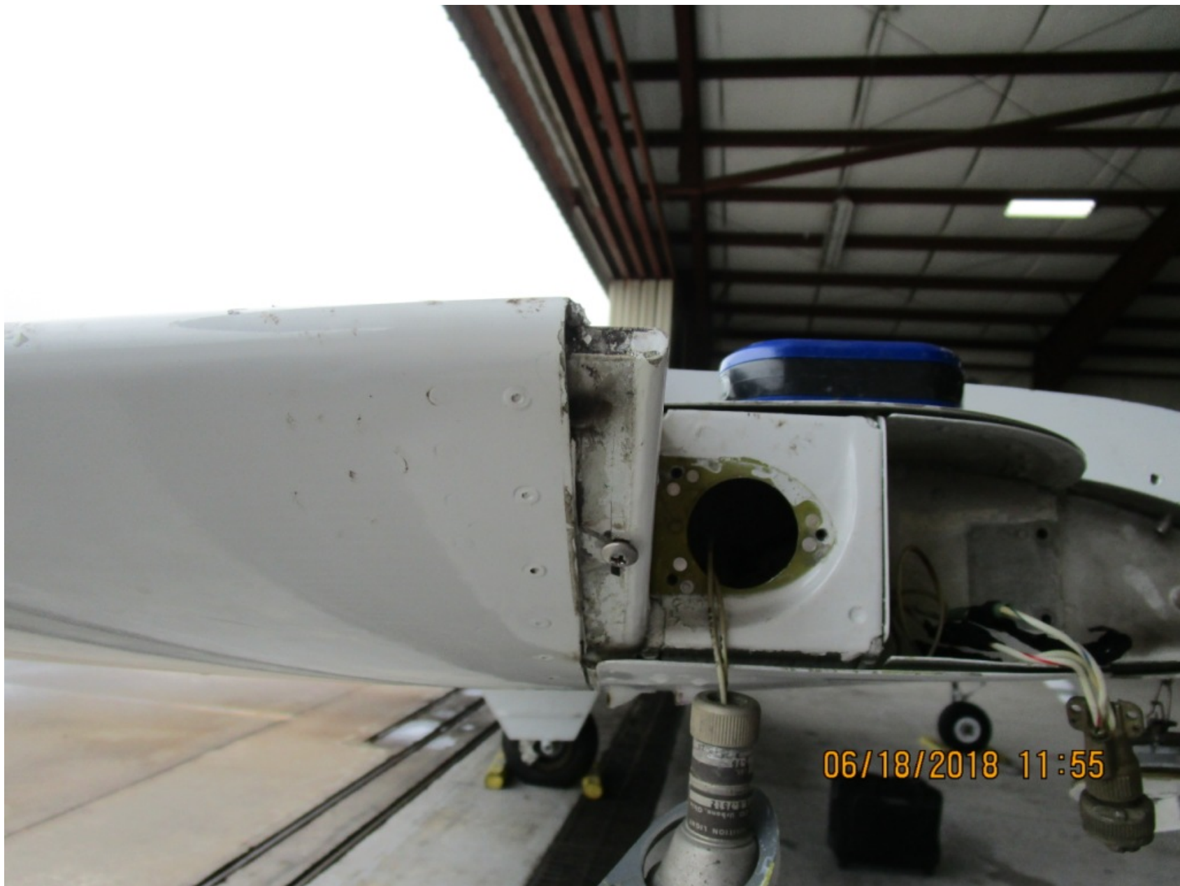
Photo 8 – View of soot near the right navigation light (FAA Photo)
