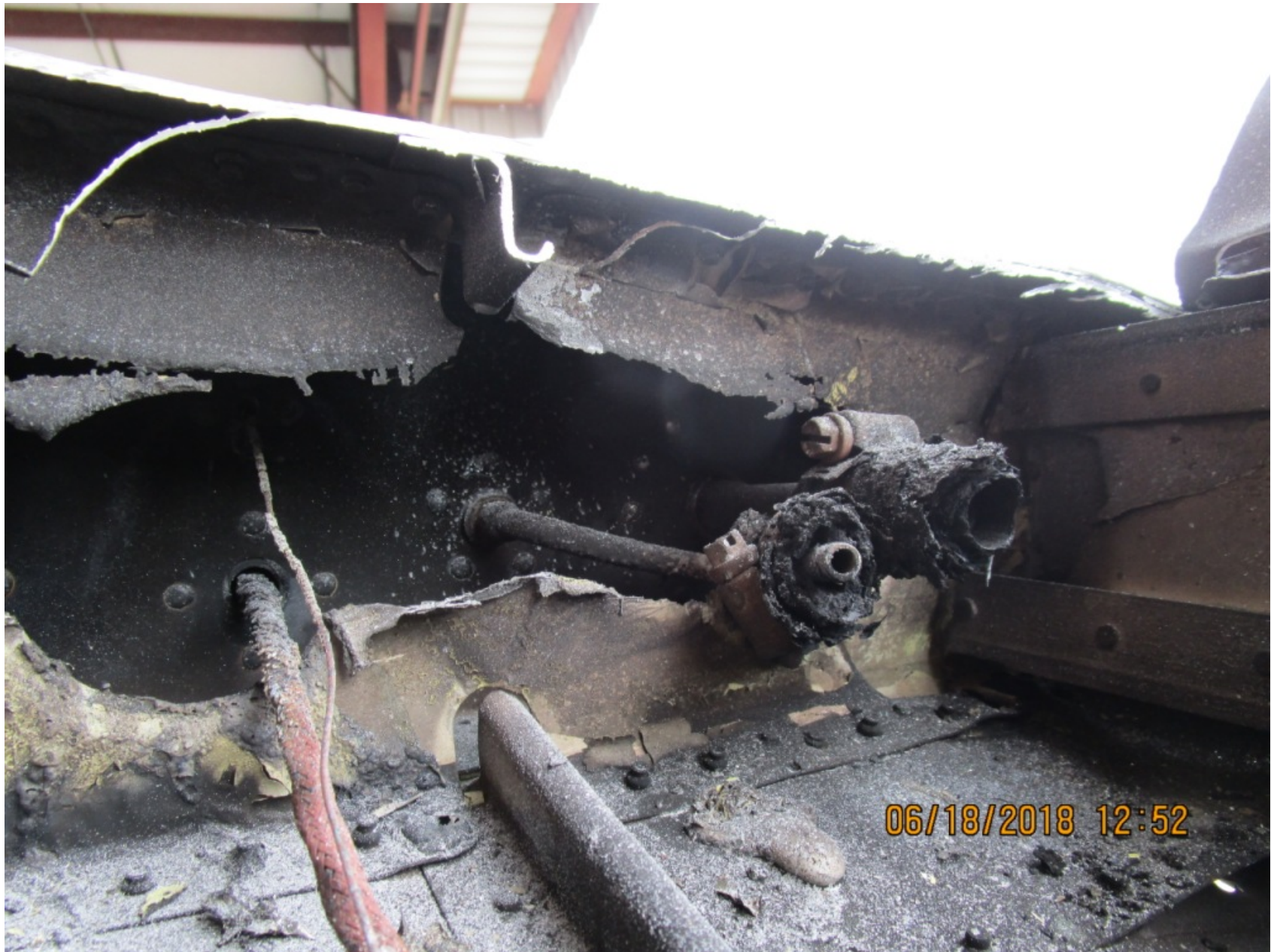
Photo 10 – View of the fire damage to the inside of the right wing (FAA Photo)
