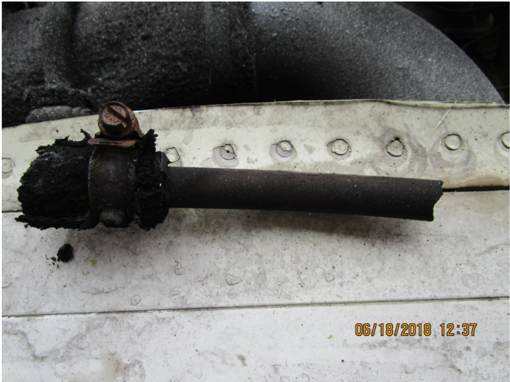
Photo 11 - View of the fire damage to a line in the right wing (FAA Photo)
