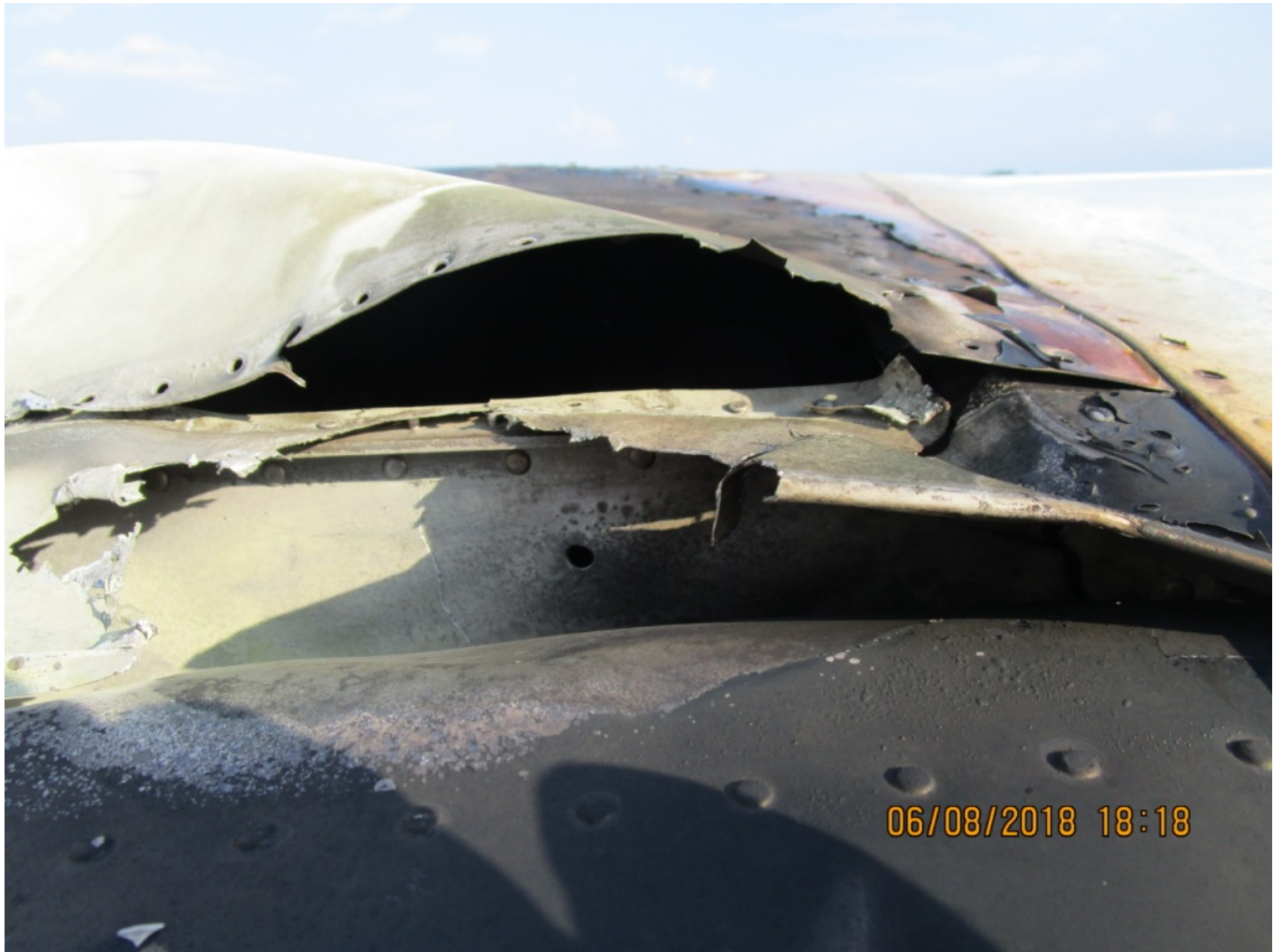
Photo 2 – Closeup view of fire damage to the right wing (FAA Photo)
