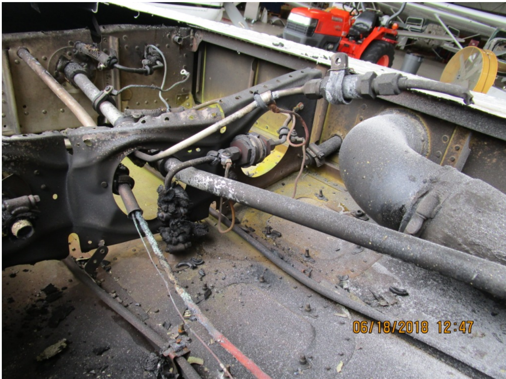
Photo 12 - View of the fire damage to the inside of the right wing (FAA Photo)
