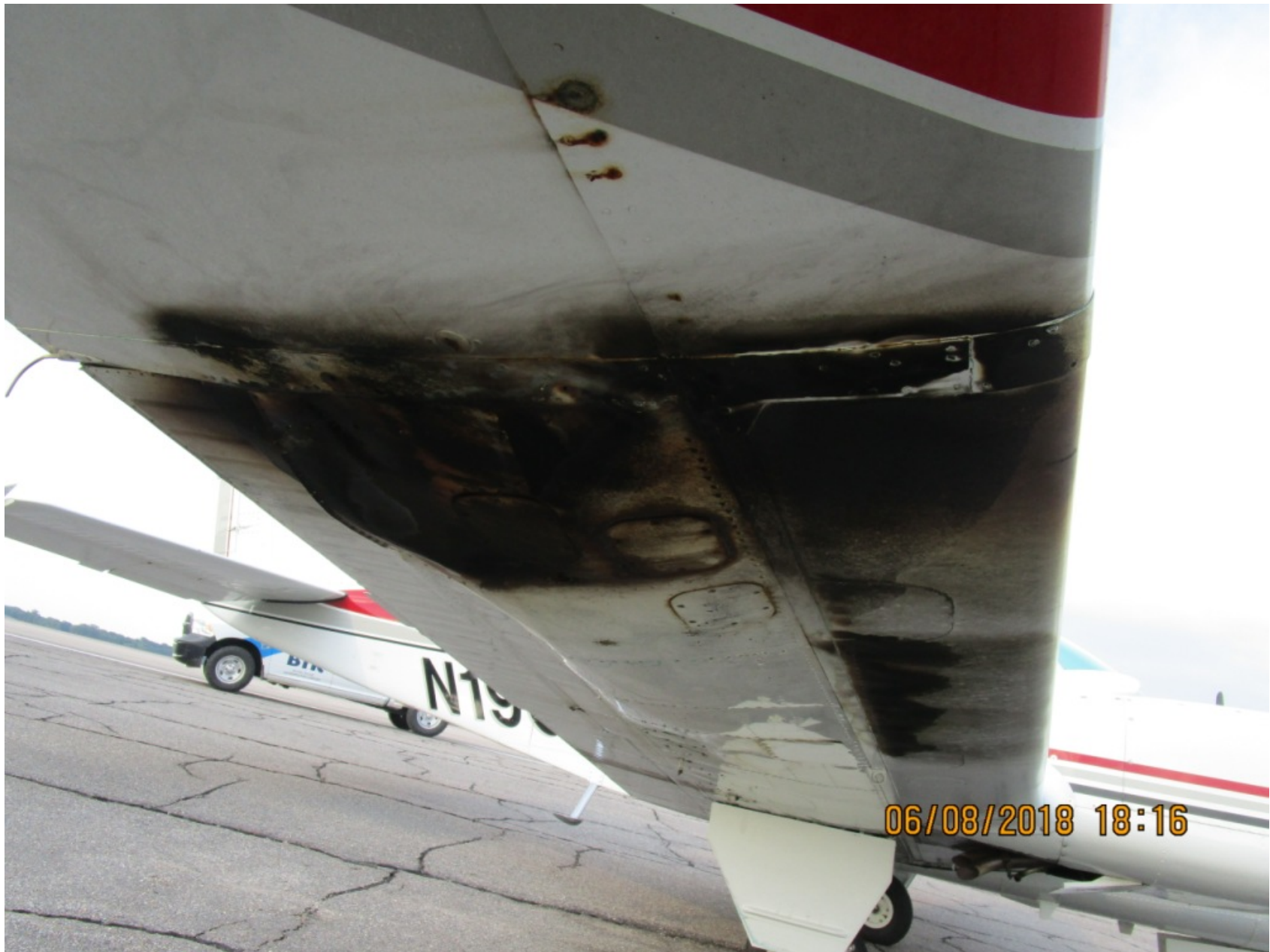
Photo 4 – View of the fire damage to the bottom of the wing (FAA Photo)
