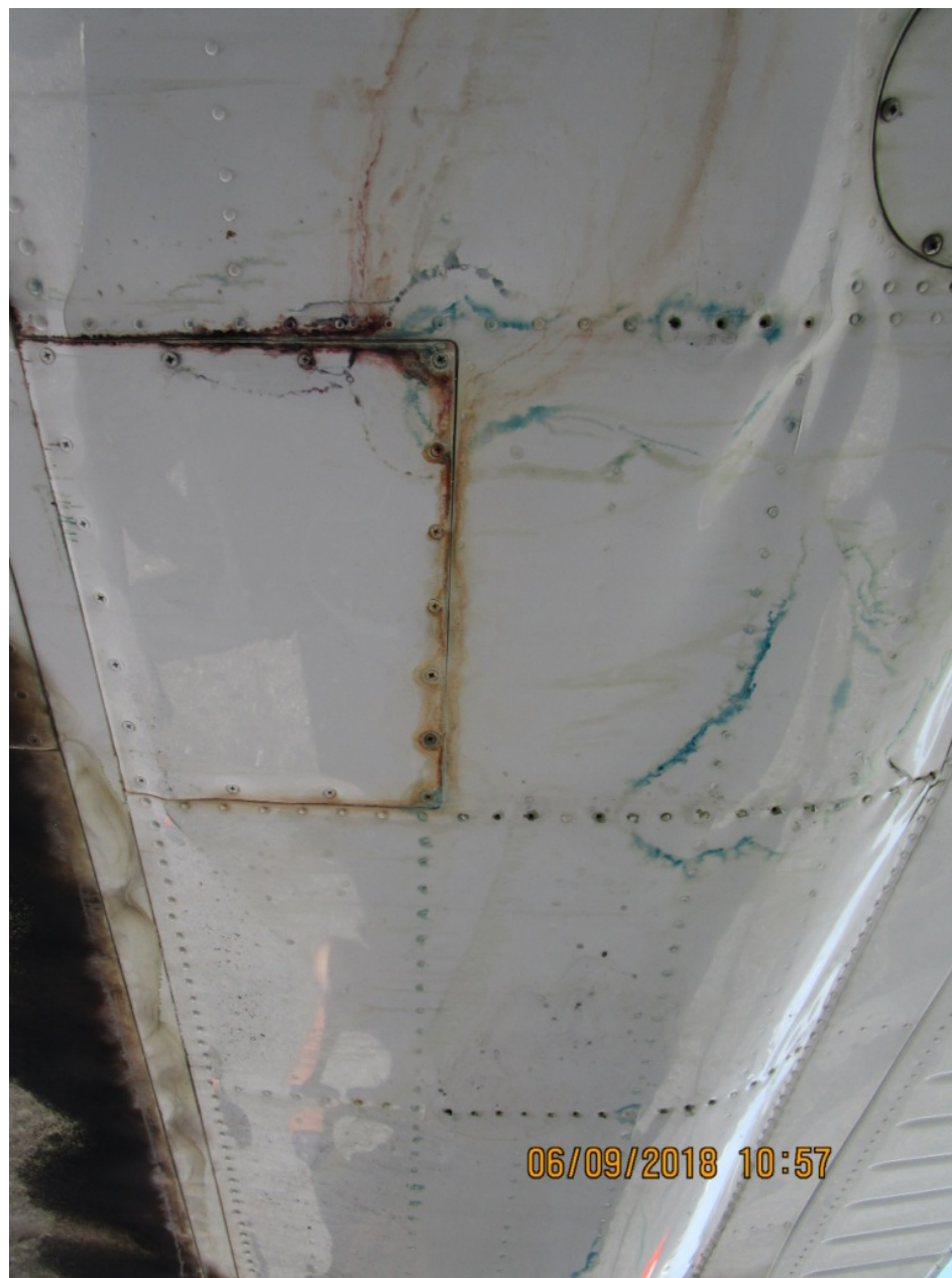
Photo 7 – View of fuel stains on the bottom side of the right wing (FAA Photos)
