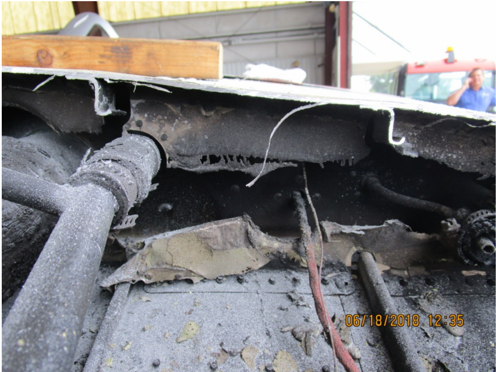
Photo 9 – View of the fire damage to the inside of the right wing (FAA Photo)
