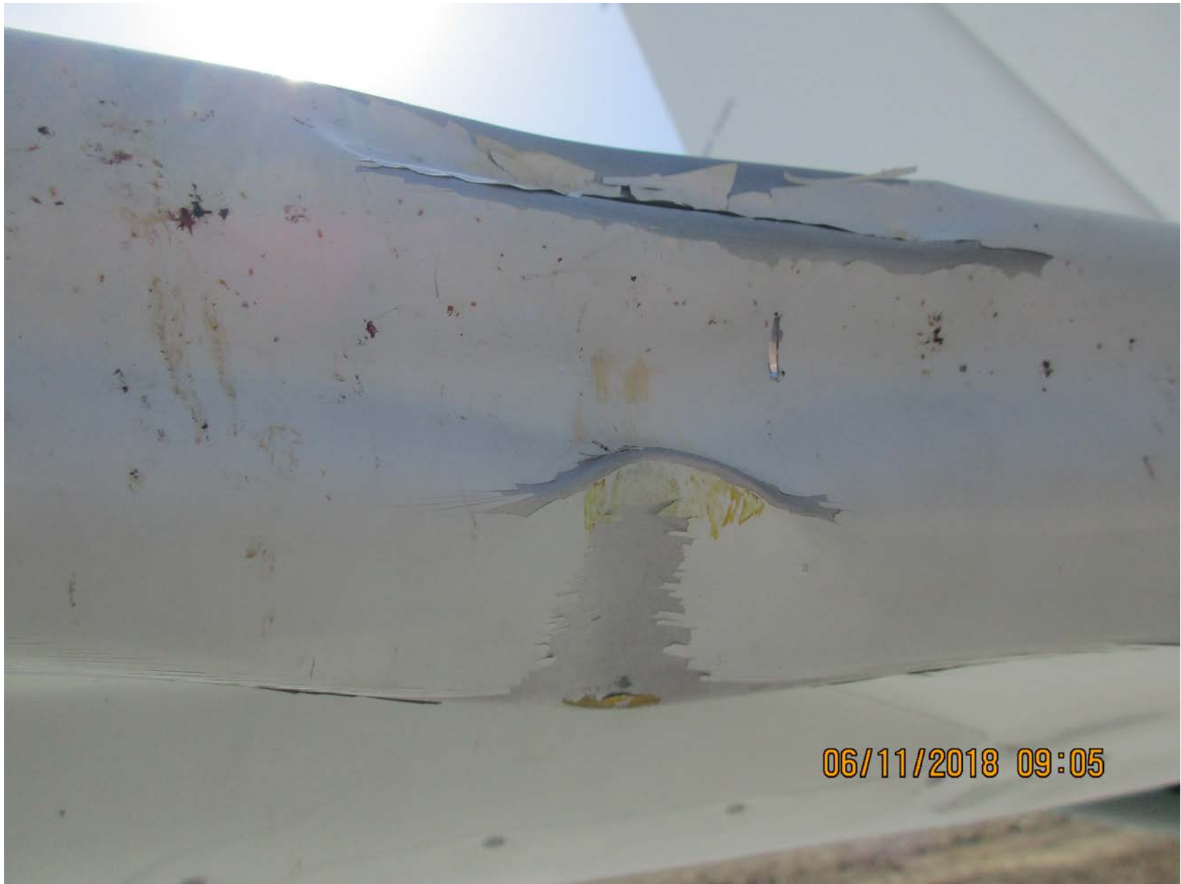
Photo 2 – Closeup of Leading Edge Damage
