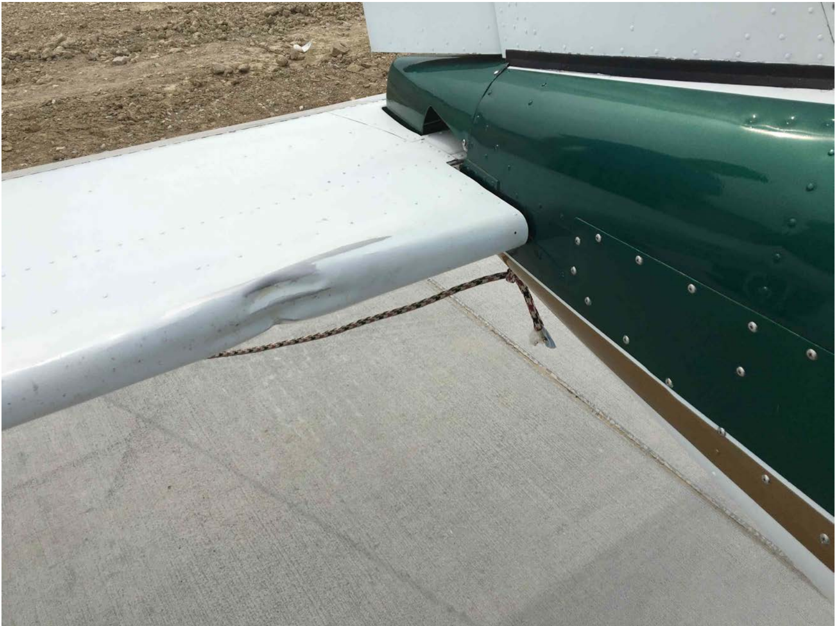
Photo 1 – Right Side Horizontal Stabilizer Leading Edge Damage
