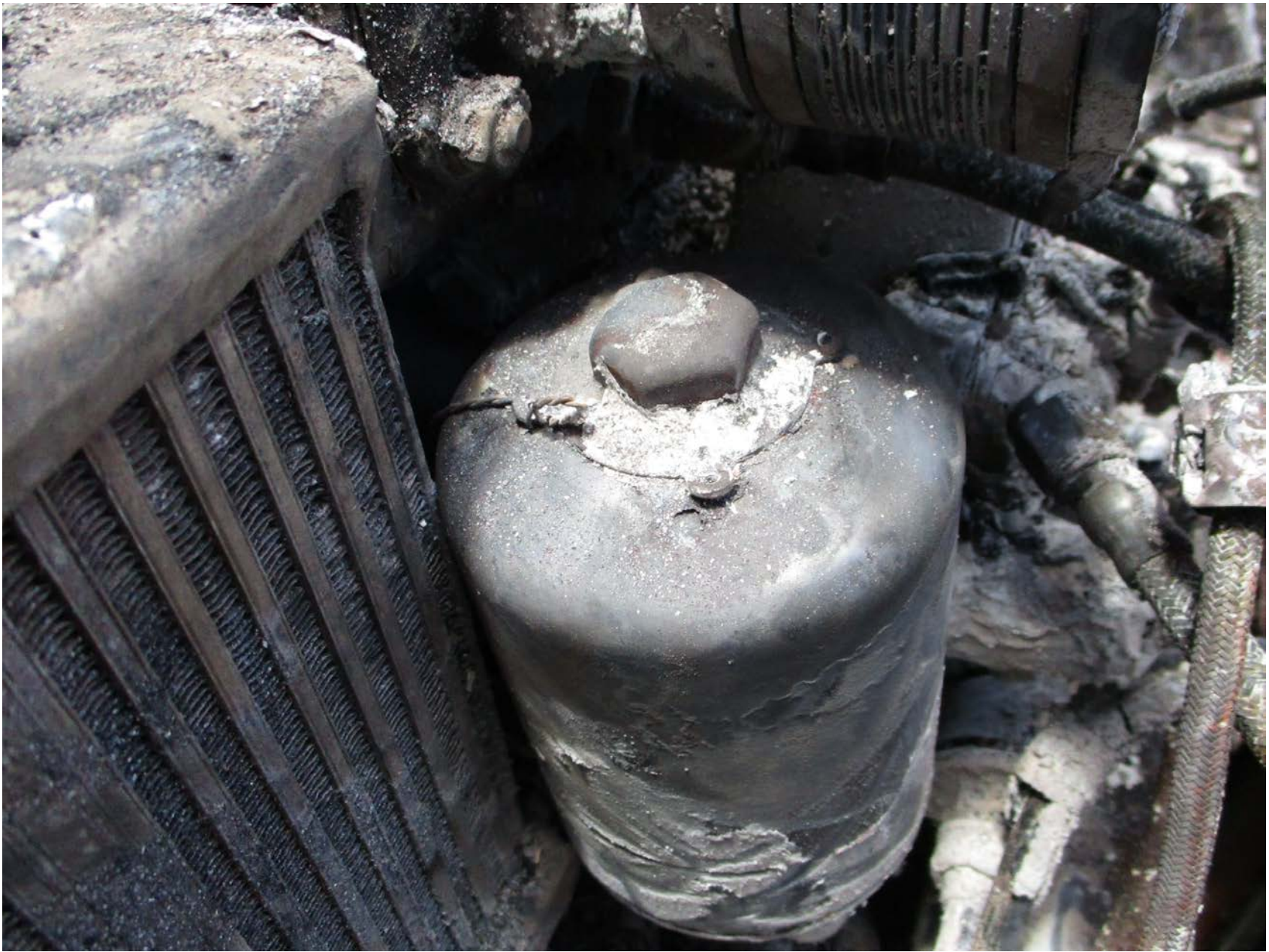
Photo 5 – Oil filter and safety wire
