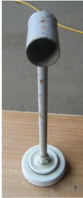
An early style vented fuel cap is shown above
