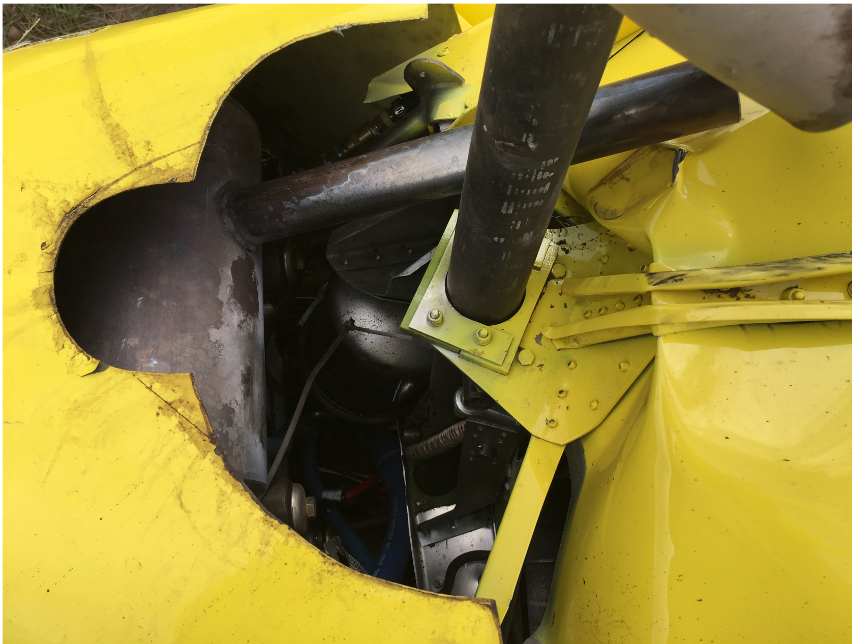
Photo 2 – Close-up of Damage to Structure at Nose Wheel Strut
