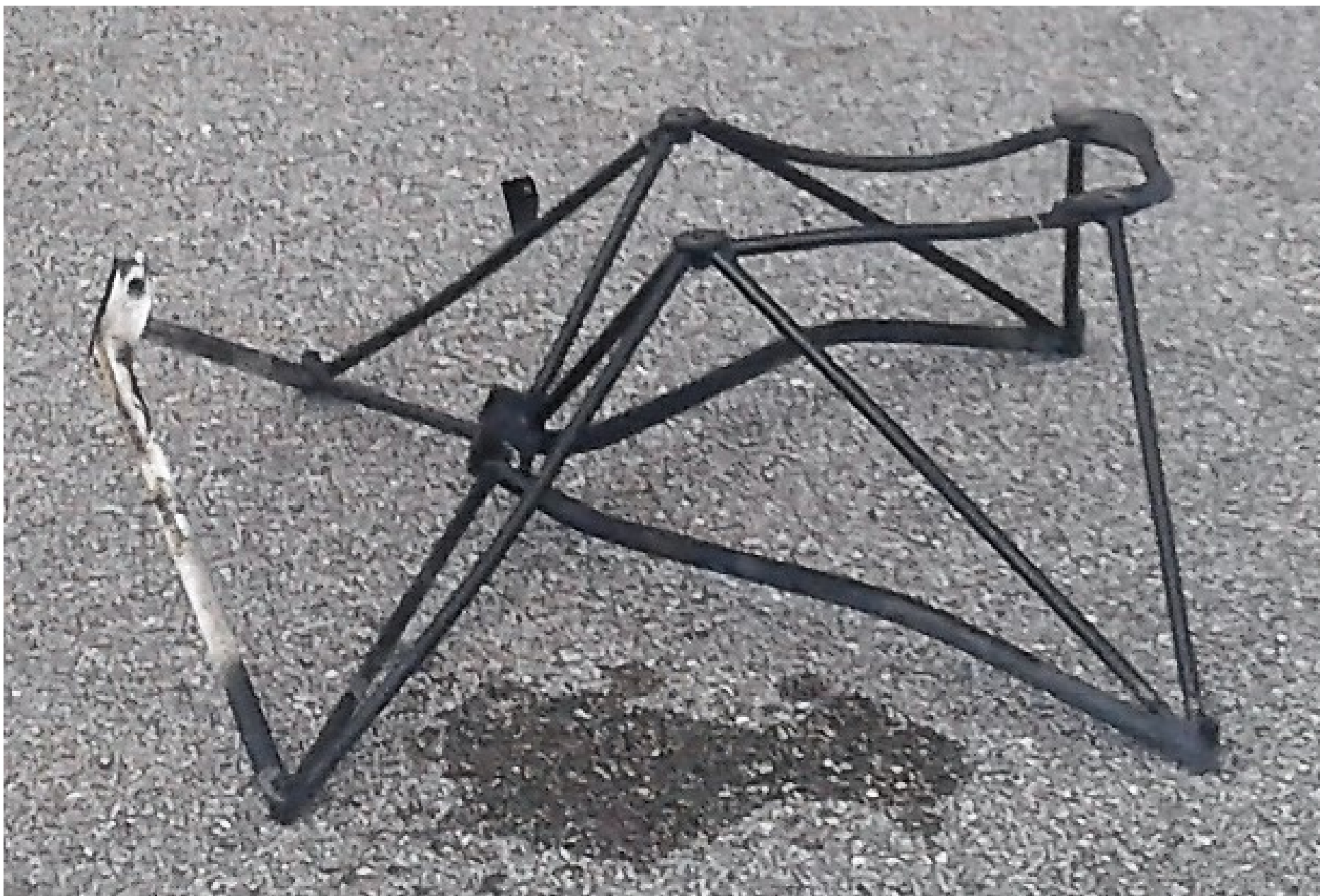
Photo 3 – Bent engine mount (Pilot photo)
