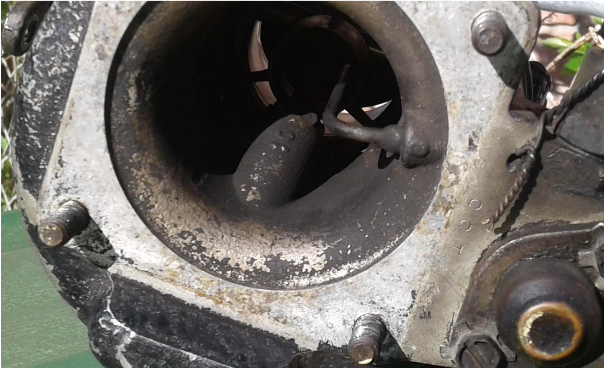
Photo 5 – View of carburetor venturi (Pilot photo)
