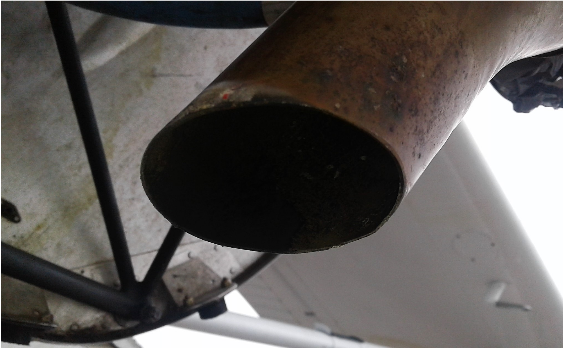
Photo 6 – View of black carbon in engine exhaust (Pilot photo)
