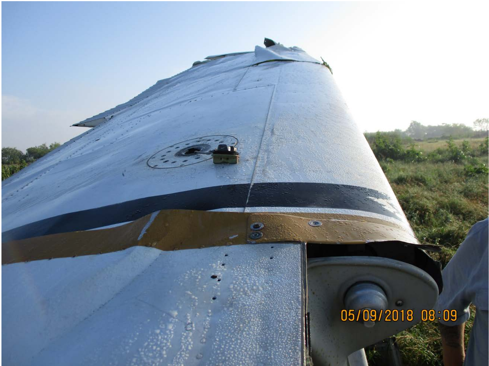
Photograph 2 – Left-Wing Fuel Cap (Provided by the FAA)
