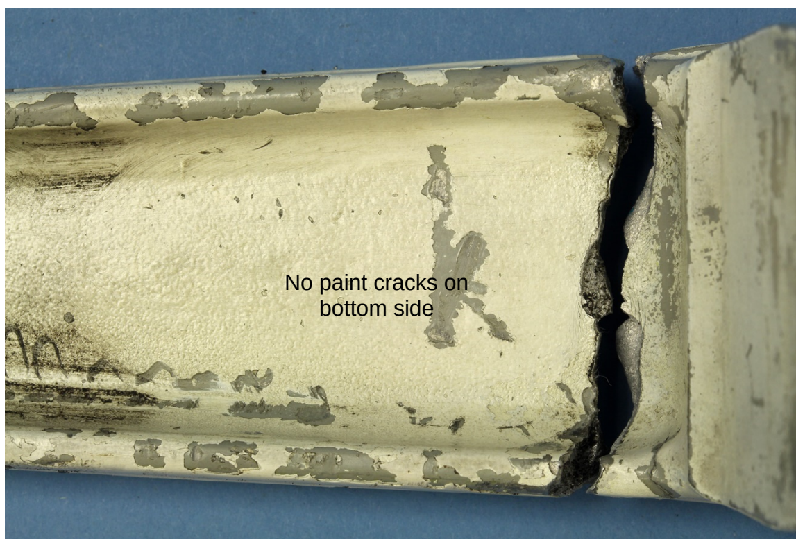
Figure 2 (cont.): c) image of the torque link assembly top side in the vicinity of the fracture showing cracks in the paint; and d) image of the bottom side in the vicinity of the fracture where no cracks were observed in the paint.
