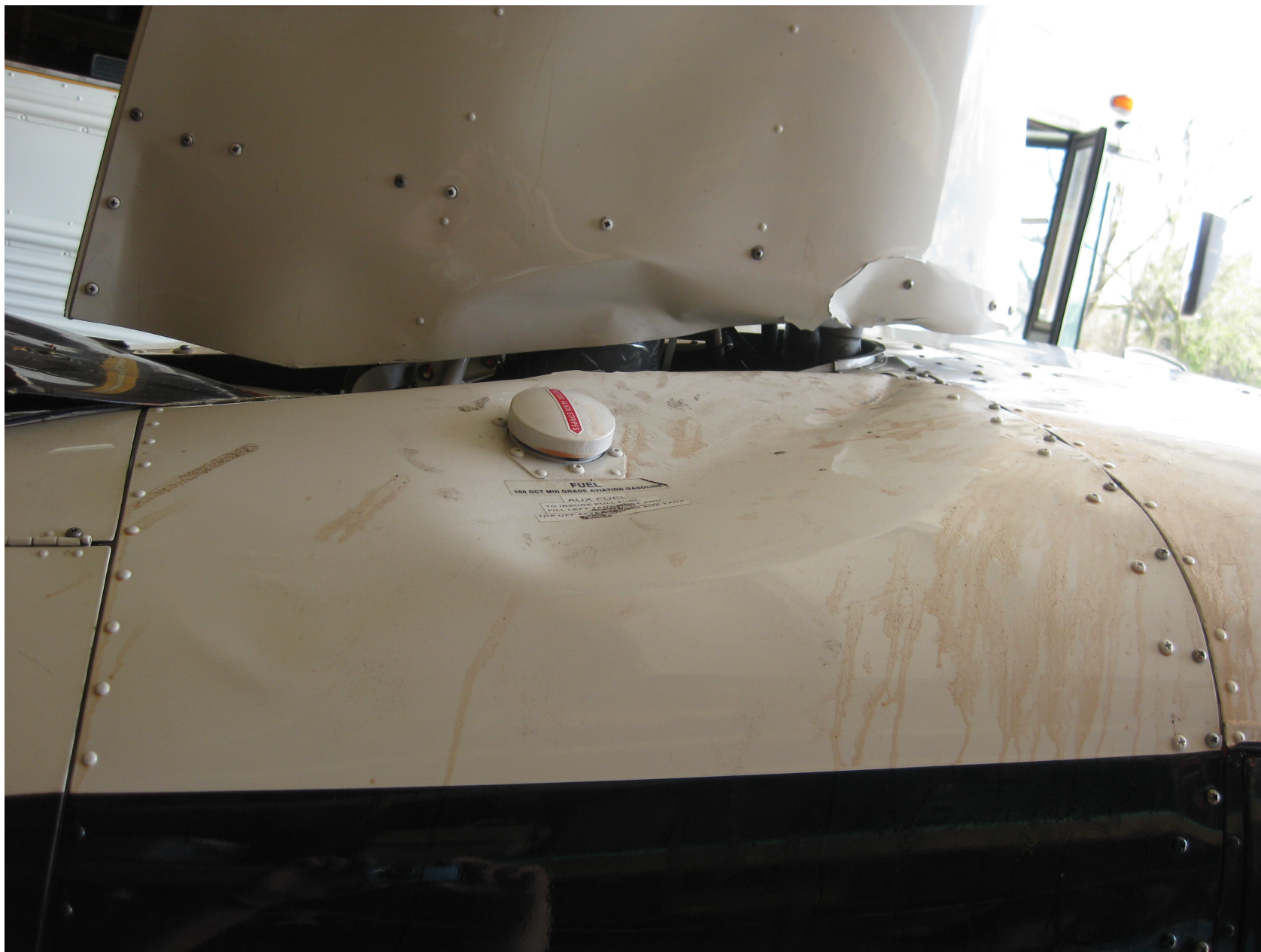
Photo 2 - Damage to Fuselage and Main Rotor Drive Shaft Under Housing (Courtesy of FAA)
