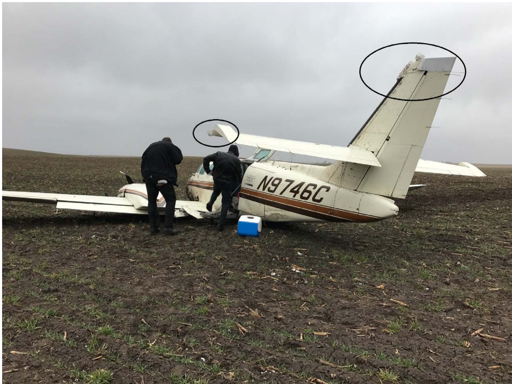
Photo 1 – Accident Site with Ice on Airframe
