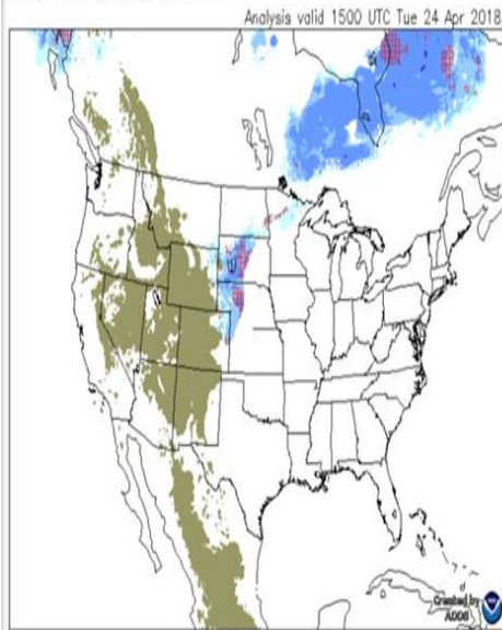
Icing severity at 5000 ft. MSL
