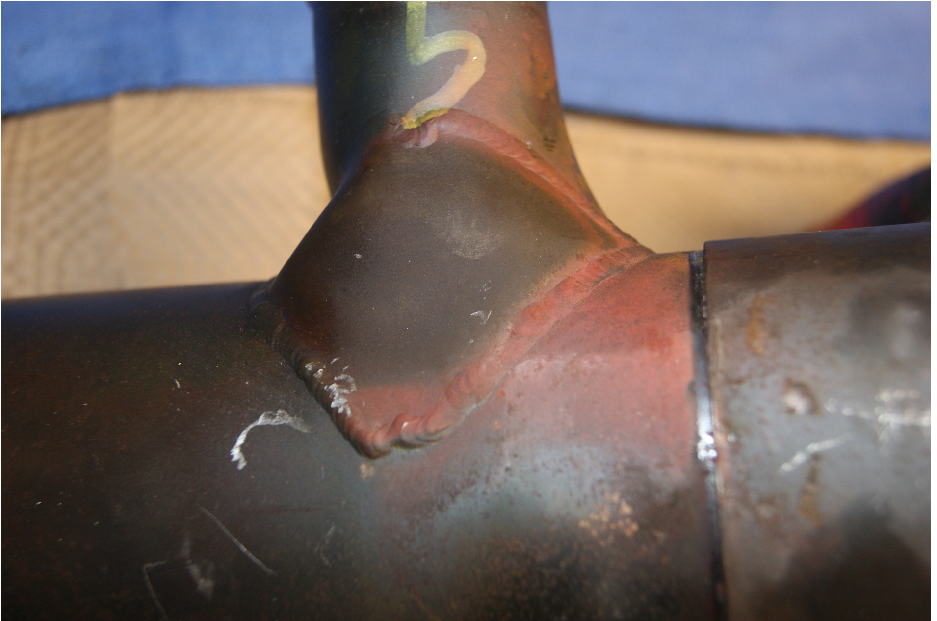
Photo 2 – Turbocharger manifold bore evidence of hot gas seepage.
