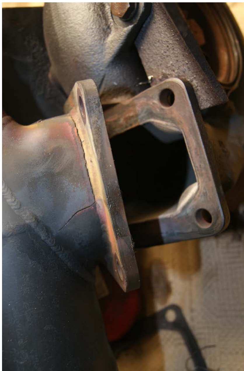
Photo 5 – Separated manifold flanges.
