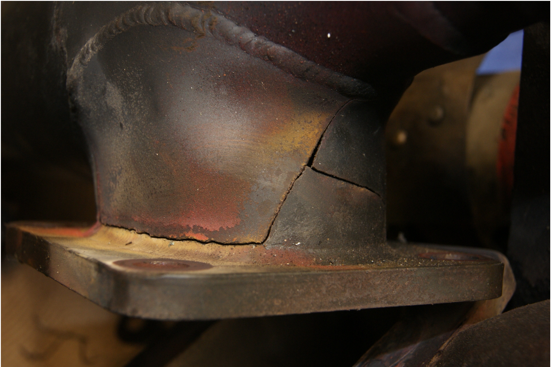
Photo 4 – Another view of the manifold crack.
