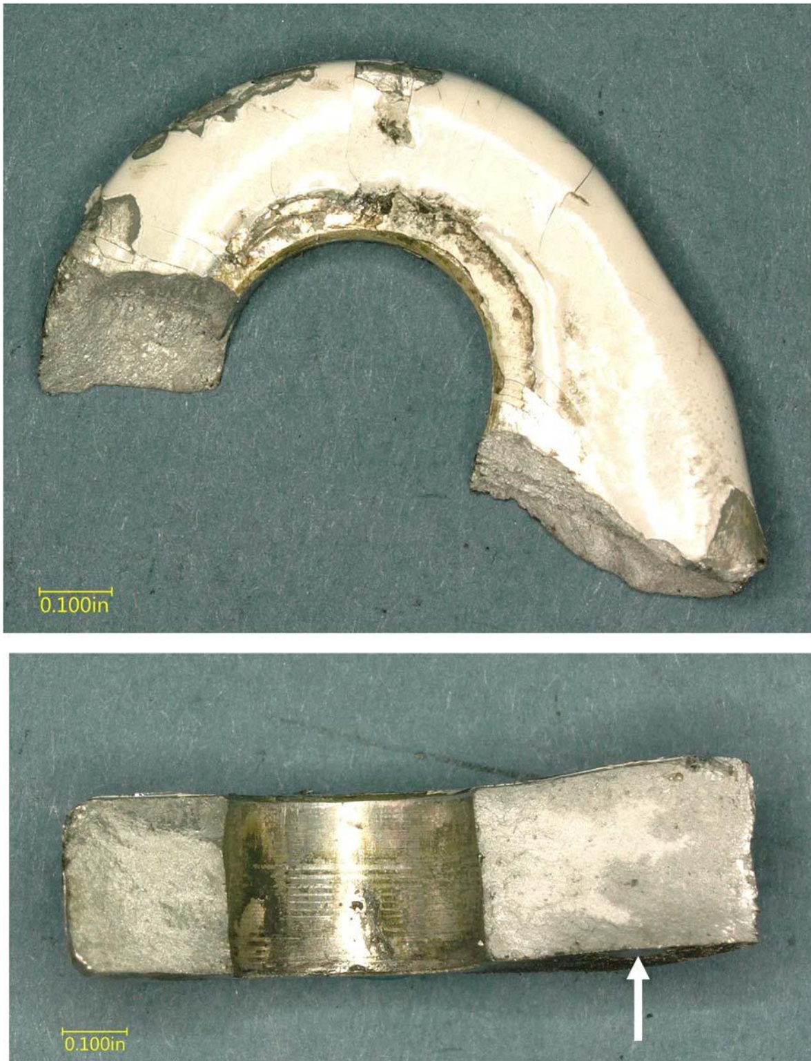
Figure 7: Digital microscope images of the flange piece. The white arrow indicates the out of plane deformation of one half of the piece.
