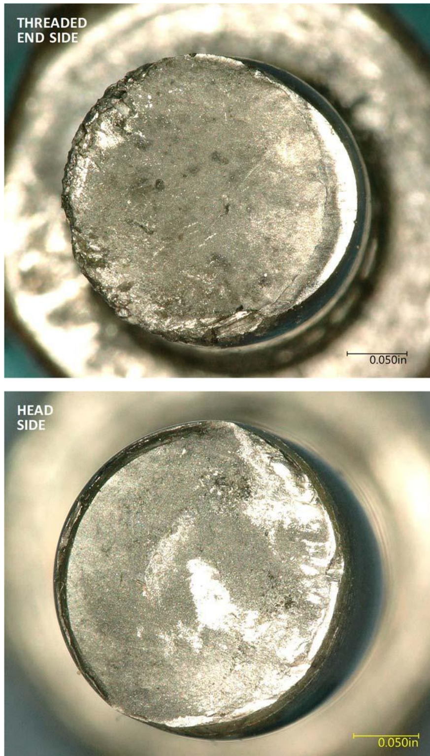
Figure 6: Digital microscope images of the fracture surfaces on the bellcrank assembly bolt pieces.
