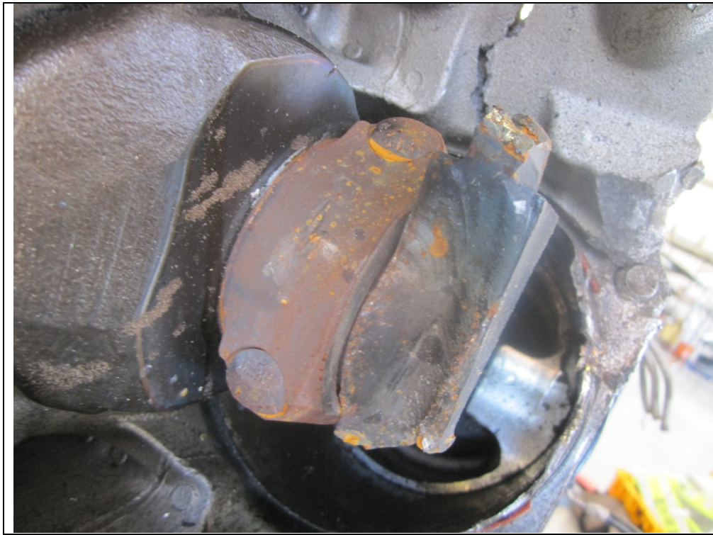
Close up view of crankshaft break. Rings are noted in the fracture surface
