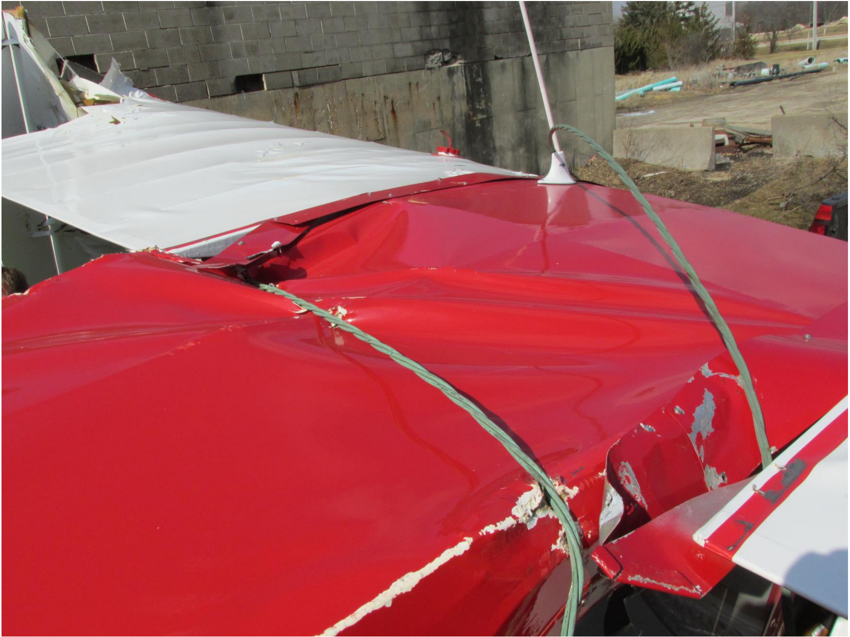
Photo 3 – Top of the Airplane and Power Line Wire
