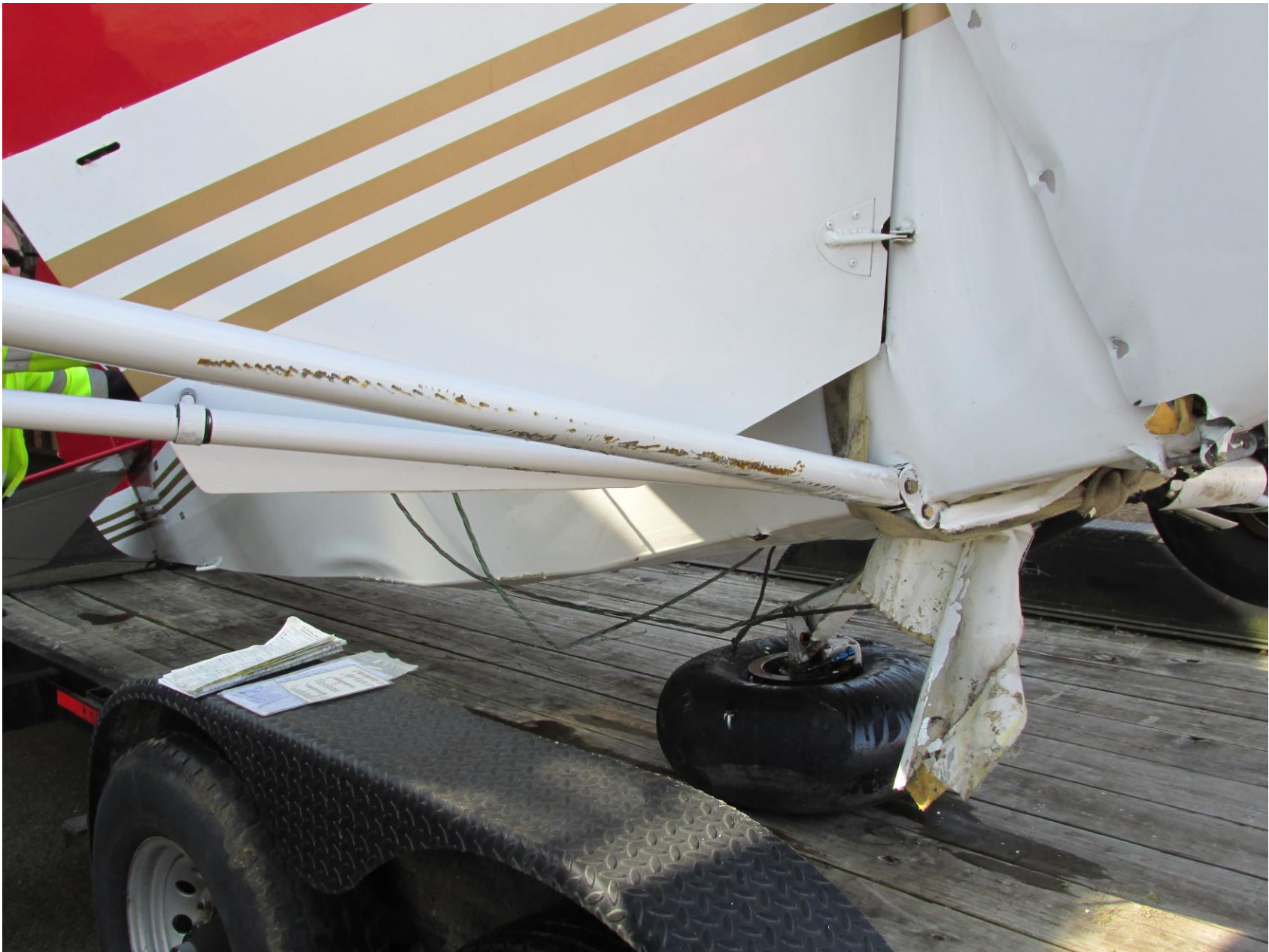
Photo 5 – Right Wing Strut with Wire Marks
