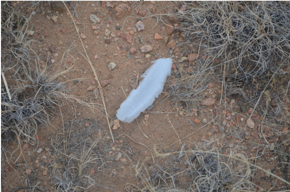
Figure 19 – Accident scene picture of an ice chunk that had fallen off the accident plane on the ground
