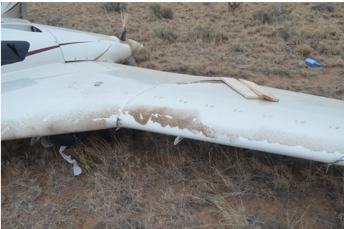
Figure 14 – Accident scene picture of ice accretion on the left wing
