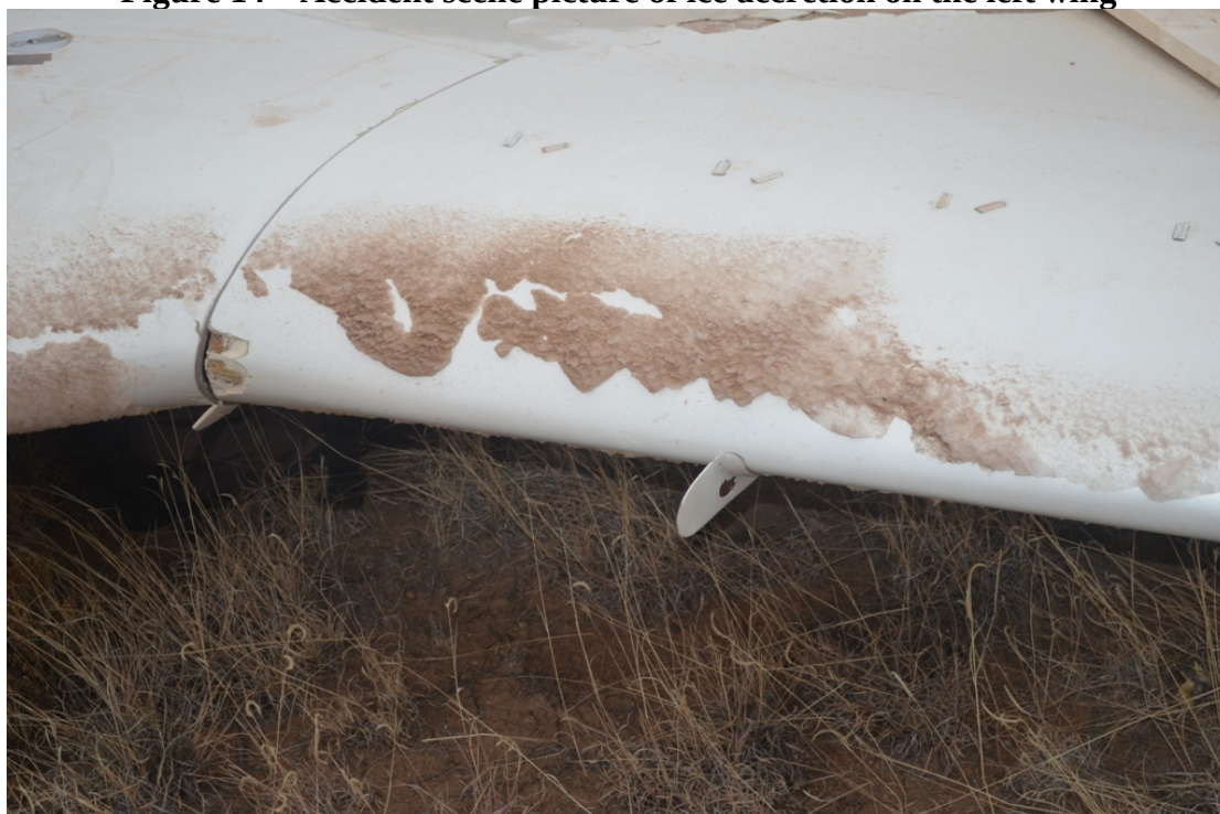
Figure 15 – Accident scene picture of ice accretion on the left wing
