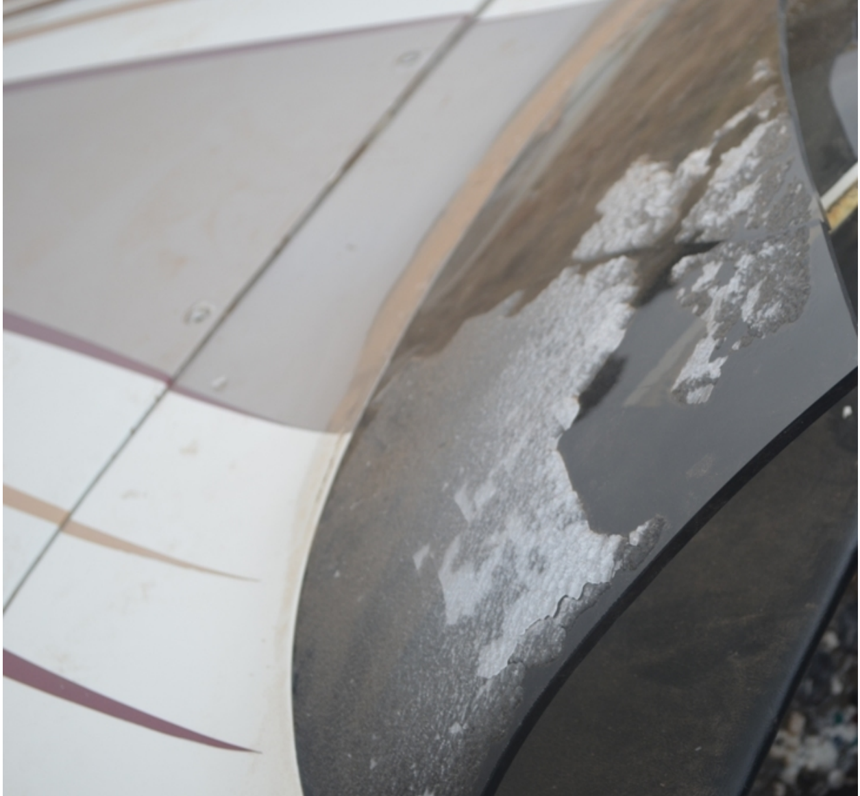
Figure 21 – Accident scene picture of ice accretion on the front windshield
