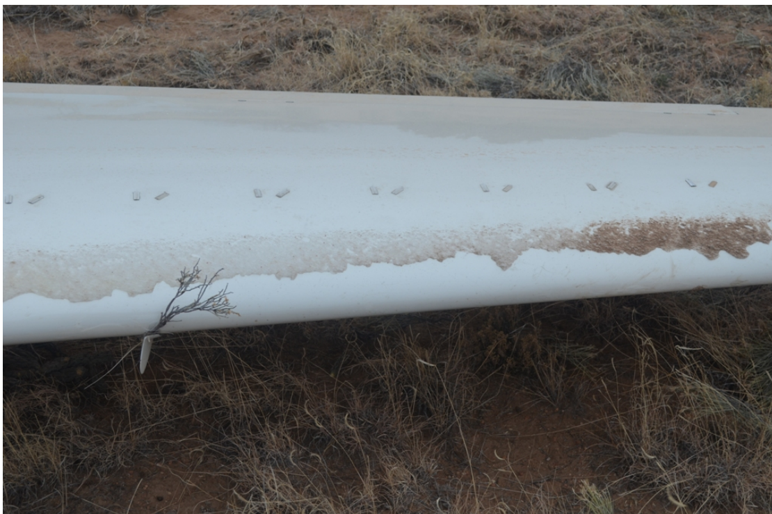
Figure 16 – Accident scene picture of ice accretion on the left wing
