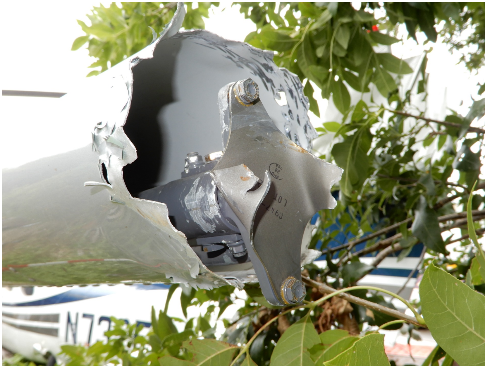
Photo 4 – Flex Plate Assembly and Tailboom
