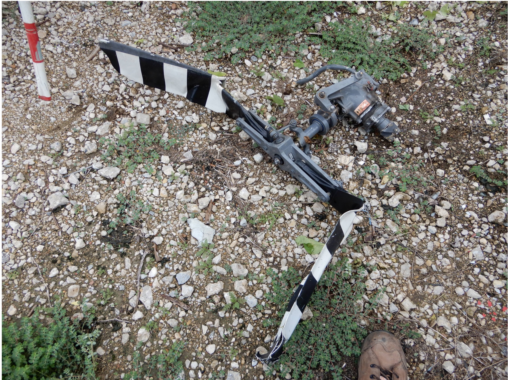
Photo 2 – Tail Rotor Assembly
