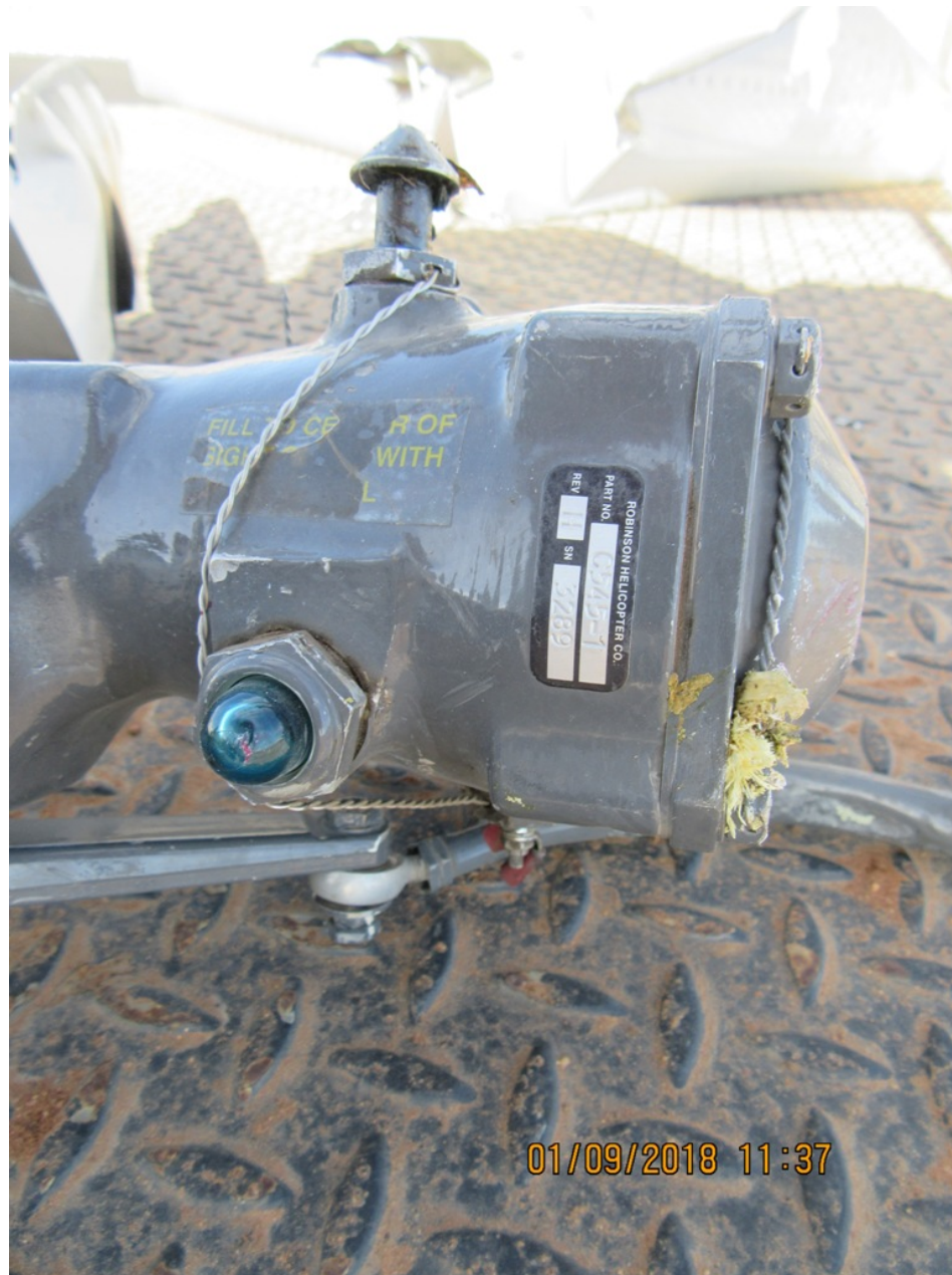
Photo 5 – Tail Rotor Gear Box (FAA Photo)
