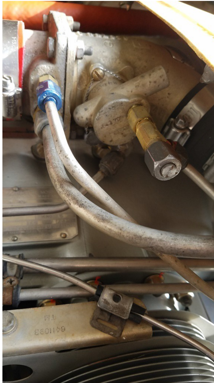
Photo 1 – View of Fuel System Test Port
