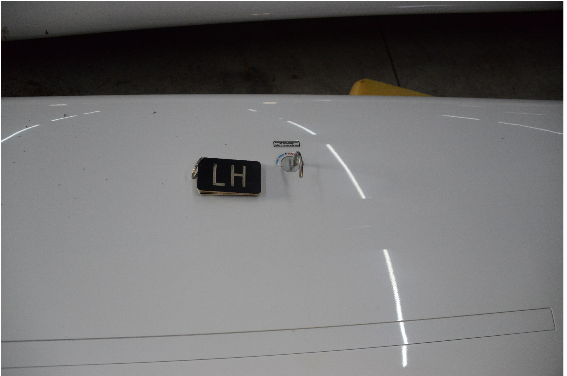
Photo 19 - View of the left fuel tank filler neck cap and vent.
