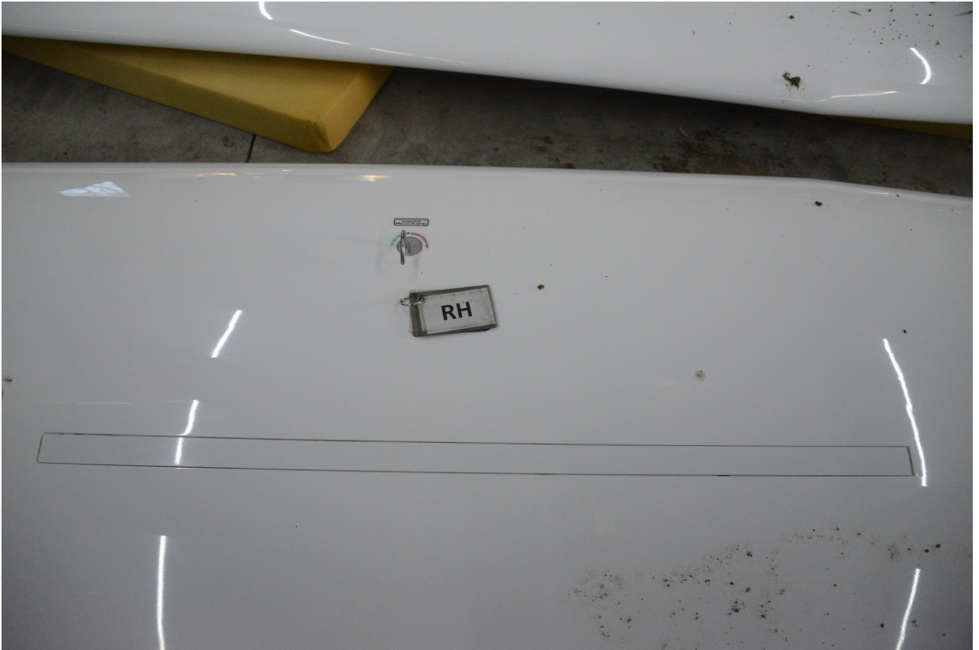
Photo 20 - View of the right fuel tank filler neck cap and vent.
