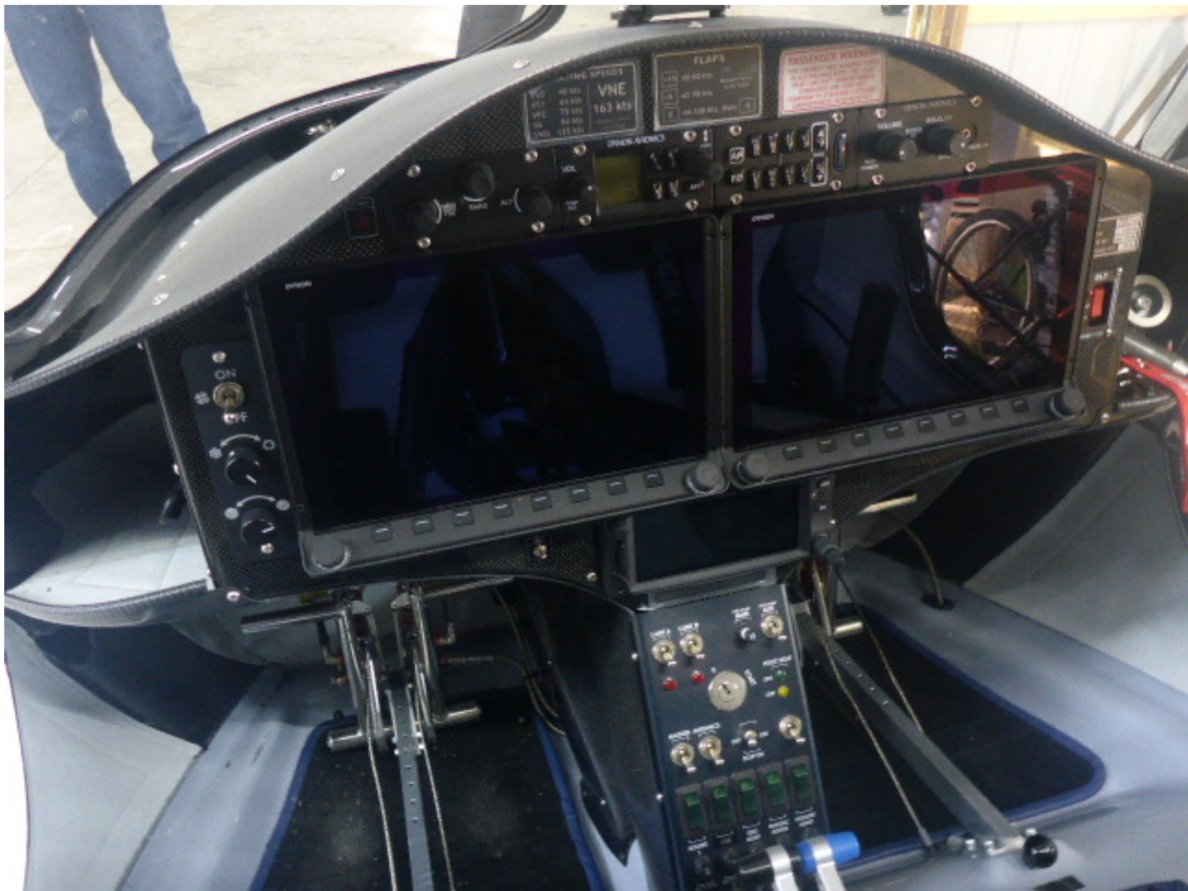
Photo 18 - View of the Dynon units before they were removed.
