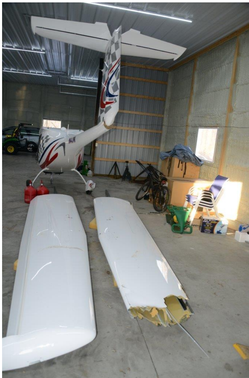
Photo 3 - View of the rear side of the recovered aircraft and detached wings.
