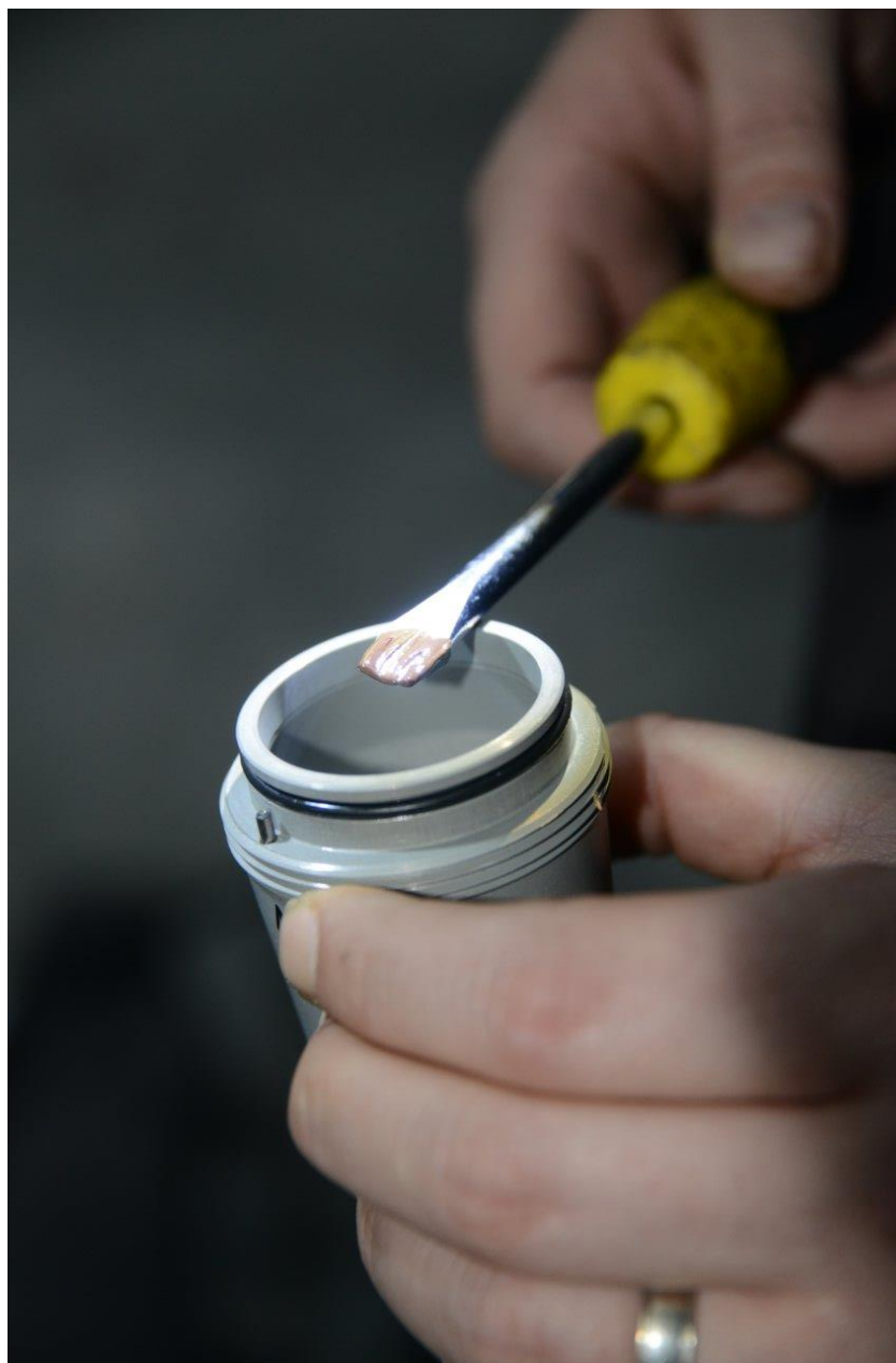
Photo 8 - View of the fuel filter bowl during testing of the liquid present for water. Testing paste exhibited no water present.
