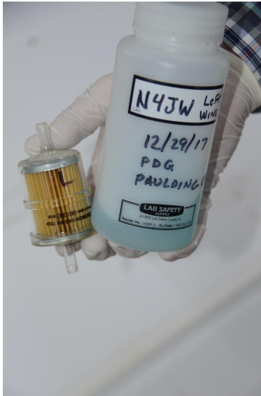
Photo 10 - View of the inline fuel filter and fuel tank sample from the left fuel system.
