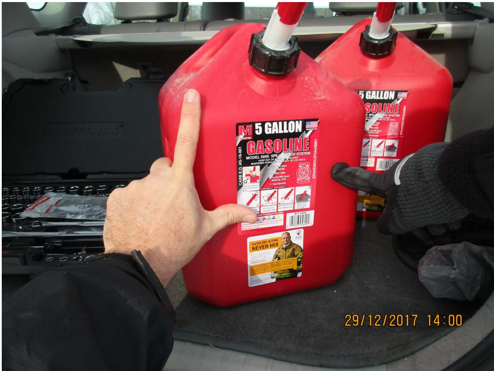
Photo 14 - View of a 5-gallon container of recovered fuel from the left tank. The recovered fuel filled about half of the container.
