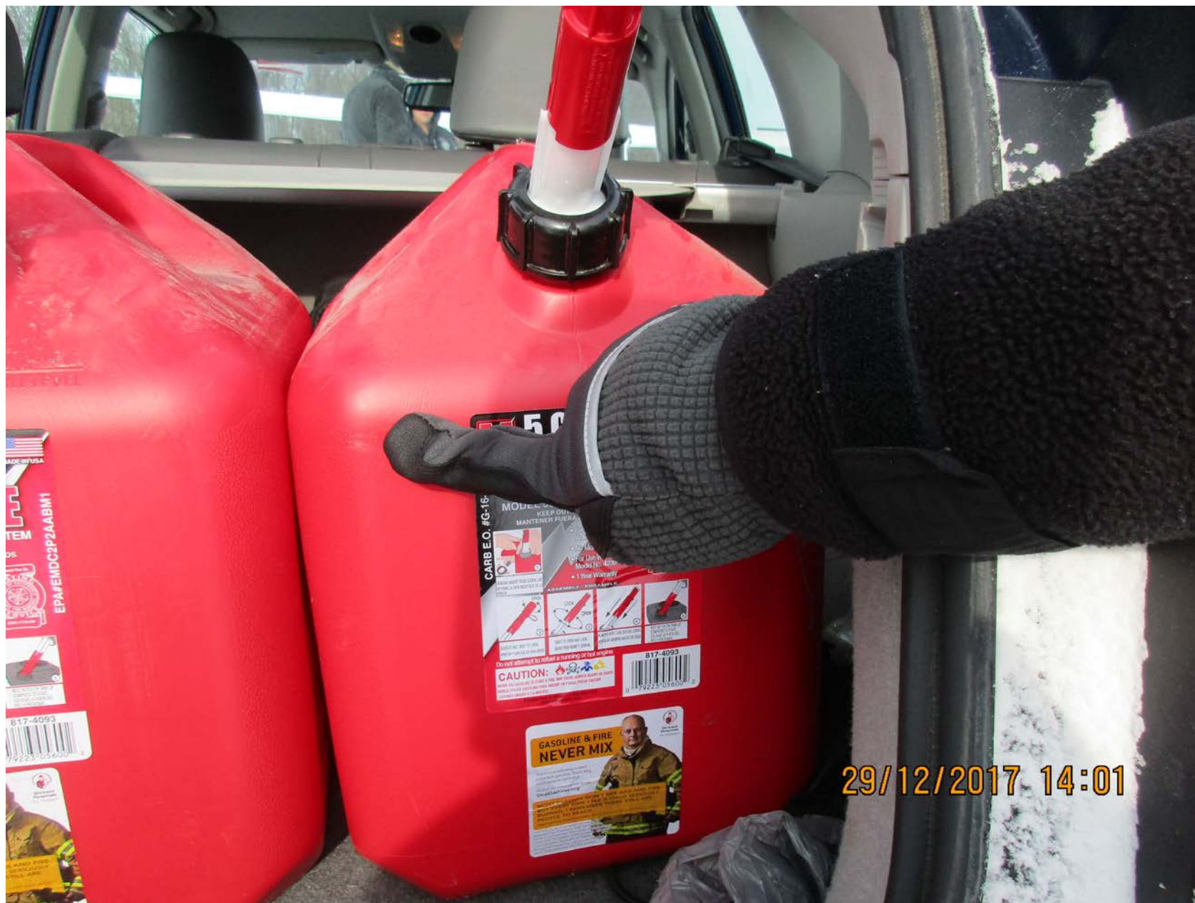
Photo 15 - View of a 5-gallon container of recovered fuel from the right tank. The recovered fuel filled about three quarters of the container.
