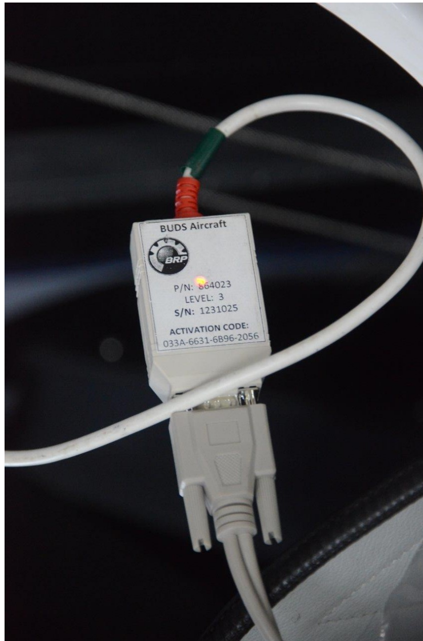
Photo 6 - View of an electrical connector during the ECU download.
