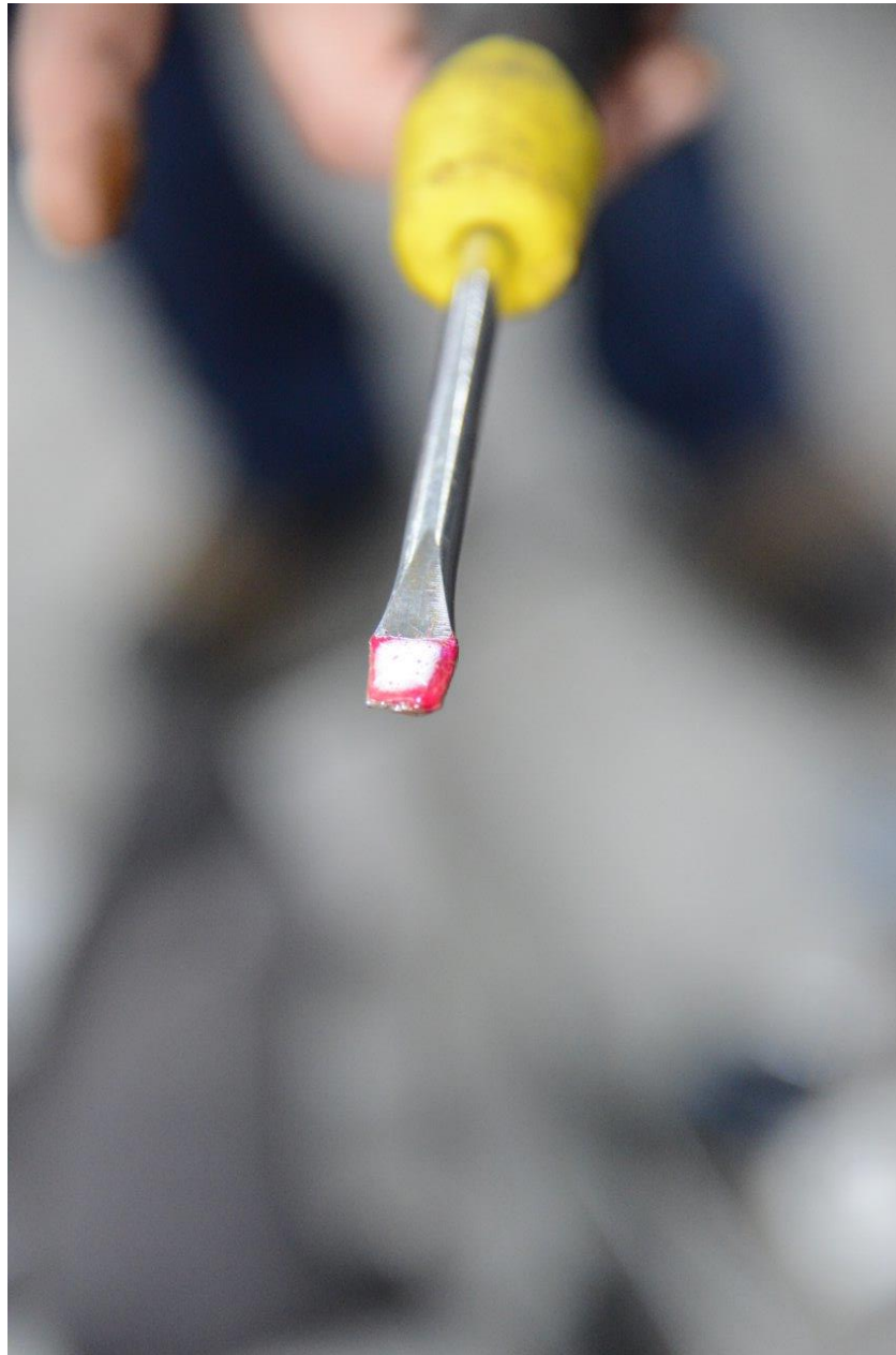
Photo 9 - View of the testing paste with water applied subsequent to fuel filter bowl liquid testing.
