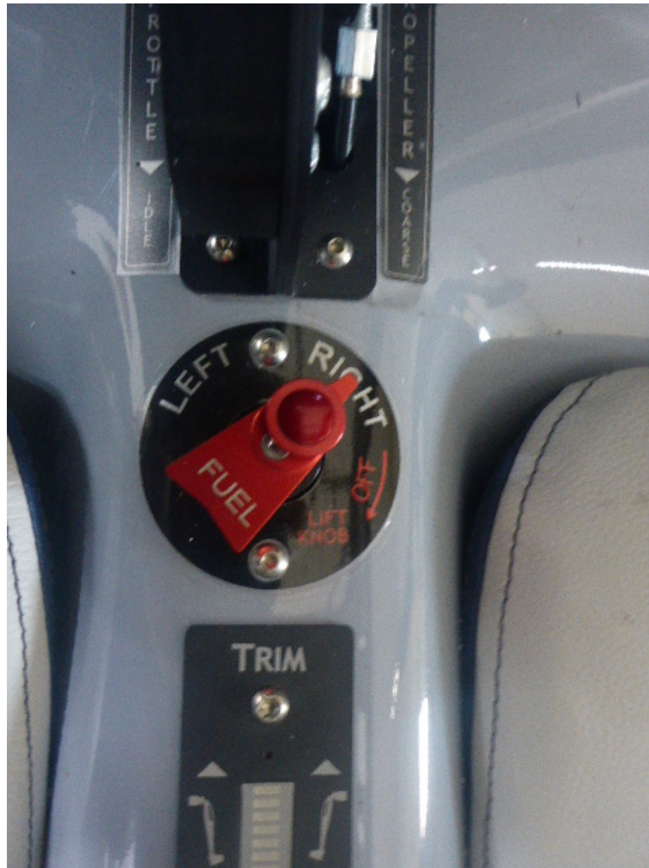
Photo 17 - View of the fuel selector showing the right tank is selected.
