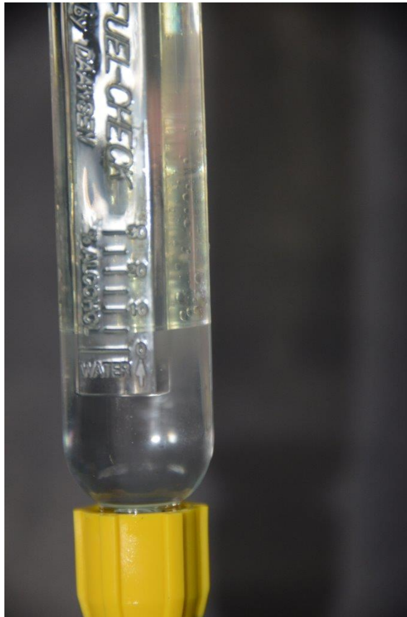
Photo 5 - View of the alcohol tester exhibiting a reading about 5%.
