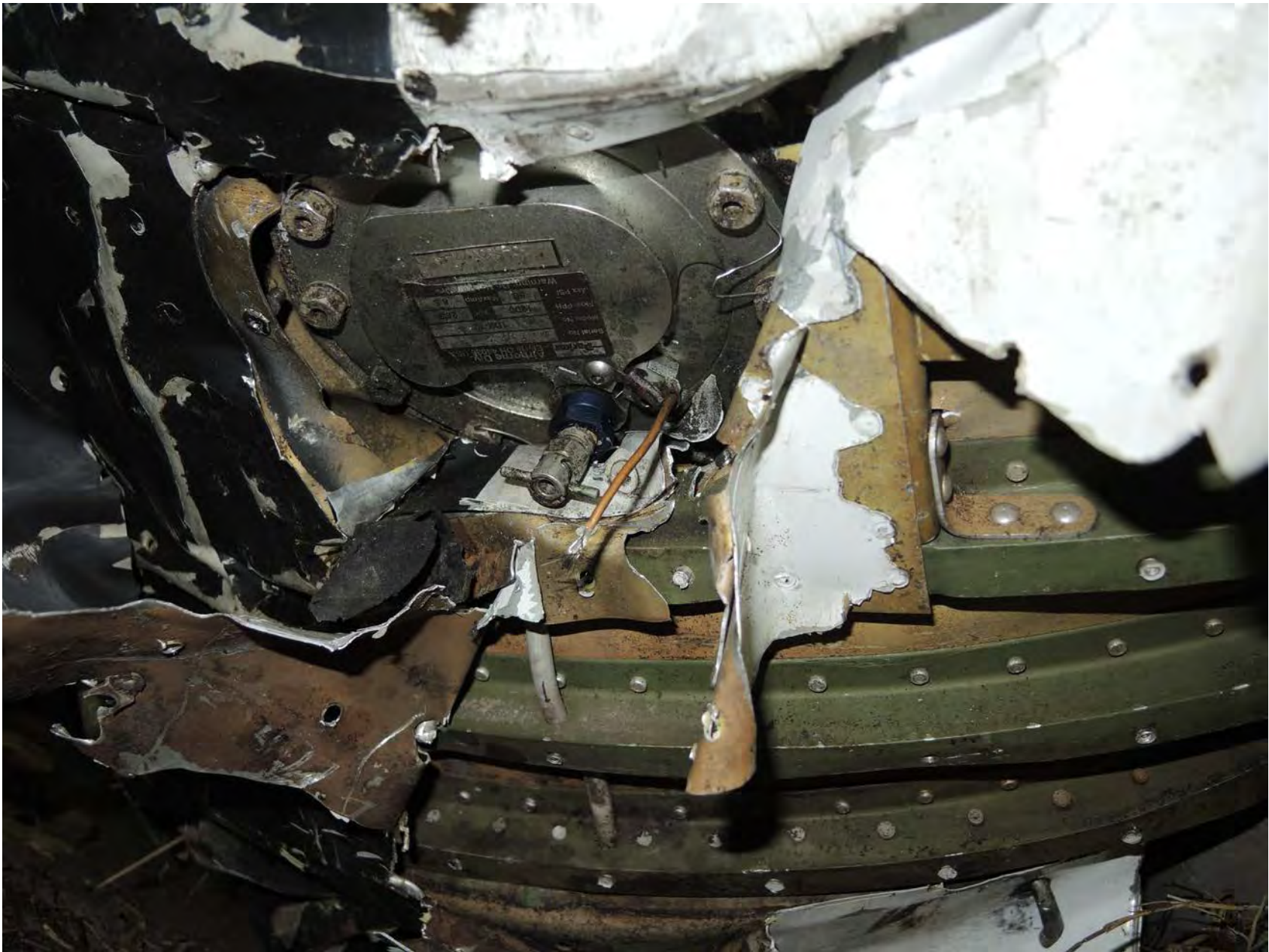
Photo 19 - View of the left nacelle fuel tank's pump with a separated electric wire.
