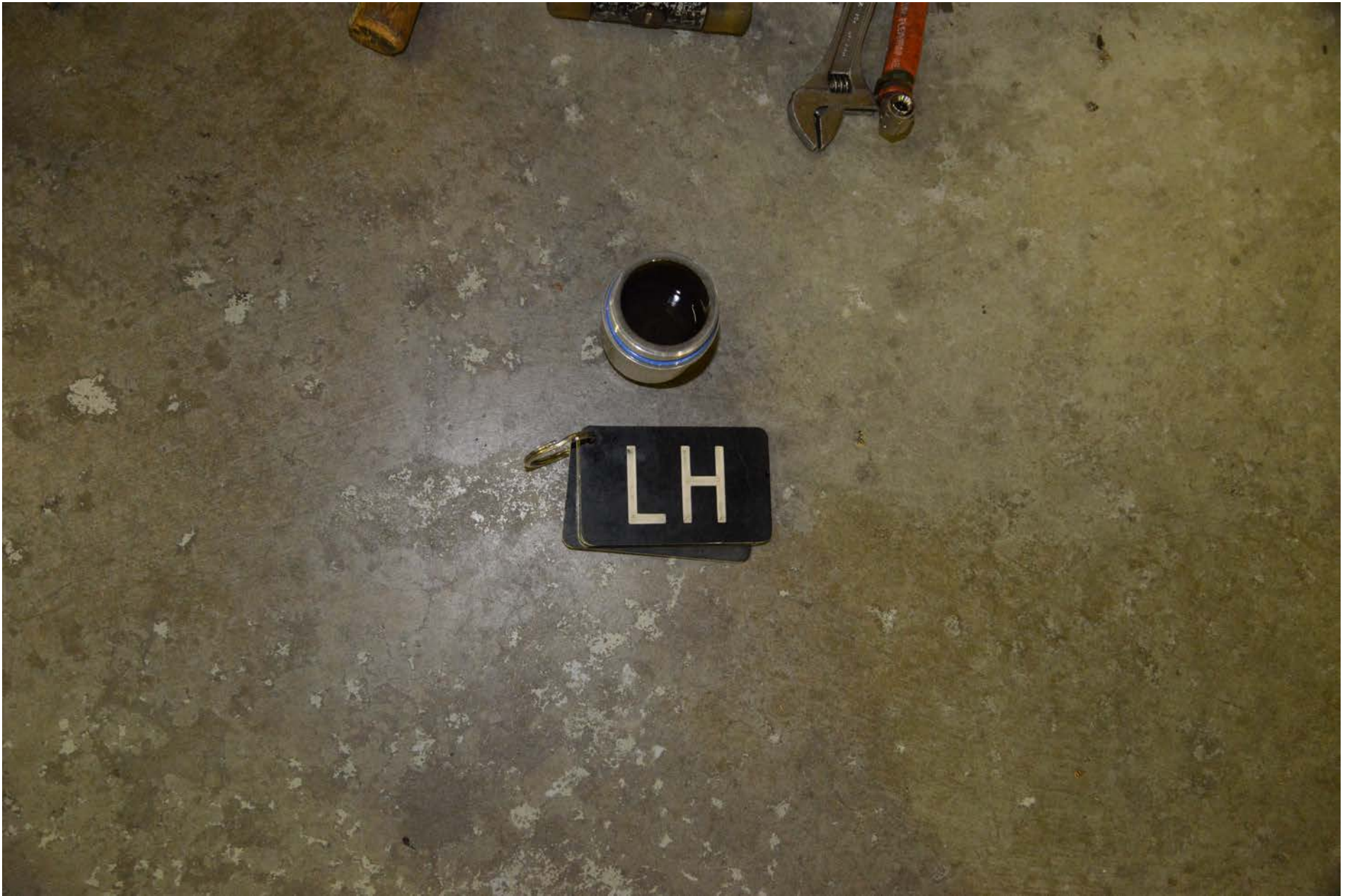
Photo 10 - View of the opened left fuel filter bowl containing a liquid.
