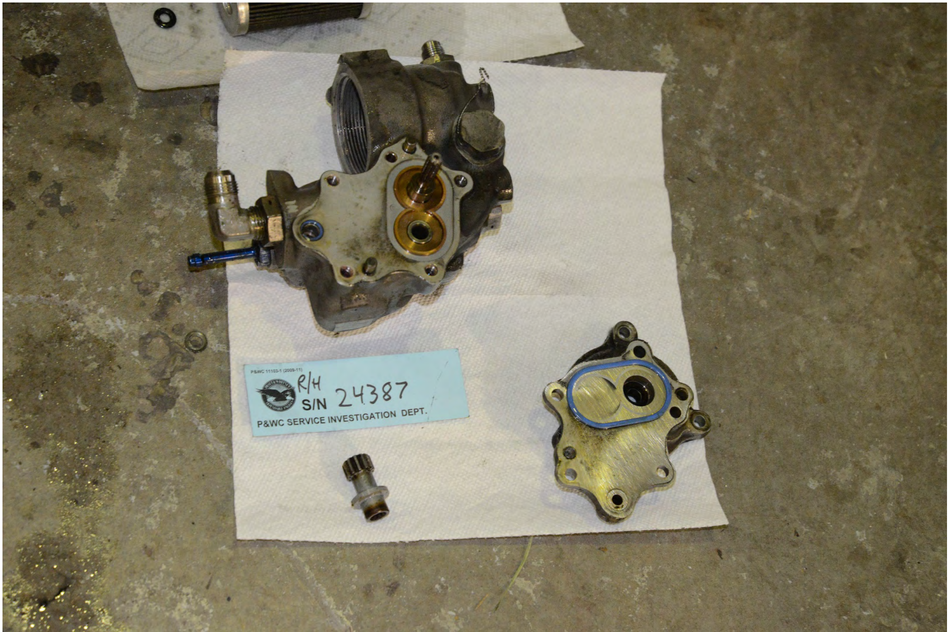
Photo 11 - View of the disassembled right engine driven fuel pump.
