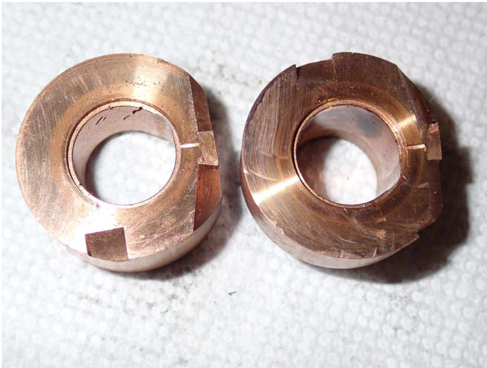
Photo 20 - Close-up view of bearings from an engine driven fuel pump.
