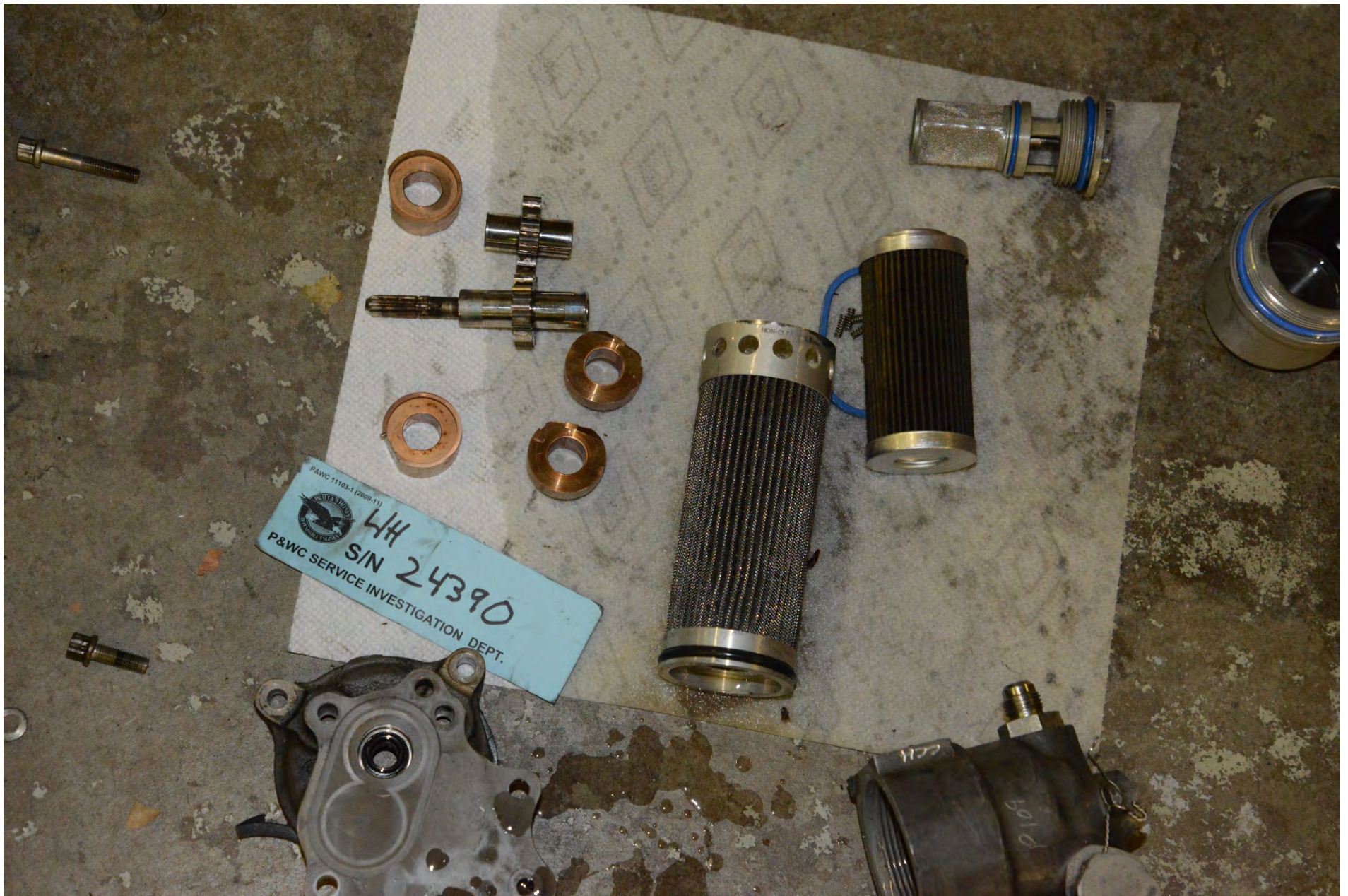
Photo 13 - View of the disassembled left engine driven fuel pump.
