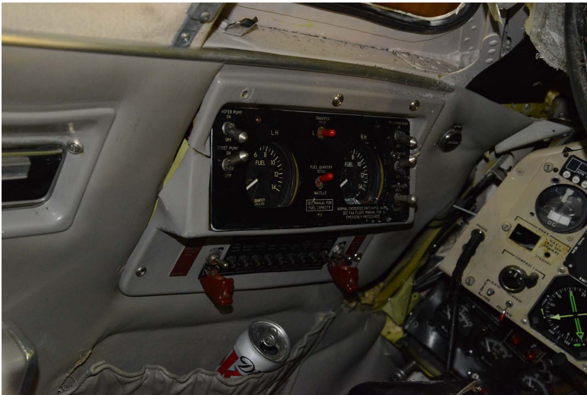
Photo 6 - View of the fuel control panel.
