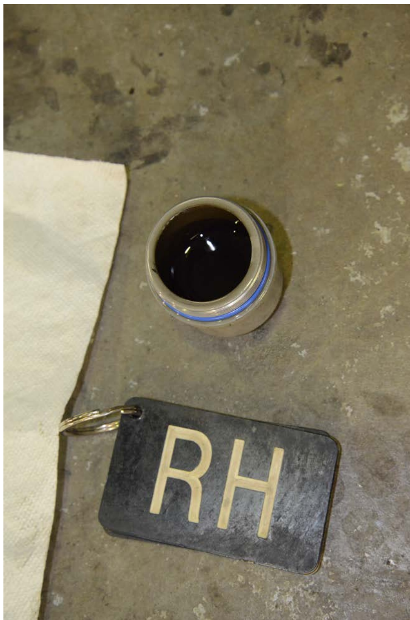
Photo 12 - View of the opened right fuel filter bowl containing a liquid.
